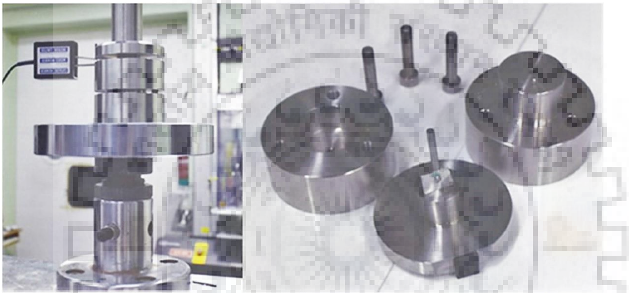
Figure 4.7: External view of machine used for Small Punch Test (left) and die and pin used for holding the sample and pushing the steel ball (right)
