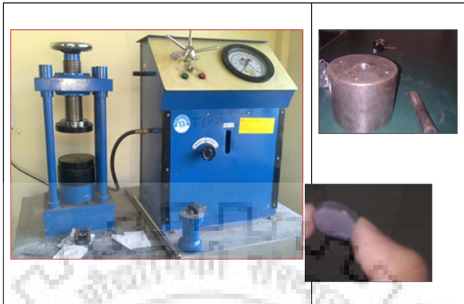
Figure 3-3: Hydraulic machine, die steel die-punch, compacted pellet
