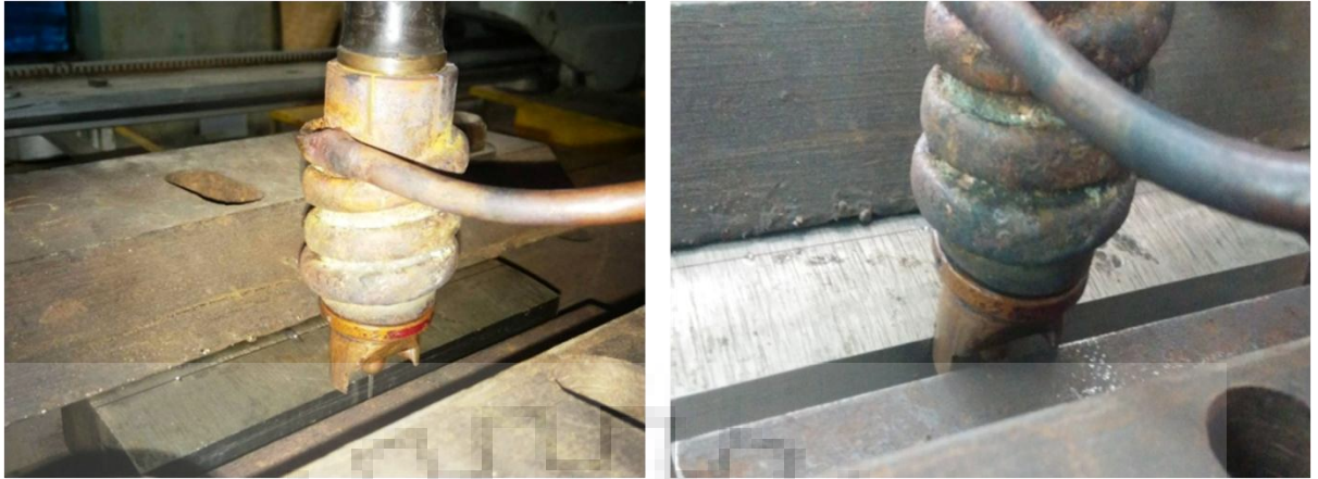
Figure 3-8 Photograph showing closely fitted narrow groove of 25 mm thick dissimilar plates with narrow welding torch nozzle inserted in it.
