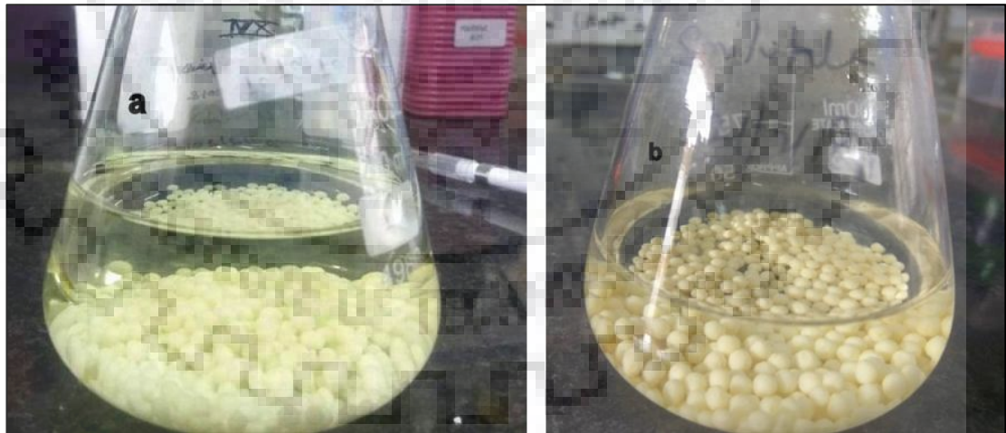
Fig. 5.20 (a) Chitosan immobilized beads before growth in the undetoxified hydrolysate (yellowish in color) (b) chitosan immobilized cells after 20 h of growth in the detoxified hydrolysate (clear solution). Yellowish color of simulated hydrolysate was due presence of HMF and furfural.
