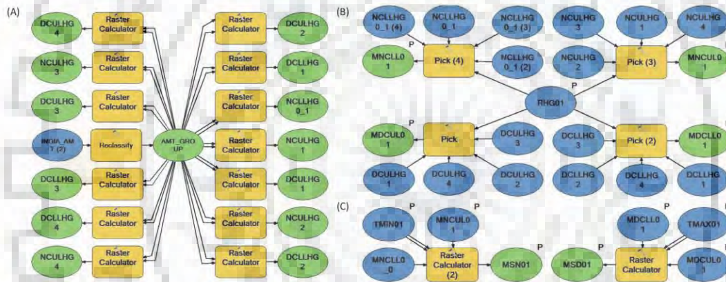
Fig. 10. Model builder tools for data diagnosis (A) Tool for adaptive comfort limits (B) PT for monthly comfort limit (C) PT for monthly stress.
