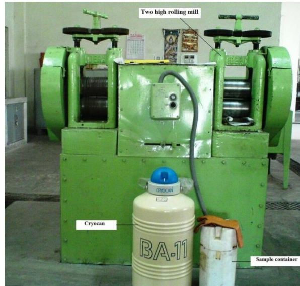
Figure 3.1 Experimental Set Up of Cryorolling
