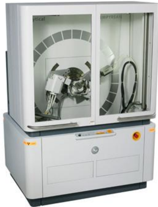
Figure 3.8 Image Showing Pan Analytical MRD System Used to Measure Texture
