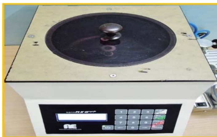
Figure 2.6: Spin coater model, Spin NXG P-1
