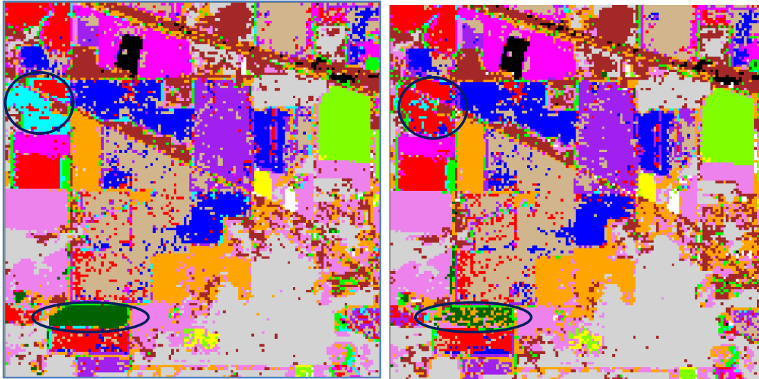
Figure 5.5 (a) SVM classified pseudo image got from Daub2_1 feature extraction of AVIRIS dataset of Indiana Pine, (b) SVM classified pseudo image got from Haar_2 feature extraction of AVIRIS dataset of Indiana Pine.
