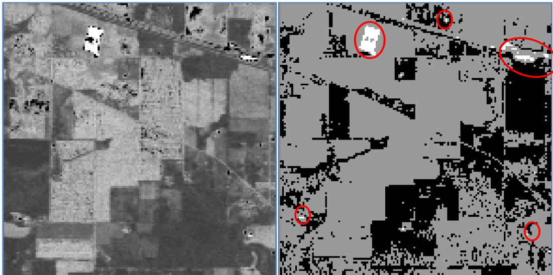
Figure 5.9: The extraction of class stone-steel towers by ICAMM two different iterations applied on Haar_1 feature extraction.
