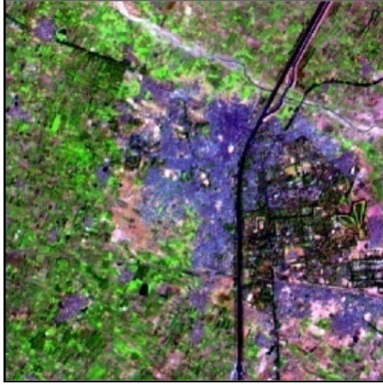
Figure 3.5: The FCC of Roorkee and its surrounding area by Hyperion sensor (Red: Band 70, Green: Band 20, Blue: Band 2).
