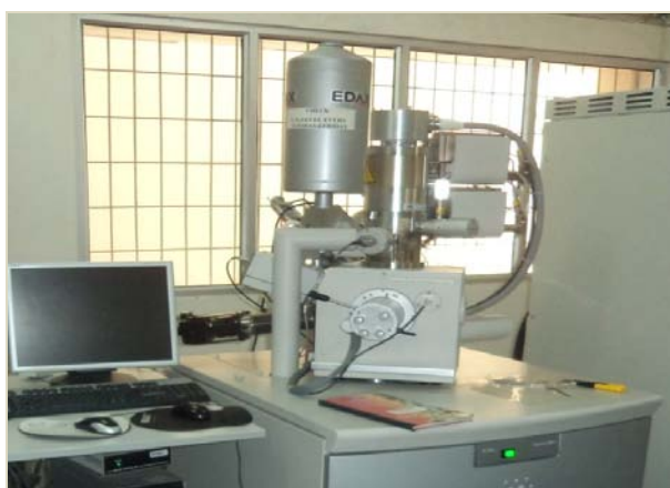
Fig. 3.2: A photograph of FEI Quanta 200F scanning electron microscope used in the present study.
