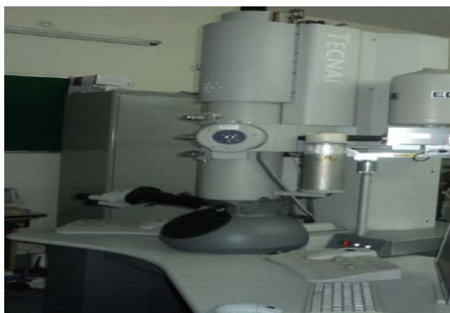
Fig. 3.3: A photograph of TECNAI G2 transmission electron microscope used in the present study.
