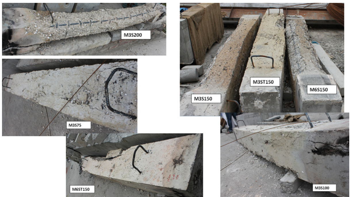
Fig. 4.17: RC columns after the fire exposure
