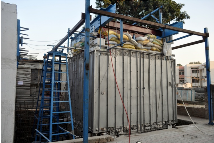
Fig.2.33: The test frame before the fire test with fire enclosure
