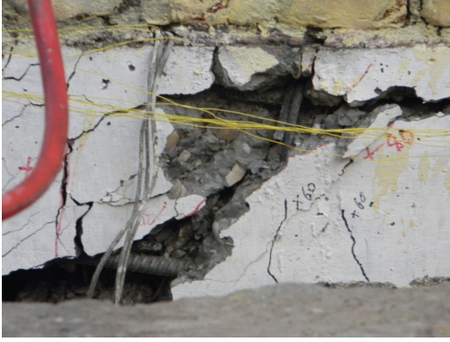
Fig.3.5: Shear failure in beam B1 with buckled reinforcement
