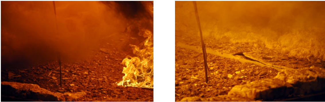
Fig.2.39: Spalled concrete from the elements of the frame during fire
