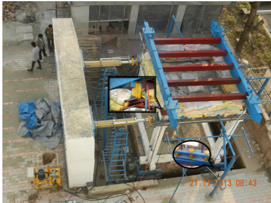
Fig.2.12: Test Arrangement for the seismic loading as seen from the top
