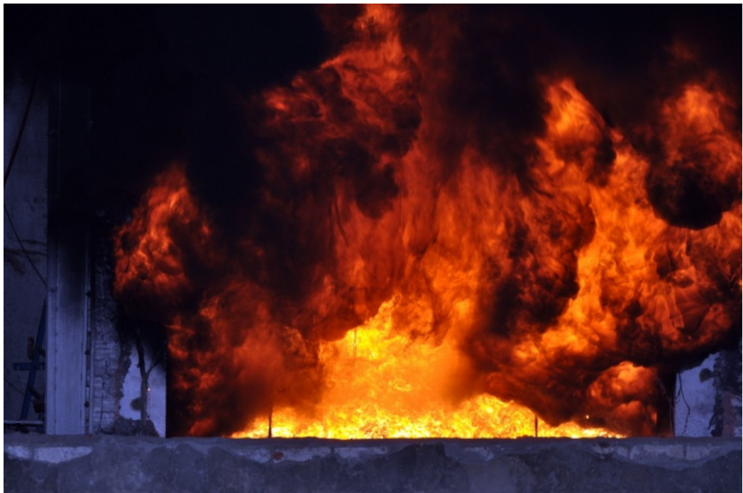
Fig.2.36: Attainment of flashover
