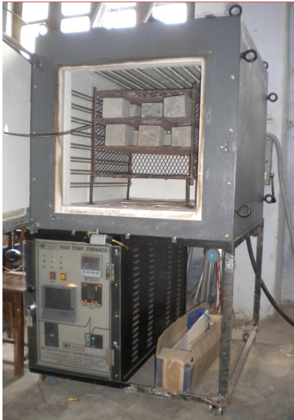
Fig. 3.4 Inside view of high temperature muffle furnace
