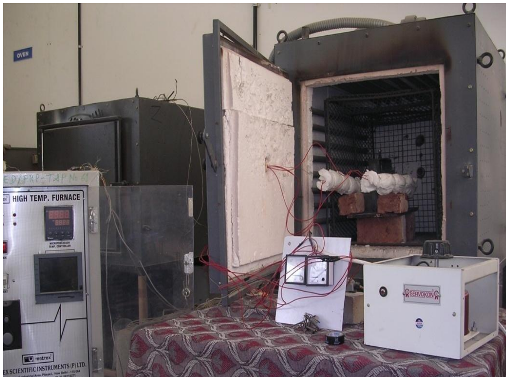
Fig. 5.4 Complete testing setup of non-steady state hot-wire method (parallel) apparatus with furnace.
