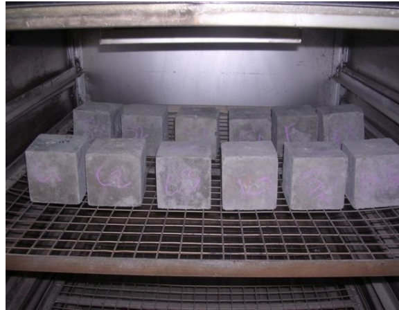
Fig. 4.4 A view of cubic specimens in an oven for measurement of moisture
