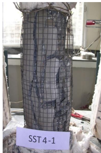
Fig. 4.12 Spalling in the specimen (SST4-1) exposed to 400 °C
