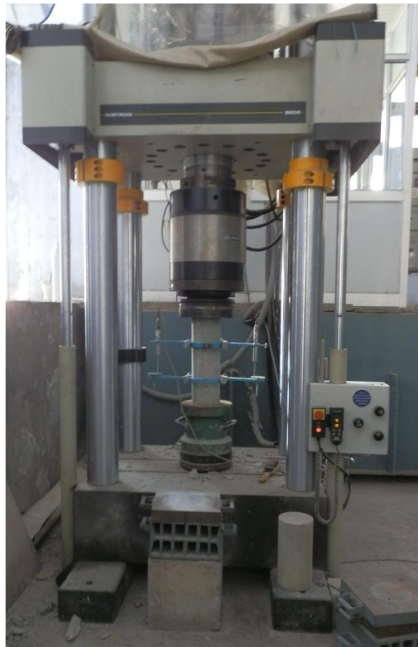
Fig. 4.7 Test setup for uni-axial compression
