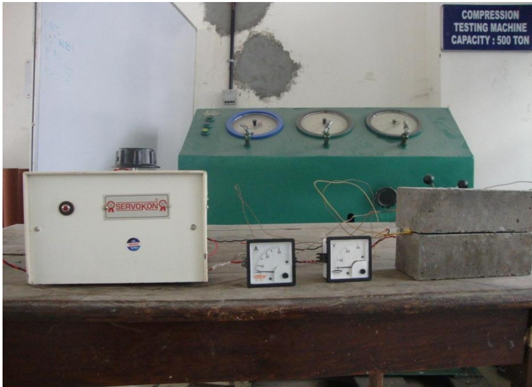
Fig. 5.3 Test setup of thermal conductivity measurement apparatus with hot-wire method (parallel).
