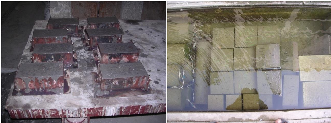
Fig 5.2 Stages of casting and curing of test specimens
