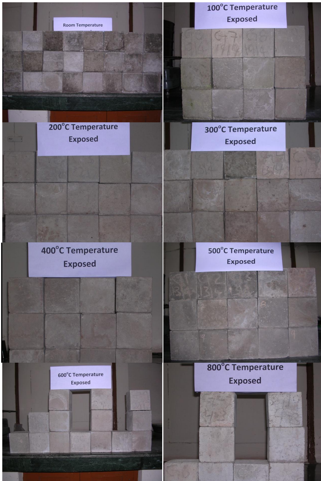
Fig. 3.14 Test specimens of GGBFS HPC subjected to different elevated temperatures
