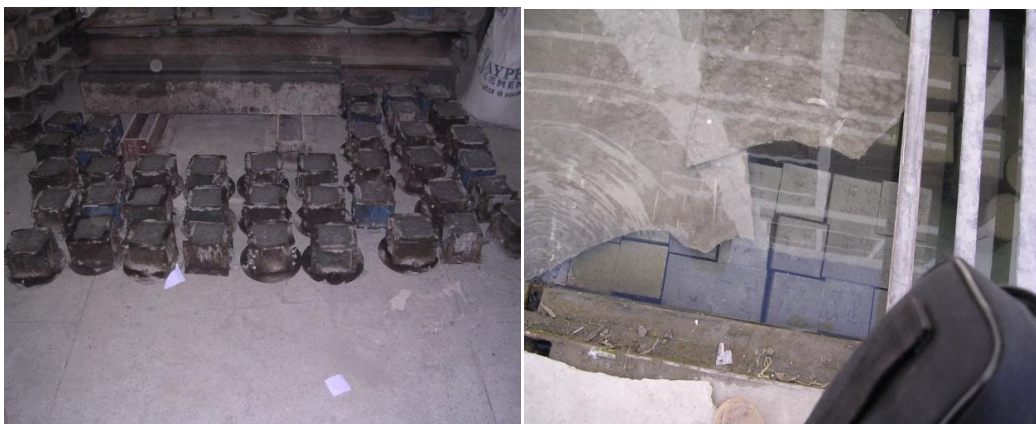
Fig. 3.2 Casting and curing of cube test specimens
