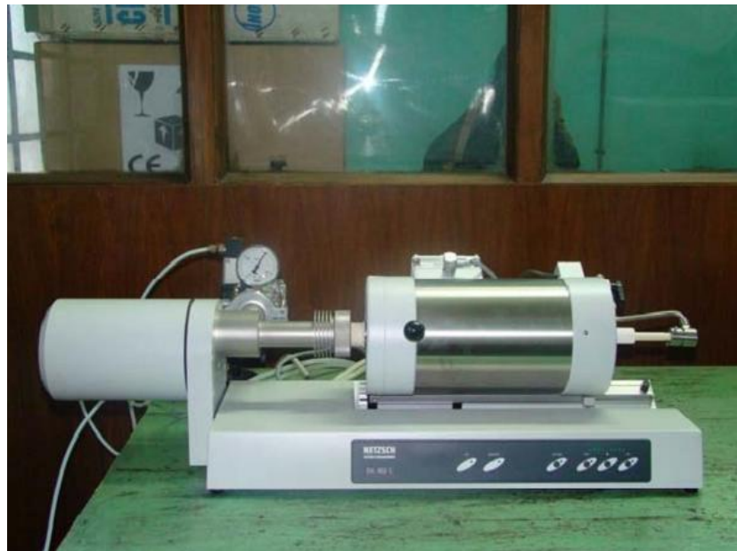
Fig. 5.5 A view of thermo dilatometric apparatus for thermal expansion test (CGCRI)
