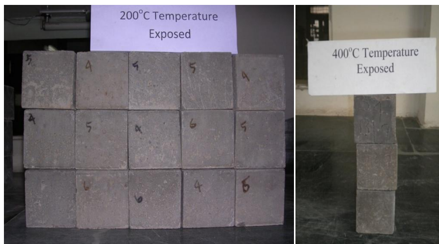
Fig. 3.19 Test specimens of silica fume HPC subjected to different elevated temperatures
