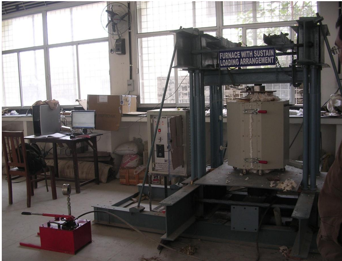
Fig. 4.5 A view of loading frame with vertical split type muffle furnace
