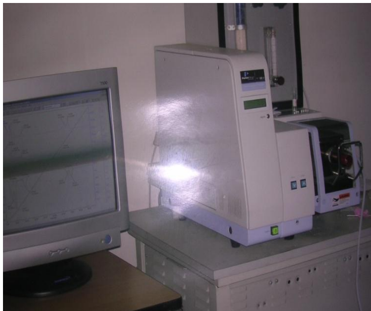
Fig 5.7 Thermogravimetric instrument for measuring mass loss of HPC concrete
