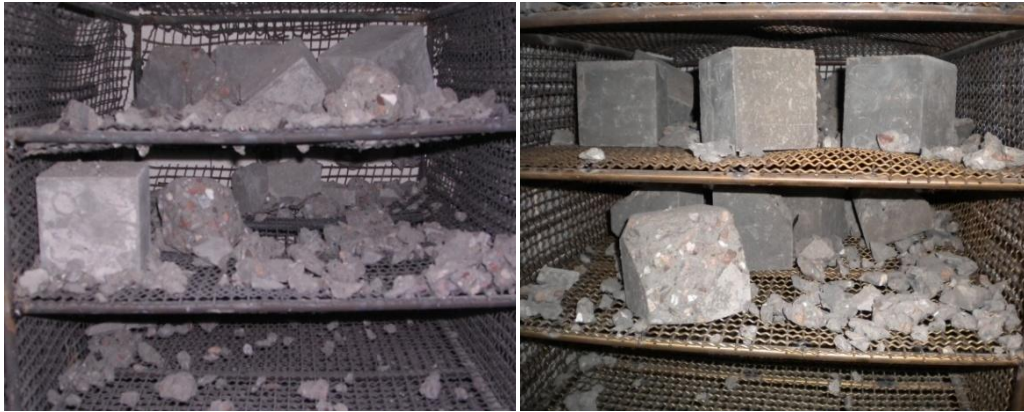
Fig. 3.20 Spalling of test specimens during thermal loading
