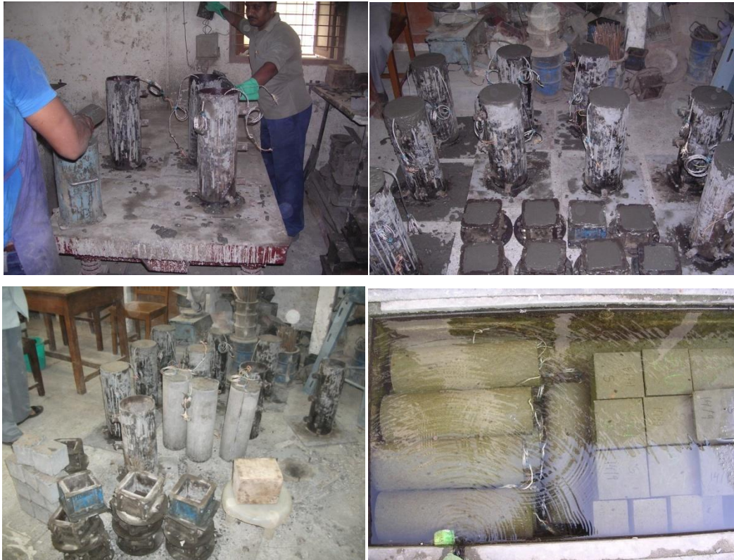
Fig. 4.3 Stages of casting, de-moulding and curing of HPC specimens
