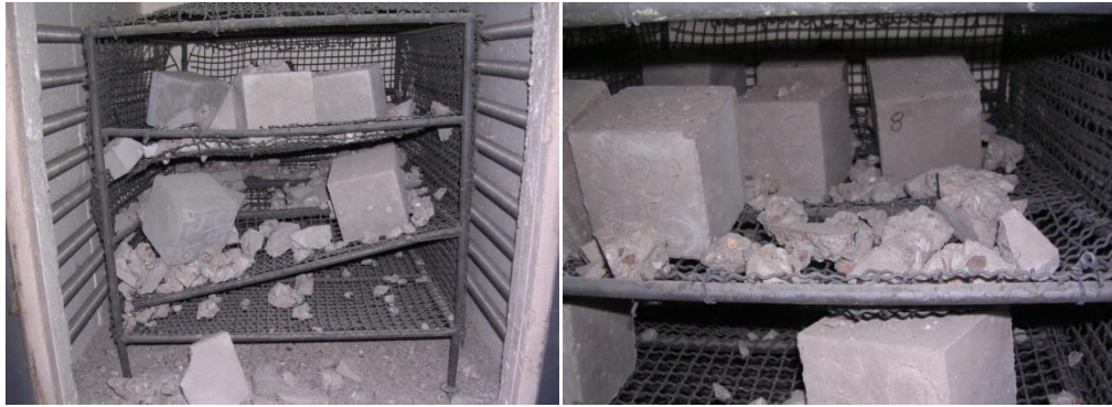
Fig. 3.16 Bursting test specimens subjected to thermal loading at 600 °C and 800 °C
