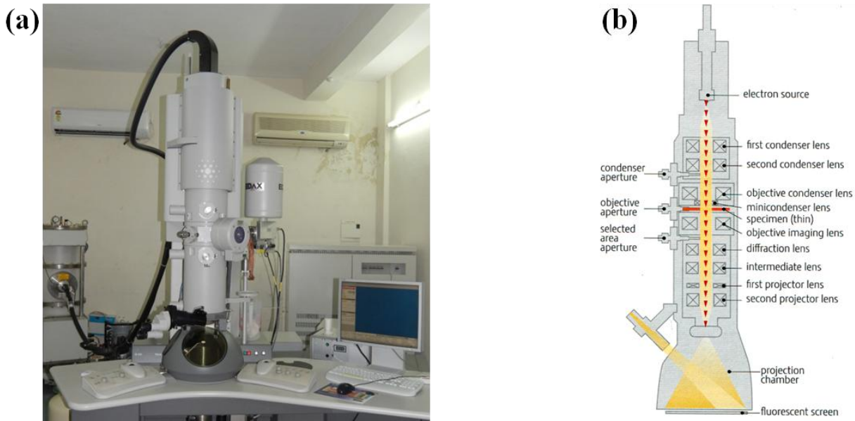
Figure 3.9: (a) Photograph of the TEM unit (FEI Tecnai-20), (b) Schematic diagram of TEM ( micron.ucr.edu/public/manuals/Tem-intro ).
