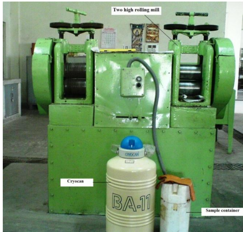
Figure 3.1: Experimental set up of cryorolling.
