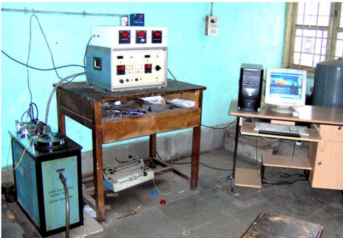
Fig. 3.13 Wear and friction (pin-on disc) machine used for conducting wear experiments.
