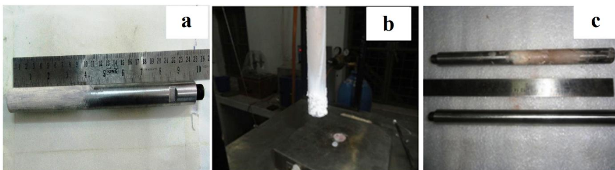
Fig.3.3 Zirconia coated ultrasonic probe. (a) before processing, (b) during processing, and (c) after processing and cleaning.
