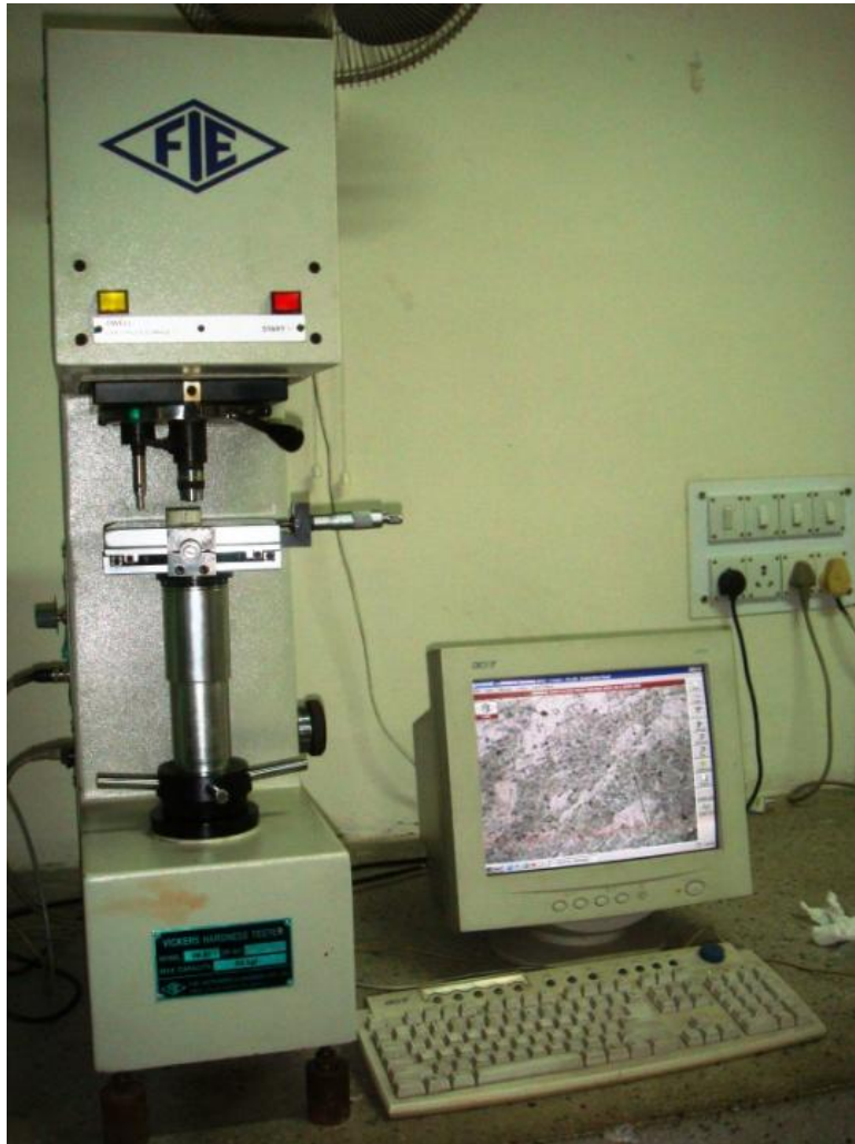
Fig. 3.8 Vickers hardness tester set up used for the measuring hardness.
