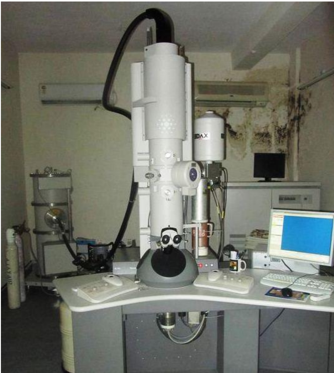
Fig. 3.6 200 kV TEM is used for the analysis of carbon black nano powder.
