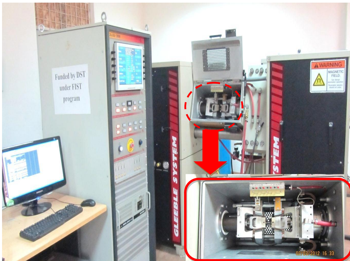
Fig. 3.11 Gleeble®3800 machine used for compression testing experiments.
