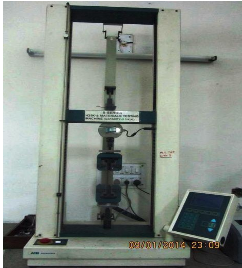
Fig. 3.10 H25 K-S Tinius Olsen tensile testing machine used for the tensile testing.
