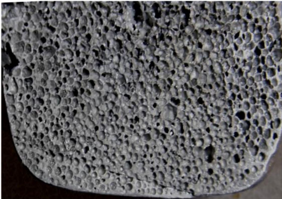
Fig. 5.3 Photograph of cast foam showing cross section of Al-Sc foam produced by melt route using TiH_2 as a blowing agent shown at approximately real size, which exhibits several features resulting from Sc addition, such as uniform pore distribution and no drainage collection at the bottom.
