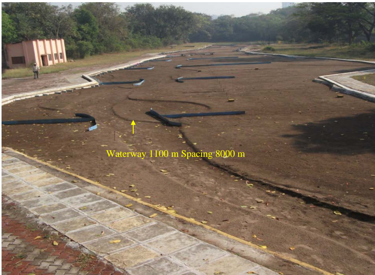
Figure 7.30 Channel configuration and position of T-shape groynes
