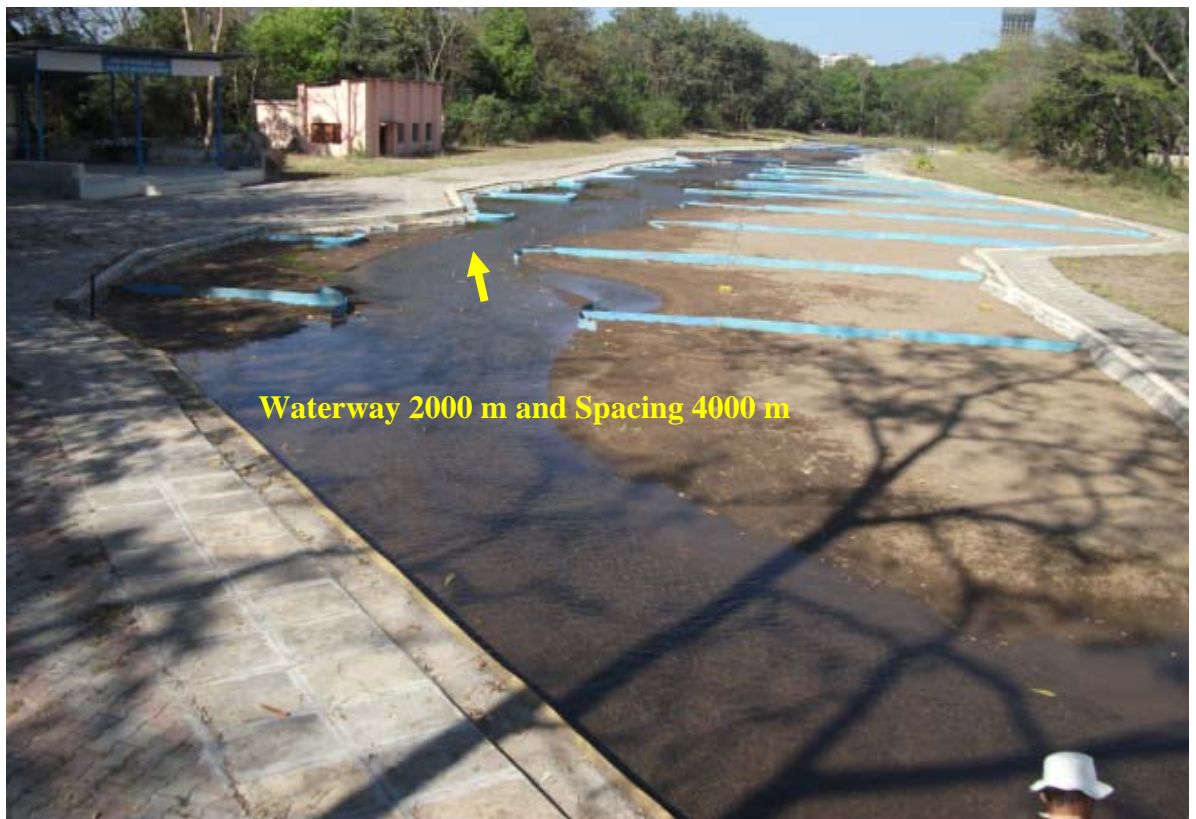
Figure 7.24 a) Flow touching the wings of T-shape groynes, but no shoal flushed and sediment motion
