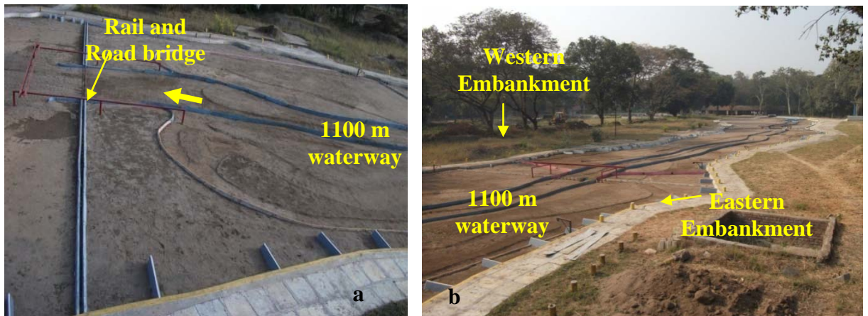
Figure 7.42 a) Channel view of model showing channel configuration at rail-cum-road bridge b) View of model showing channel configuration downstream of Kosi Barrage
