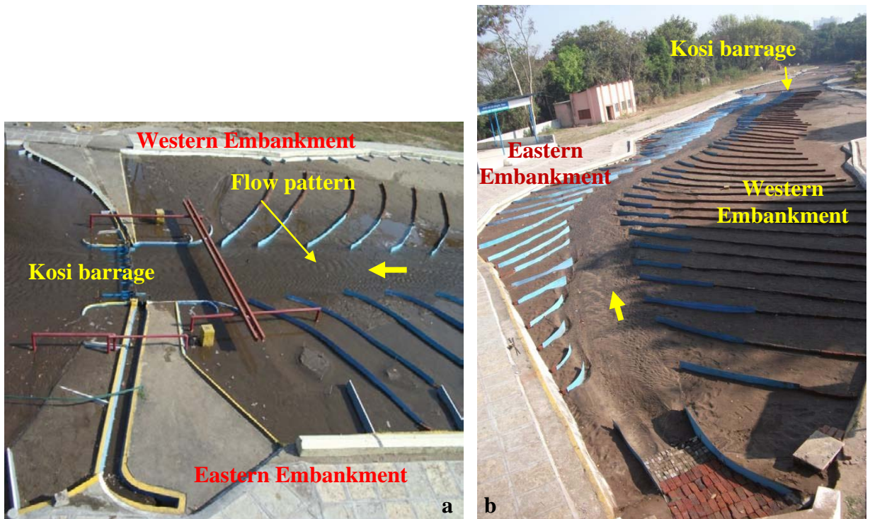
Figure 7.52 a) Side view of model with a discharge of 15586 \text{ m}^3/\text{s} at Barrage b) Upstream view of model showing bed formation after a discharge of 15586 \text{ m}^3/\text{s}
