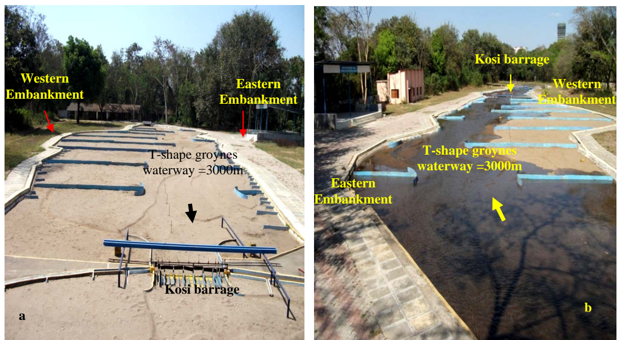
Figure 7.20 b) Downstream and Figure 7.21 Upstream view with T-shape groynes for water way of 3,000 m in the model with Discharge of 15,586 \text{ m}^3/\text{s}
