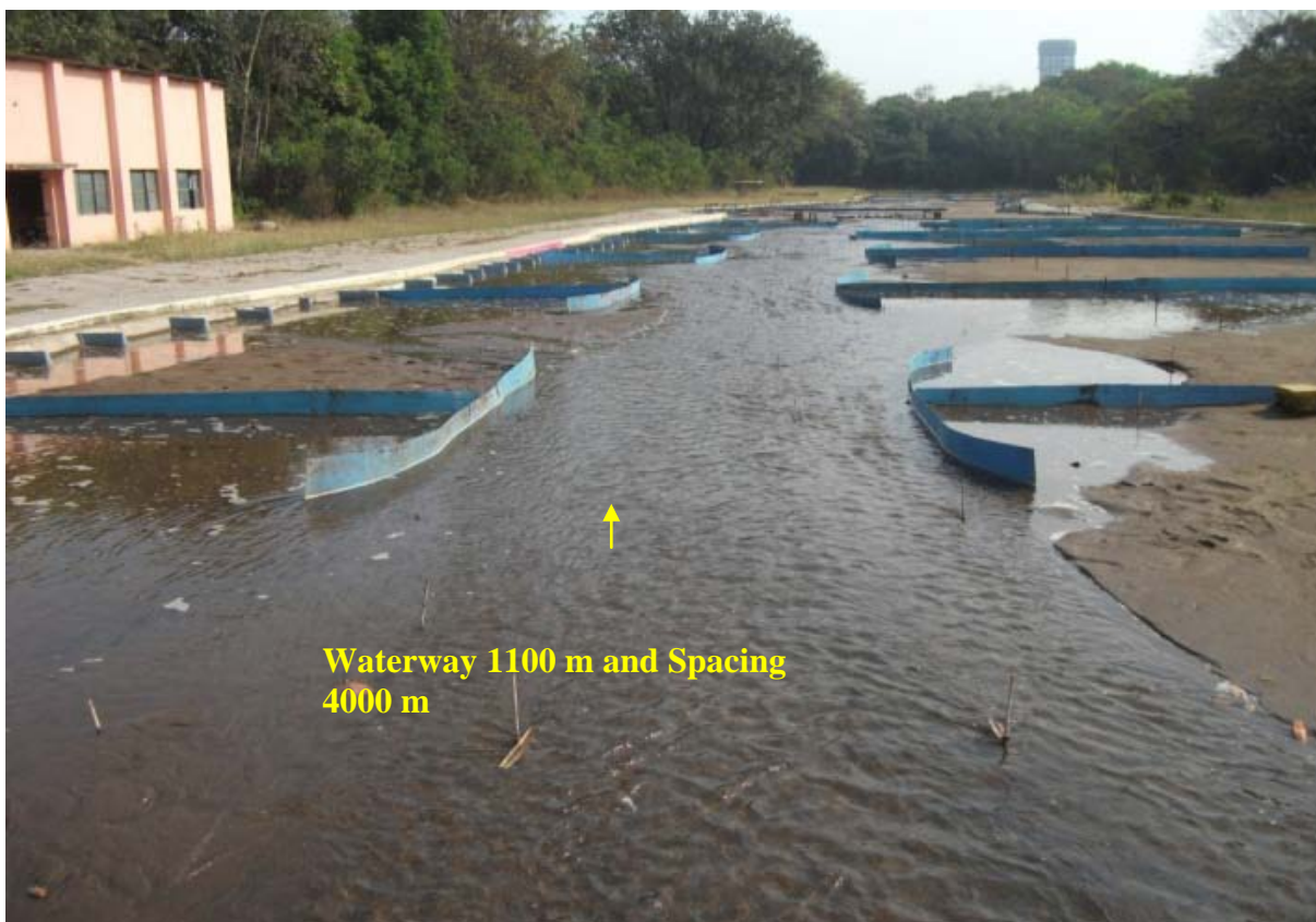
Figure 7.28 a) Closer view showing formation of regime channel in the model
