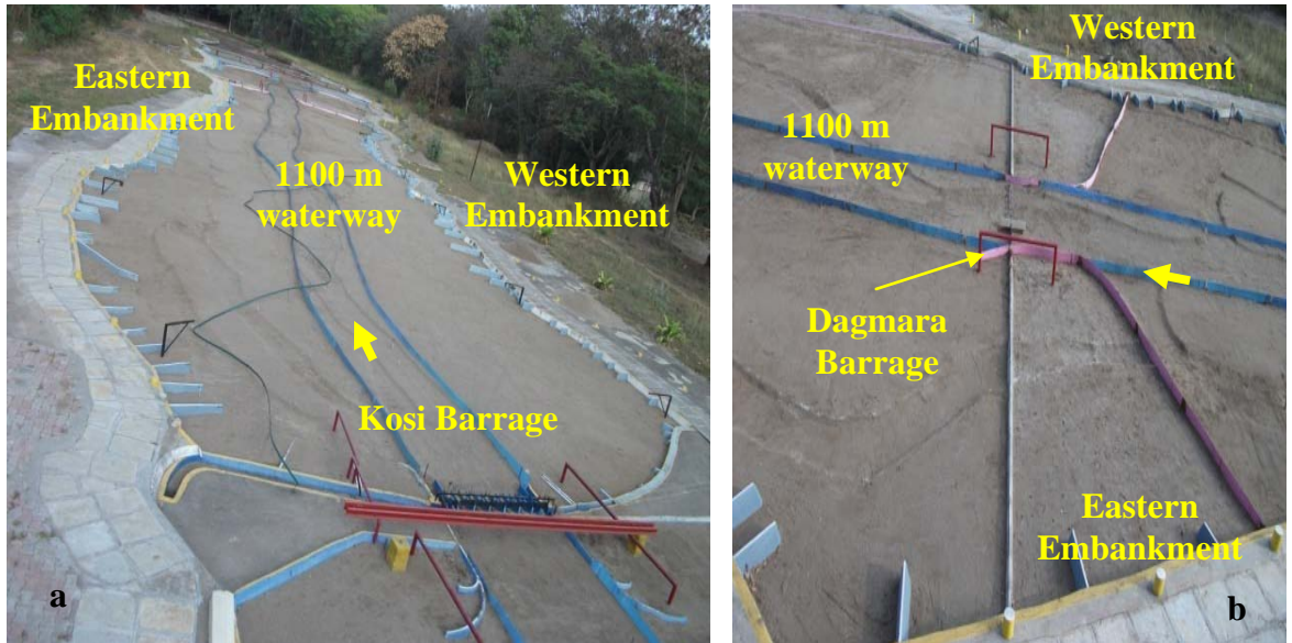
Figure 7.41 a) Channel configuration showing position of embankment from Kosi Barrage to rail-cum-road bridge b) View of model showing channel configuration at Dagmara Barrage
