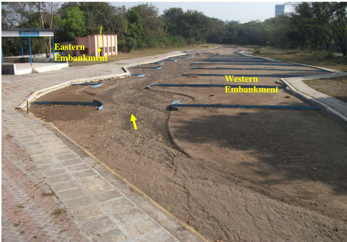
Figure 7.25 Flow touching the wings of T-shape groynes, but no sediment motion took place
