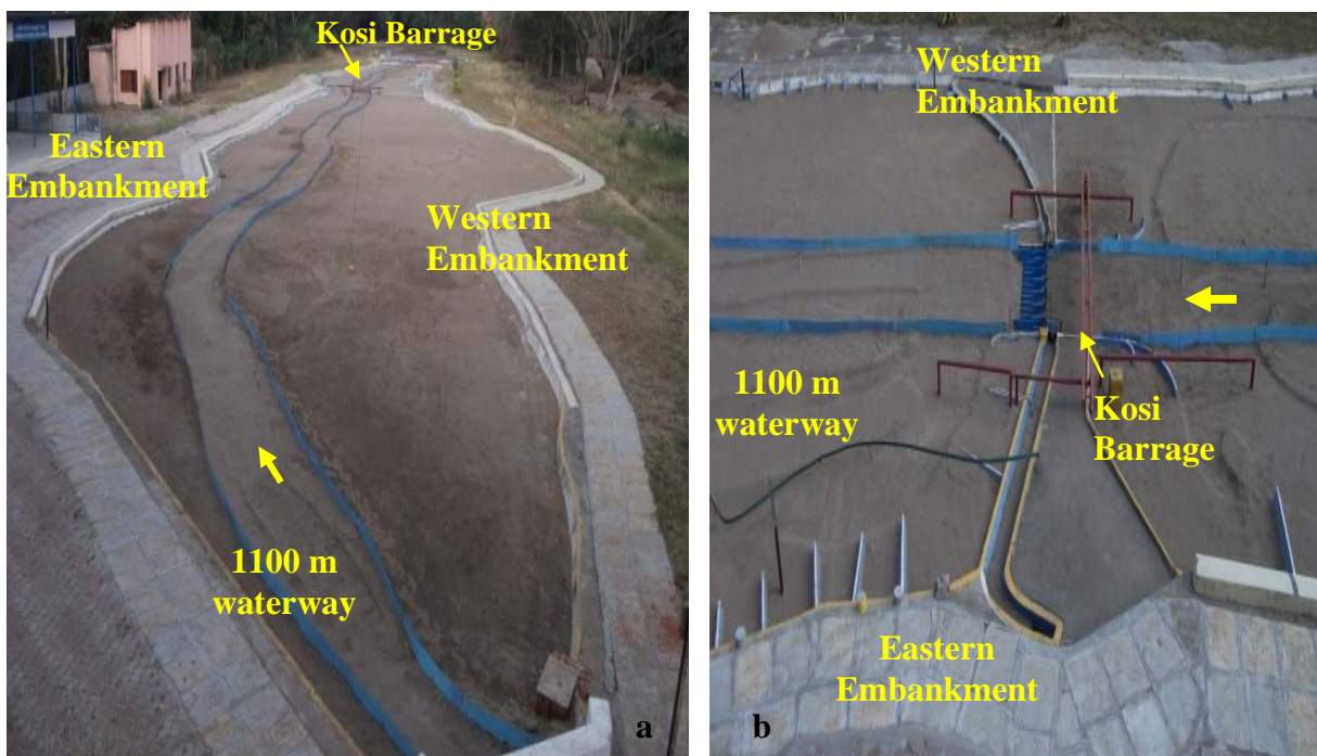
Figure 7.40 a) Upstream view showing position of embankment from Chatra to rail-cum-road bridge b) View of model showing channel configuration at Kosi barrage
