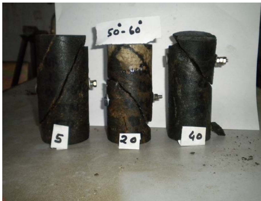
Fig.4.21d Failure of jointed reinforced rock under triaxial compression
