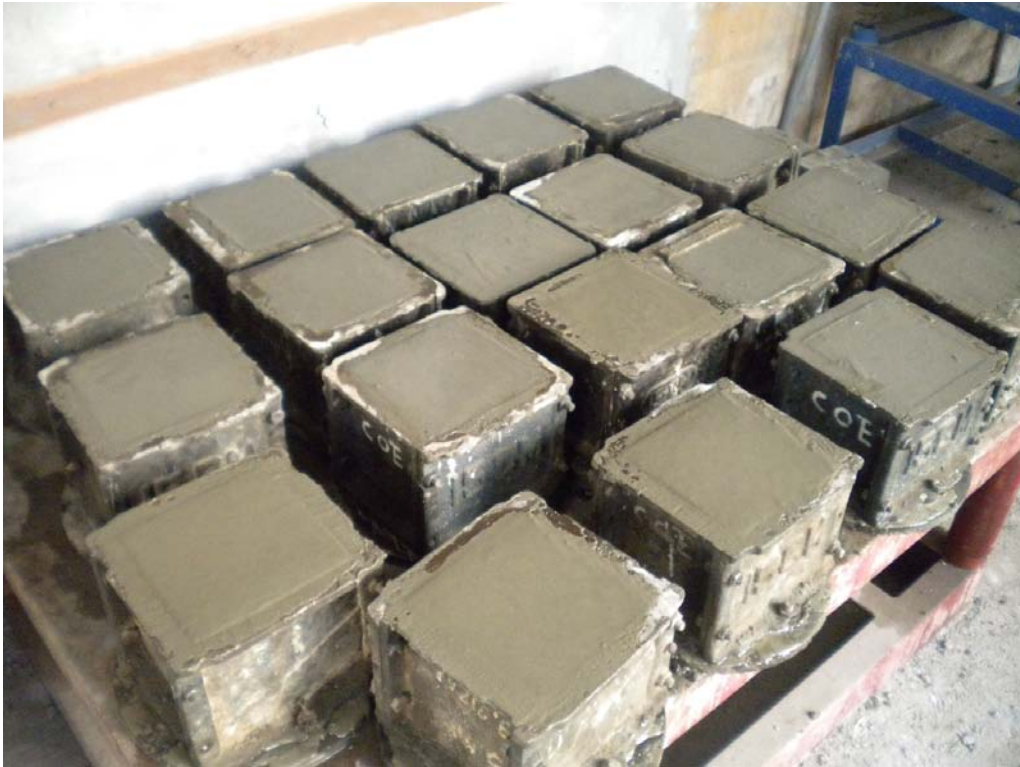
Fig. 3.6a Casting of concrete blocks
