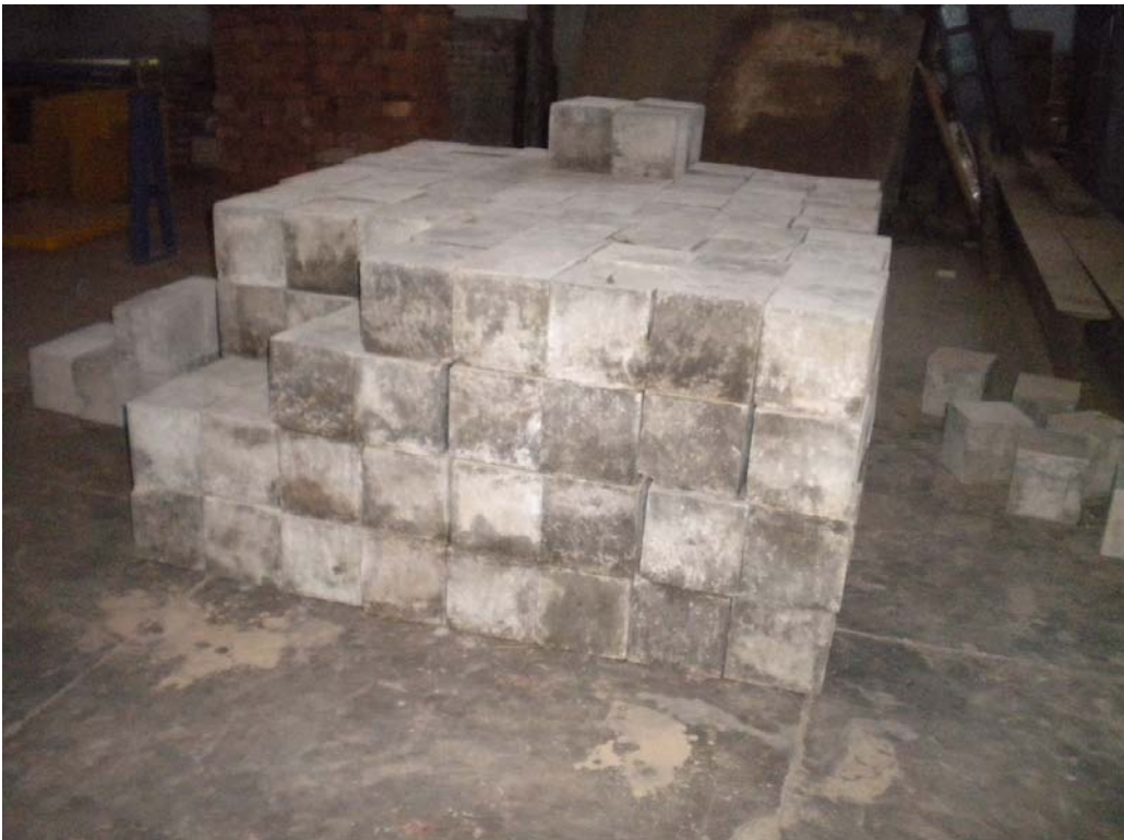
Fig. 3.6b Prepared concrete blocks of size 150 mm x 150 mm x 150 mm
