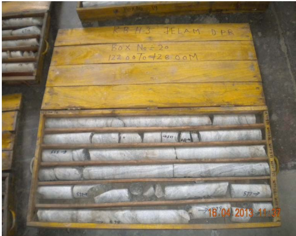
Fig.3.17 Natural rock cores obtained from the site
