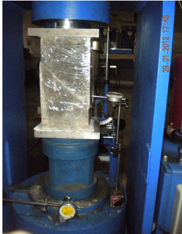
Fig. 3.16 Testing of specimens under uniaxial compression
