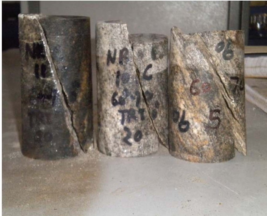
Fig.4.21c Failure of jointed unreinforced rock under triaxial compression
