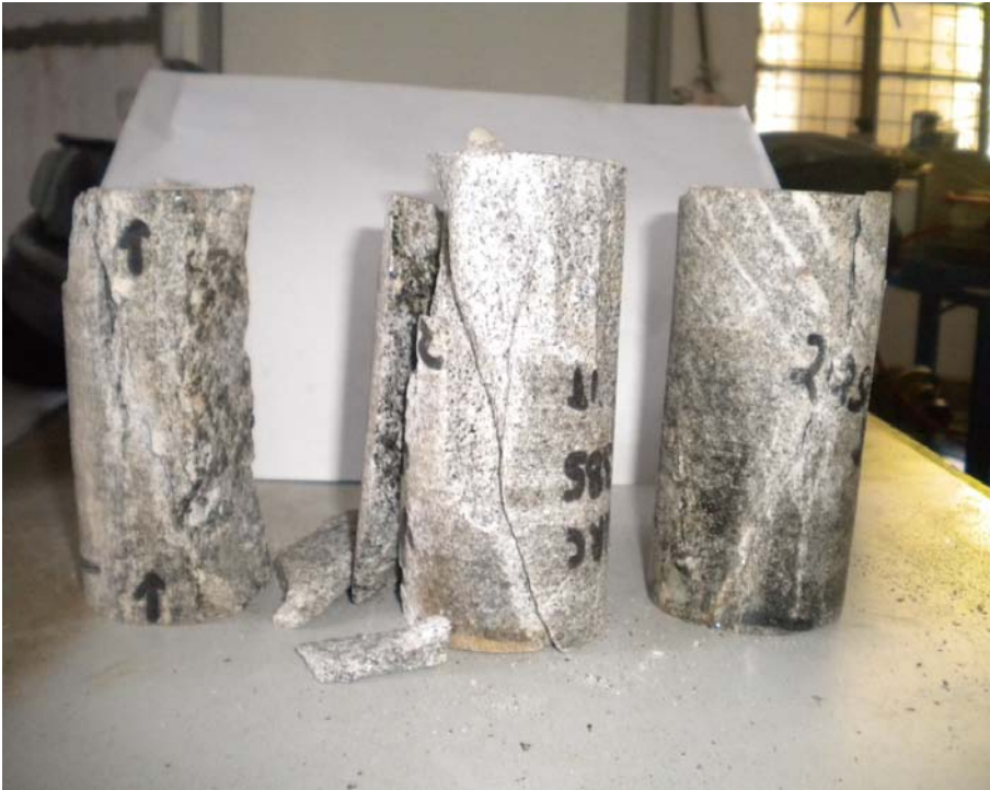
Fig.4.17a Failure of intact rock under uniaxial compression
