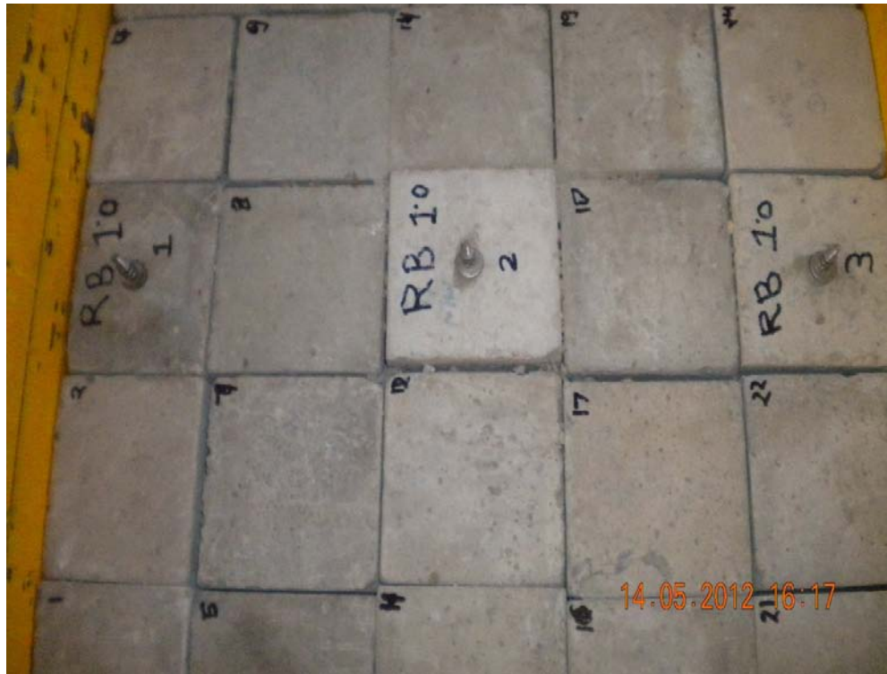
Fig. 3.10 Reinforced specimen in shear box
