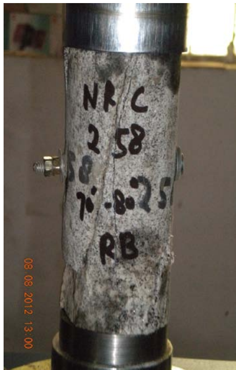
Fig.4.21b Failure of Reinforced jointed rock under uniaxial compression
