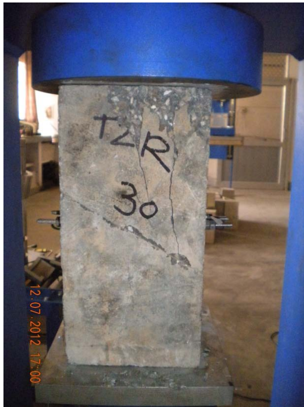
Fig.4.15 Failure in specimens of syntactic reinforced jointed rock
