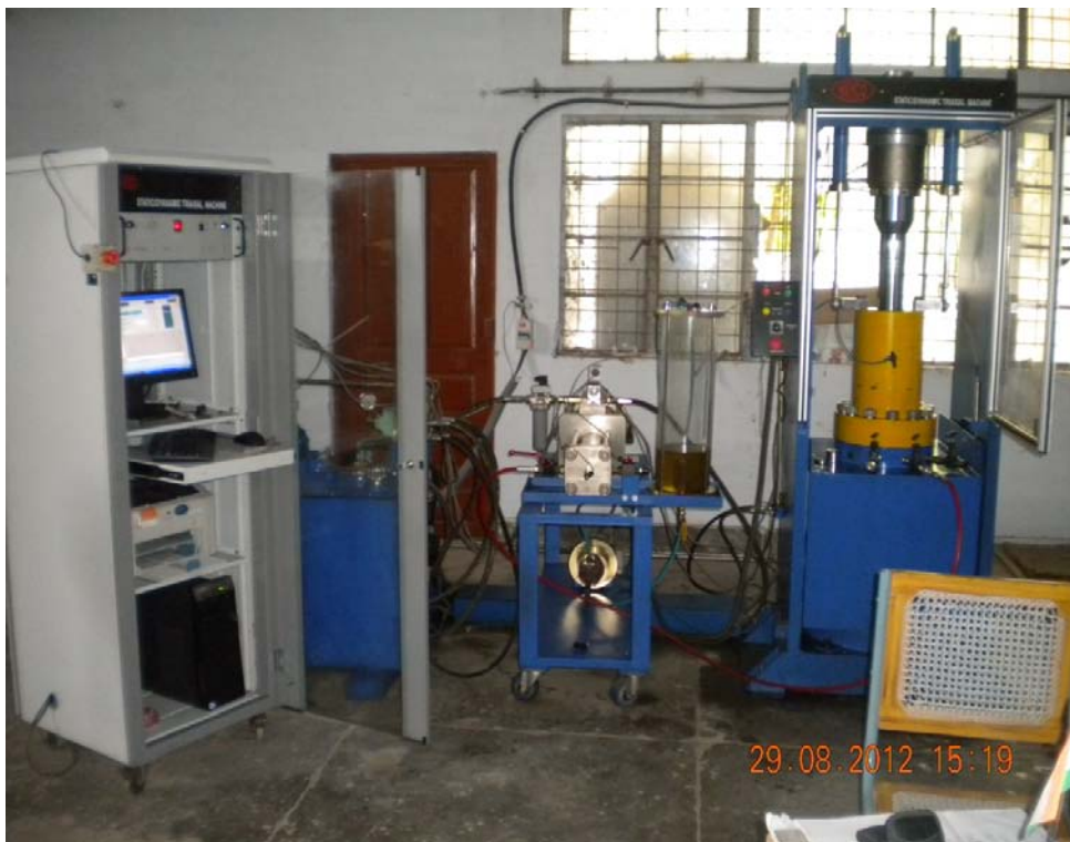
Fig. 3.20 Servo-controlled static / dynamic triaxial machine
