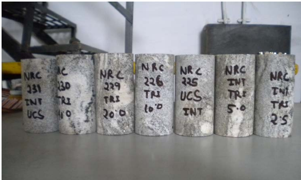
Fig. 3.19a Prepared specimens of intact natural rock
