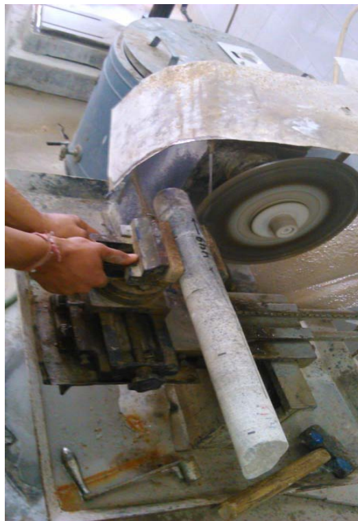
Fig. 3.18 Cutting operation of core to prepare specimens
