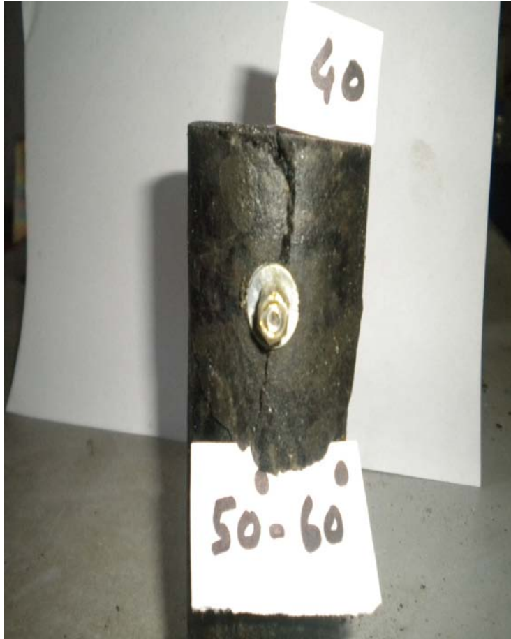
Fig.4.21e Failure of jointed reinforced rock under triaxial compression
