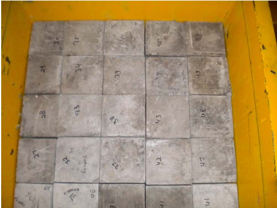
Fig. 3.8 Filling of shear box with 150 mm 3 concrete blocks
