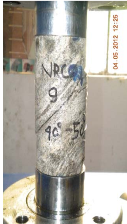
Fig. 4.21a Failure of unreinforced jointed rock under uniaxial compression
