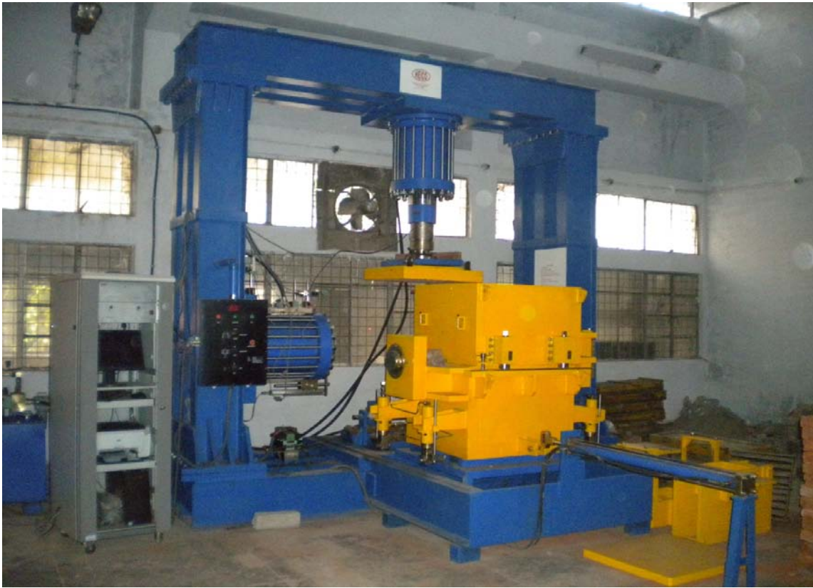
Fig.3.2 Servo-controlled large direct shear test machine
