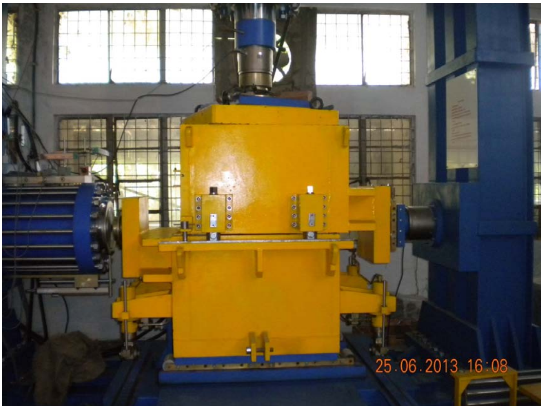
Fig. 3.3 Large shear box of size 750 mm x 750 mm x 1000 mm
