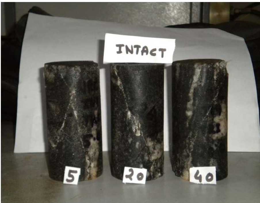
Fig.4.17b Failure of intact rock under triaxial compression
