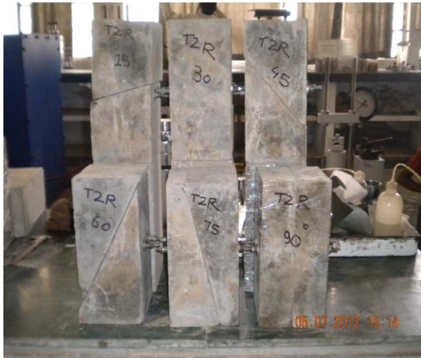
Fig. 3.13 Prepared reinforced specimens of synthetic rock
