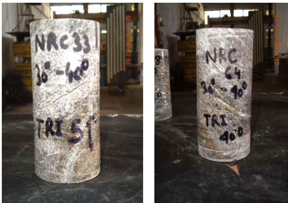
Fig. 3.19b Prepared specimens of jointed natural rock
