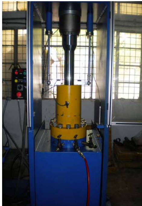
Fig.3.22 Fixing of specimen in triaxial cell
