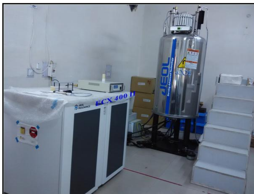
Fig. 2.8: JEOL 400 MHz NMR spectrometer (Model ECX 400 II).
