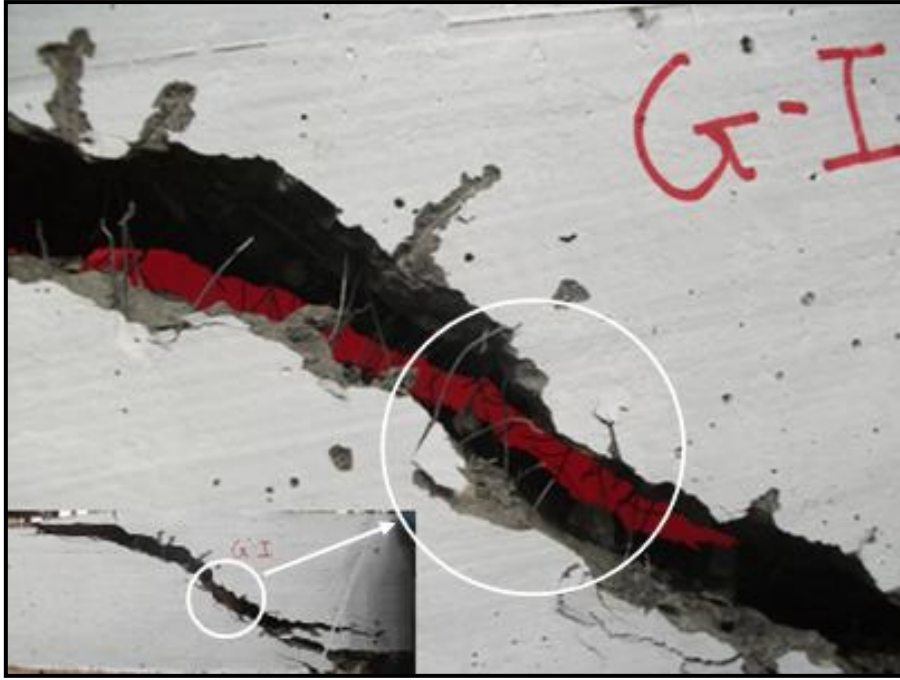
Fig. 4.44: Illustration of the pull-out mode of fibre failure observed in the beam specimens
