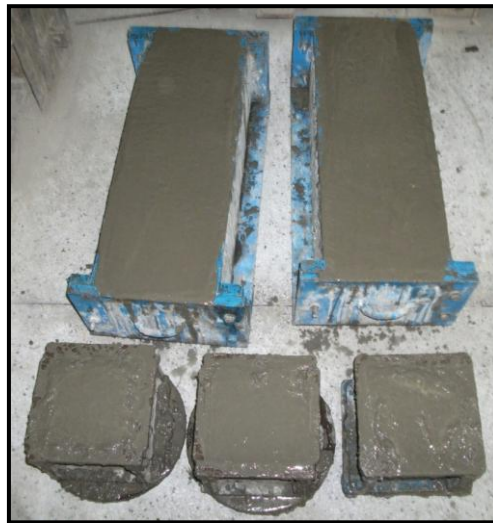
Fig. 3.6: A sample of one set of prismatic specimens and their control cubes soon after casting
