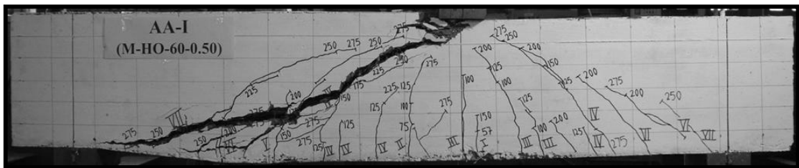
(f) 0.50 % V_f of 60 mm long hooked-end steel fibres
