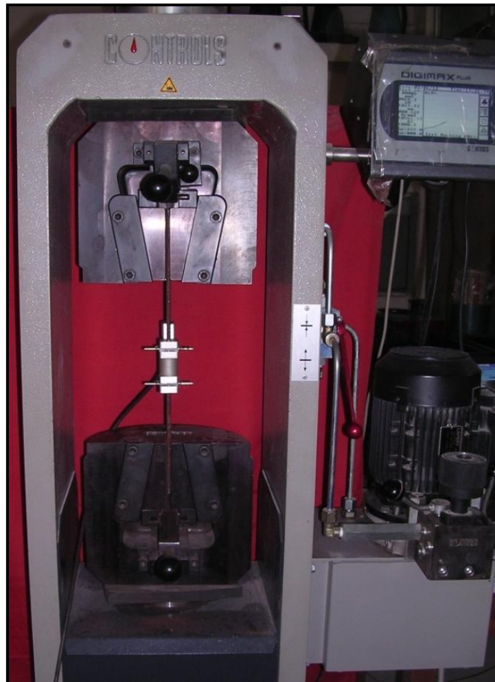
Fig. 3.3: Tension testing of the steel reinforcement bars.
