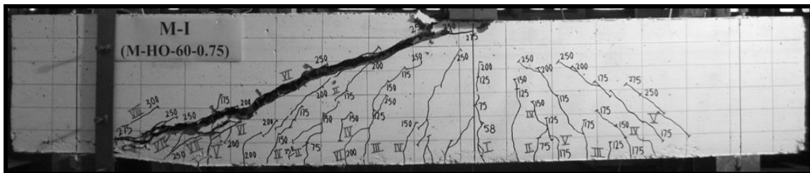
(g) 0.75 % V_f of 60 mm long hooked-end steel fibres
