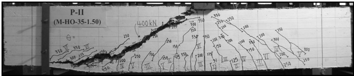
(e) 1.50 % V_f of 35 mm long hooked-end steel fibres
