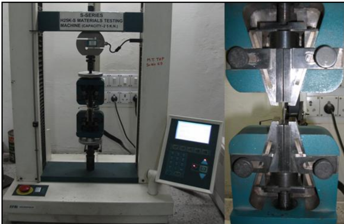
Fig. 3.1: Tension testing of the steel fibres
