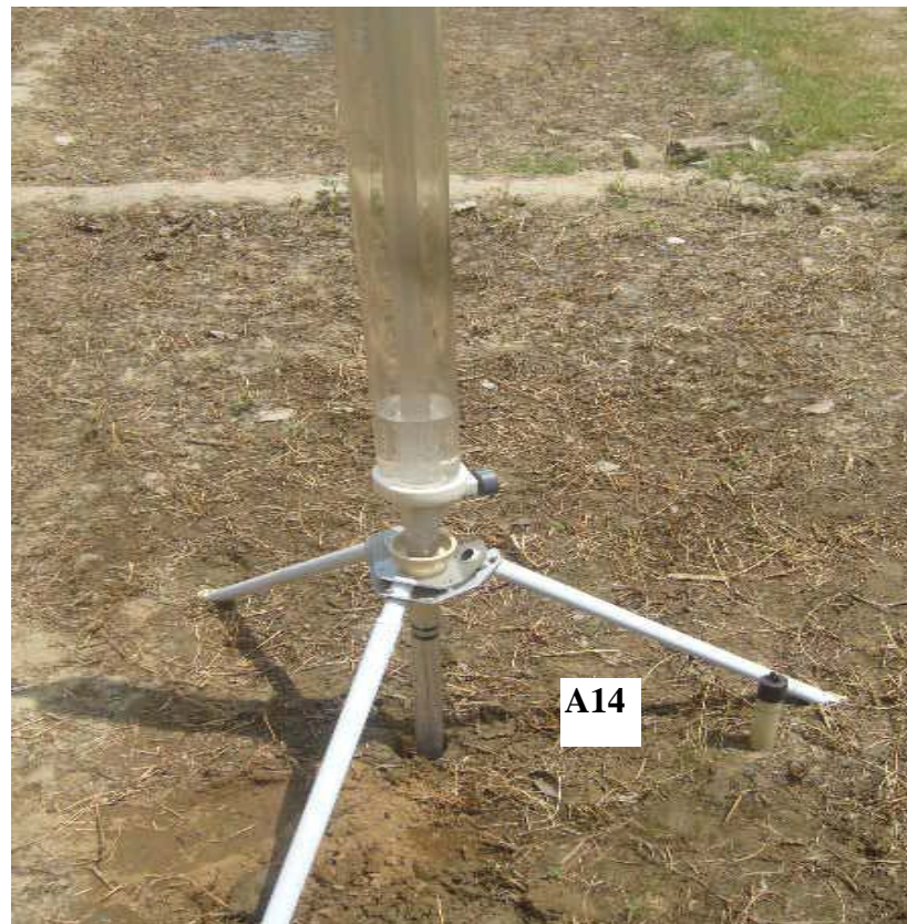
Fig. 3.16 Guelph Permeameter in operation in test spots A21 and A14
