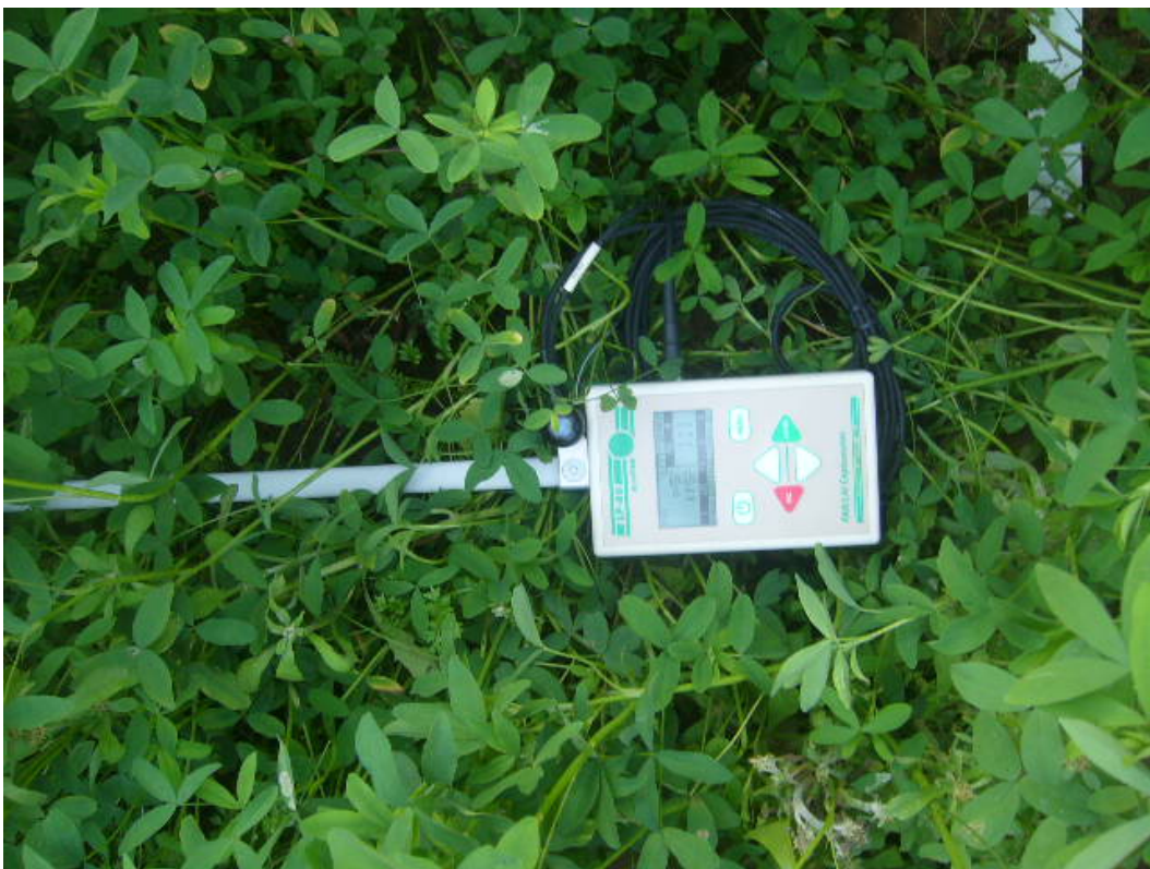
Fig. 3.28 LAI measurement with LP-80 Ceptometer during berseem season 2
