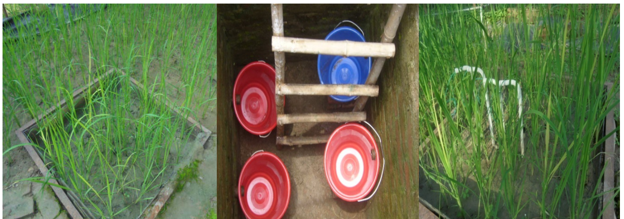
Fig. 3.7 Lysimeters and drainage collection arrangements
