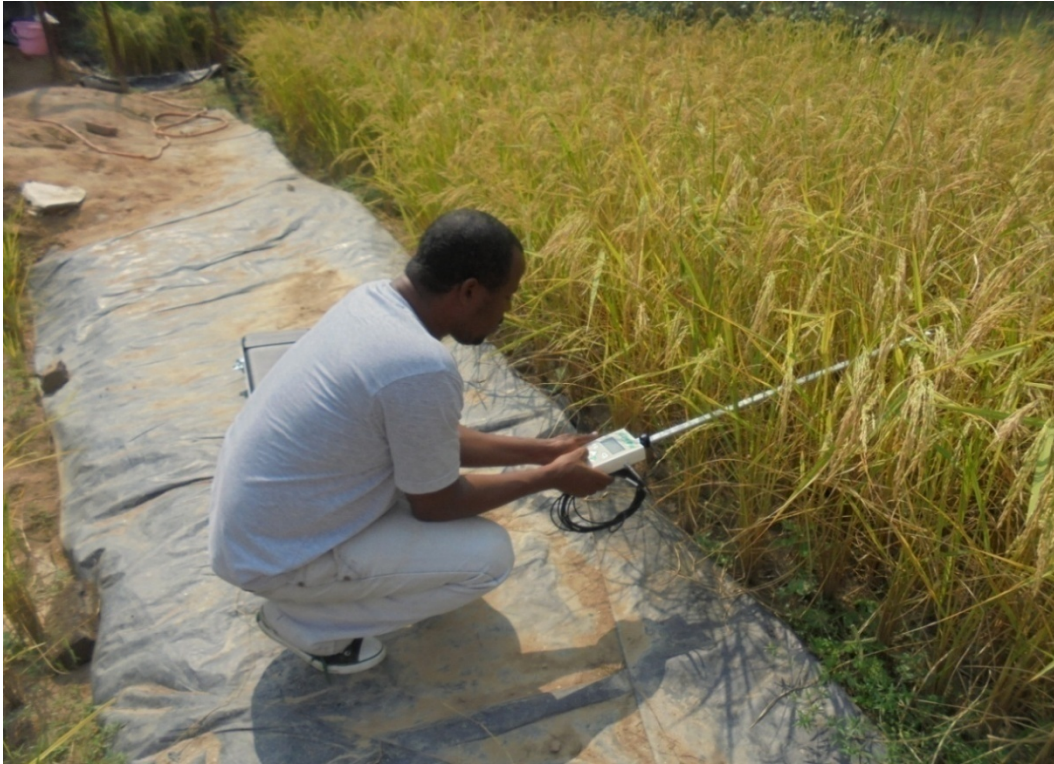
Fig. 3.27 LAI measurement with LP-80 Ceptometer during rice season 2
