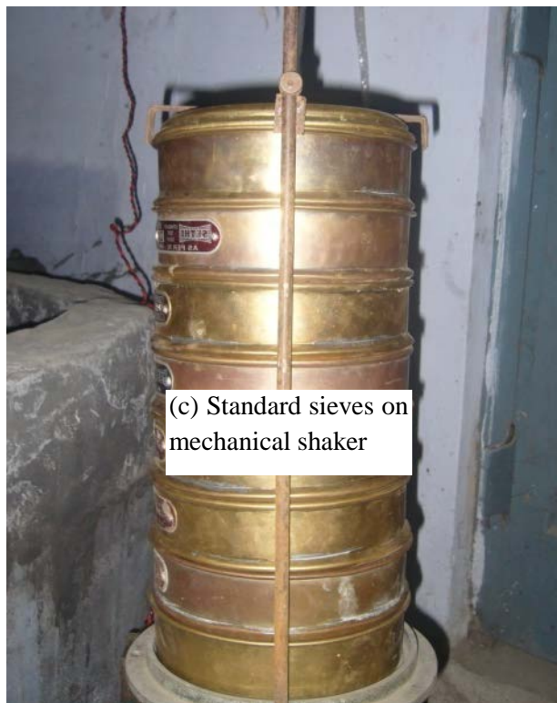
Fig. 3.8 Grain size distribution analysis
