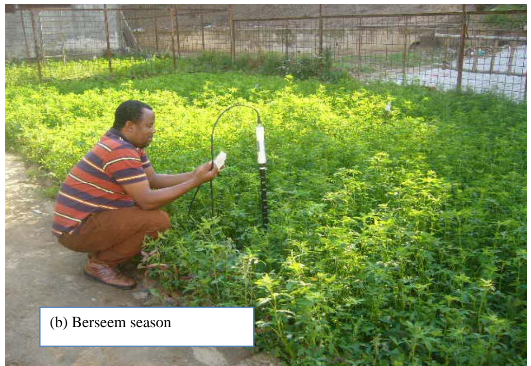
Fig 3.5 Monitoring soil moisture using profile probe
