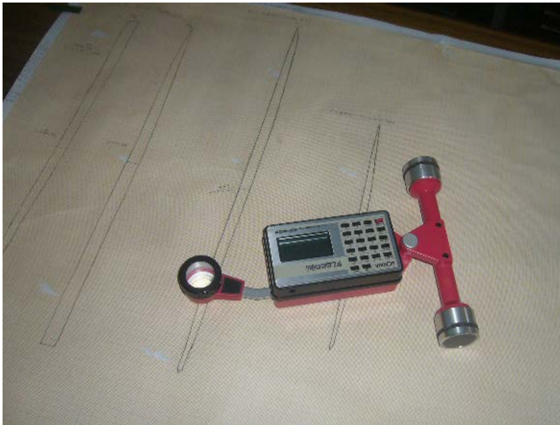
Fig. 3.26 Digital planimeter for measurement of leaf profile during rice season 1
