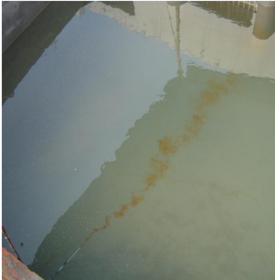
Figure 6.2 Dye injected at bed of the forebay
