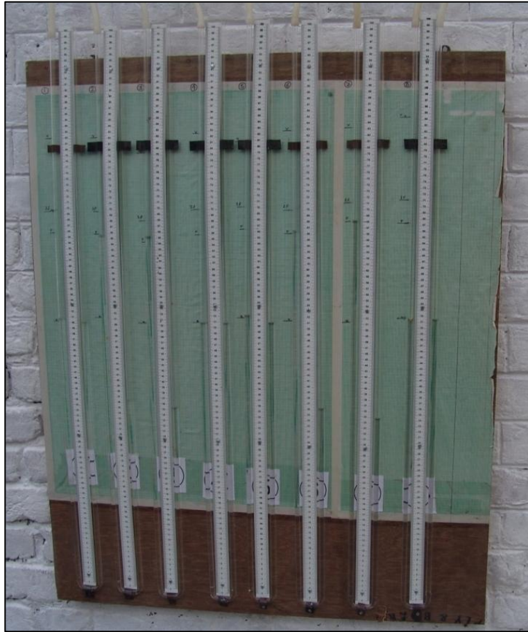
Figure 3.15 Manometer board used to measure pressure difference
