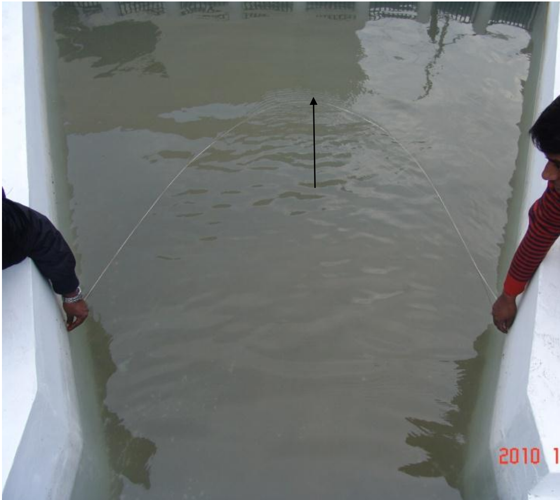
Figure 6.9 Shape of a thread placed on water surface
