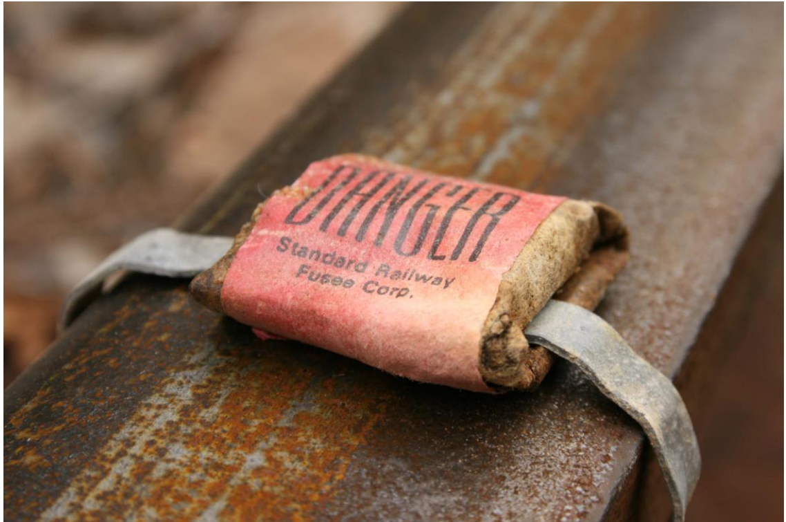
Figure 2.3: Railway track detonator.
