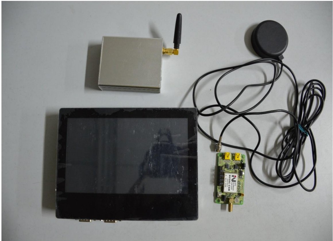
Figure 6.5: Development board, GNSS receiver, Antenna and GSM modem.
