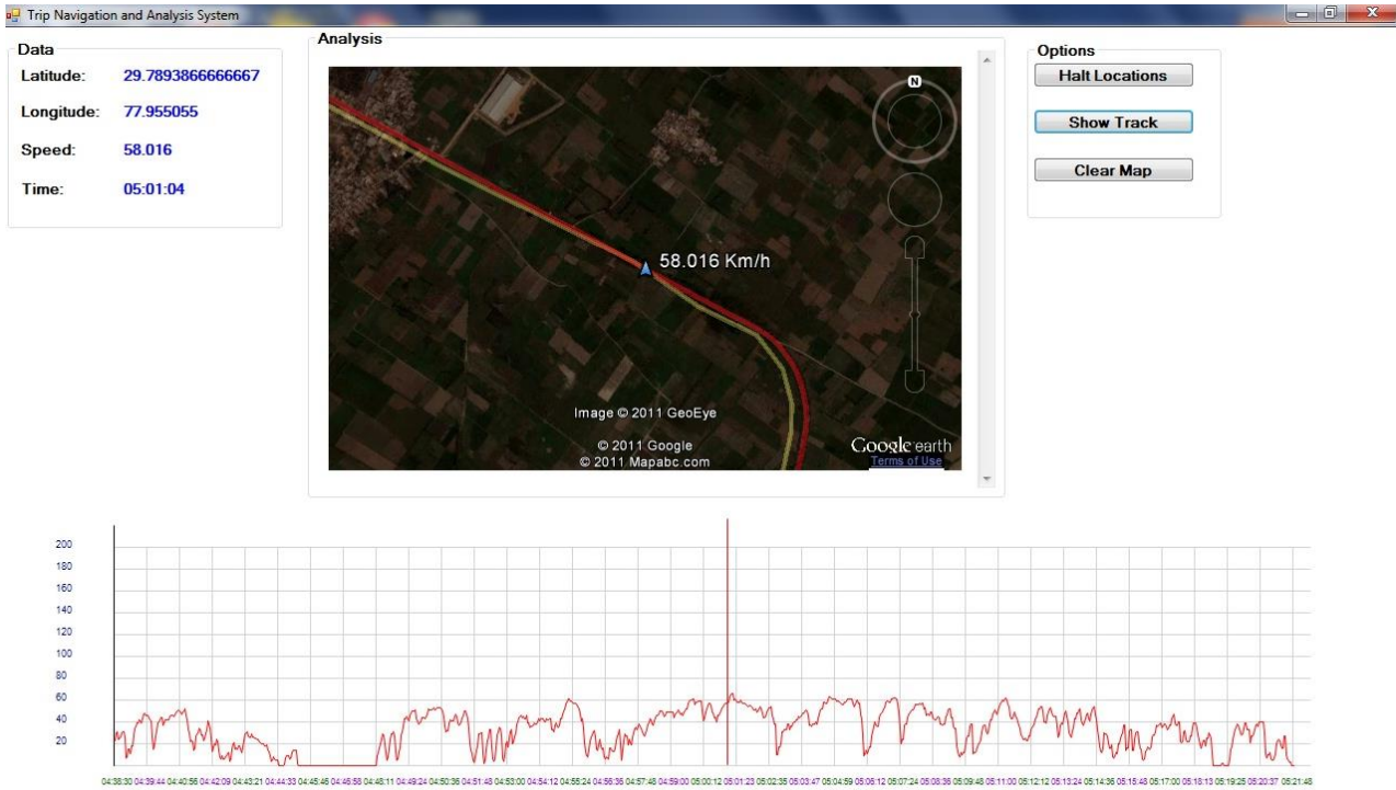
Figure 8.11 (a): Location with speed on Google Earth at time 05:01:04 UTC while cursor moving on graph of a car trip.
