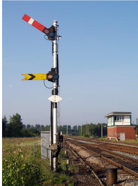
Figure 2.6: Semaphore signal combined with warner signal.
