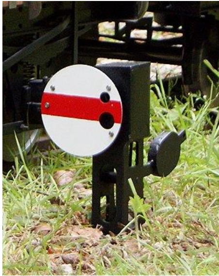
Figure 2.7: Disc signal for shunting.
