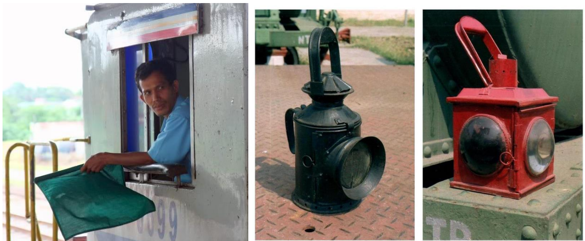
Figure 2.4: Flag and lamps for signaling.
