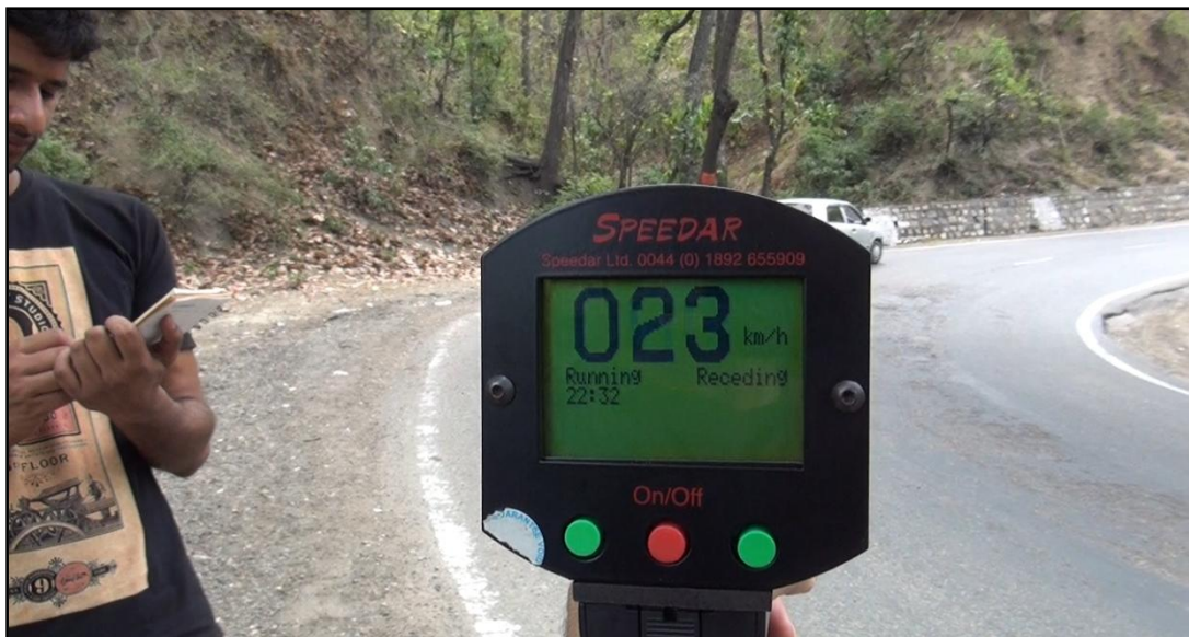
Figure 7.7 SPEEDAR speed gun used for measuring FFS
