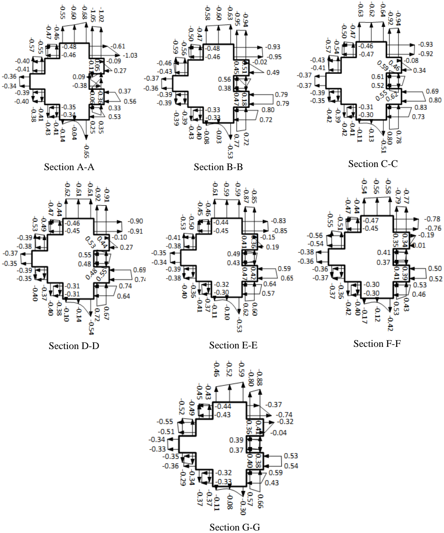
Fig. 5.80 Cross-sectional variation of mean wind pressure coefficients ( C_{p,mean} ) on model-H at 150^\circ wind incidence angle
