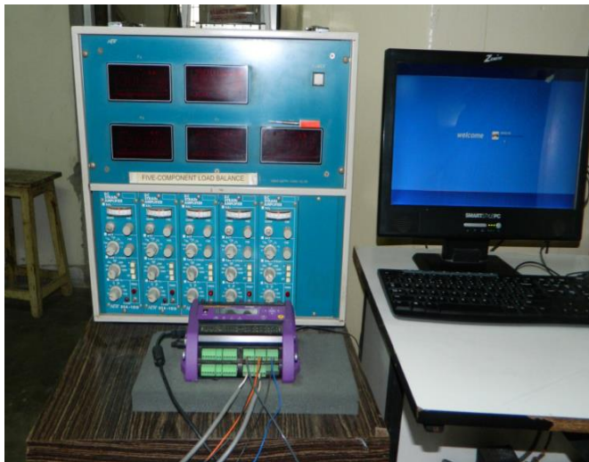
Photo. 3.5 Display unit for five components Load Cell, Data Acquisition System and Computer
