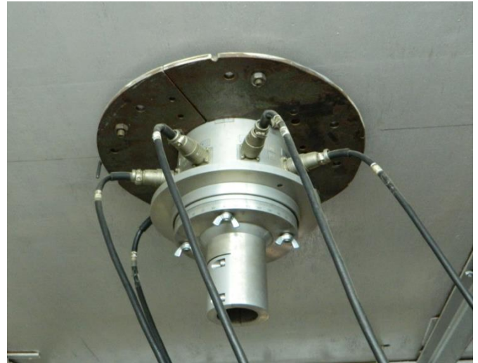
Photo. 3.4 Five component load cell attached to the lower side of the wind tunnel floor
