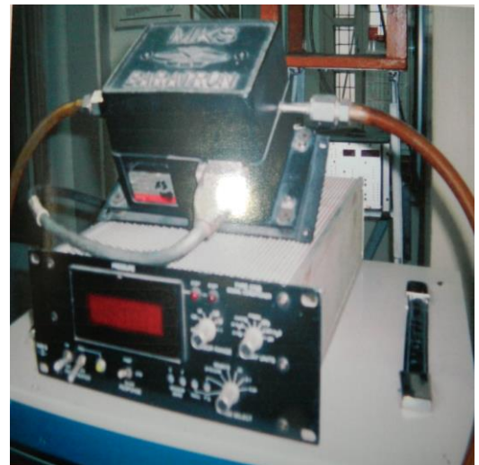
Photo. 3.6 Pressure Transducer: Head and Display unit
