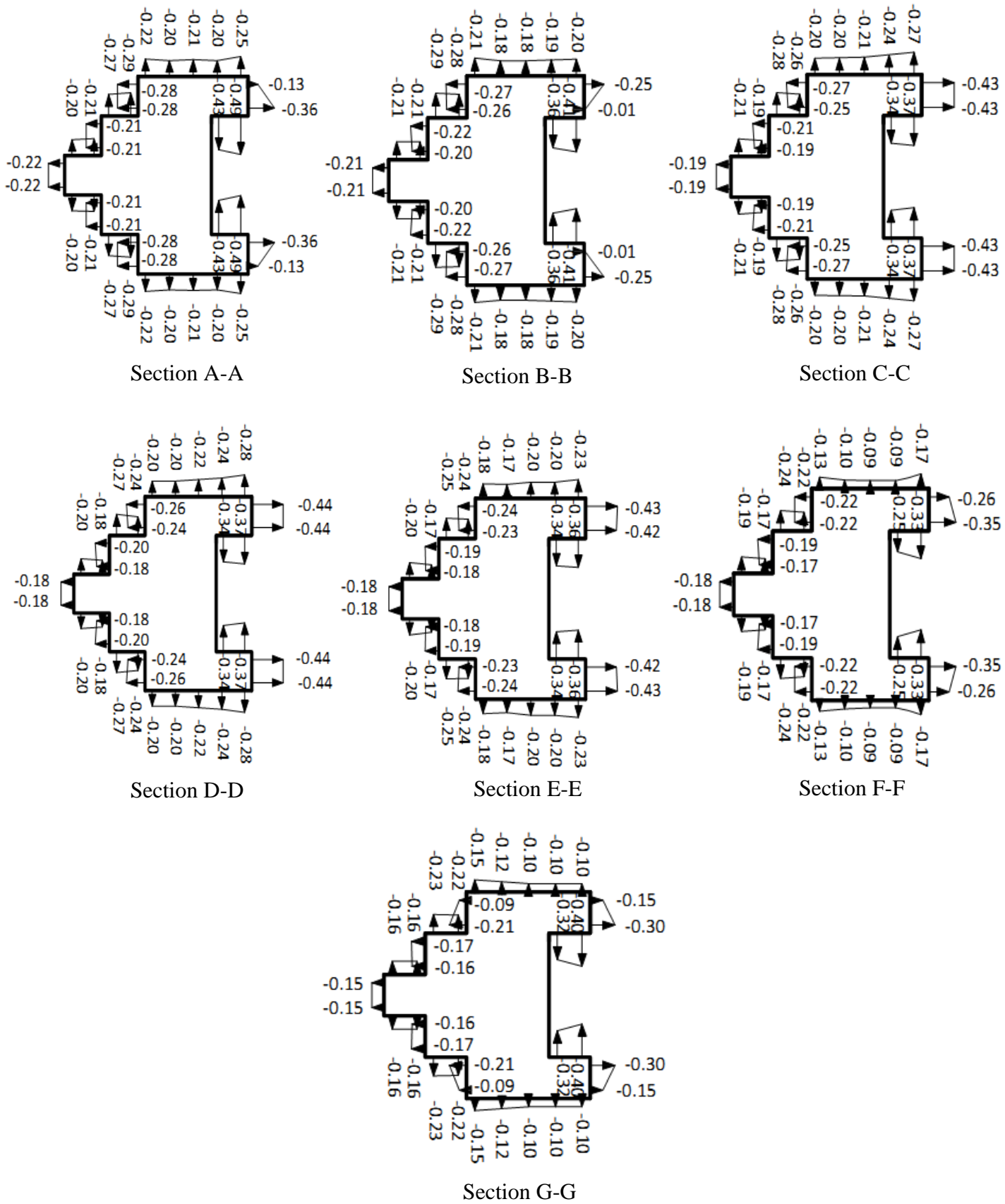
Fig. 5.126 Cross-sectional variation of mean wind pressure coefficients ( C_{p,mean} ) on model-G in front-to-back interference condition
