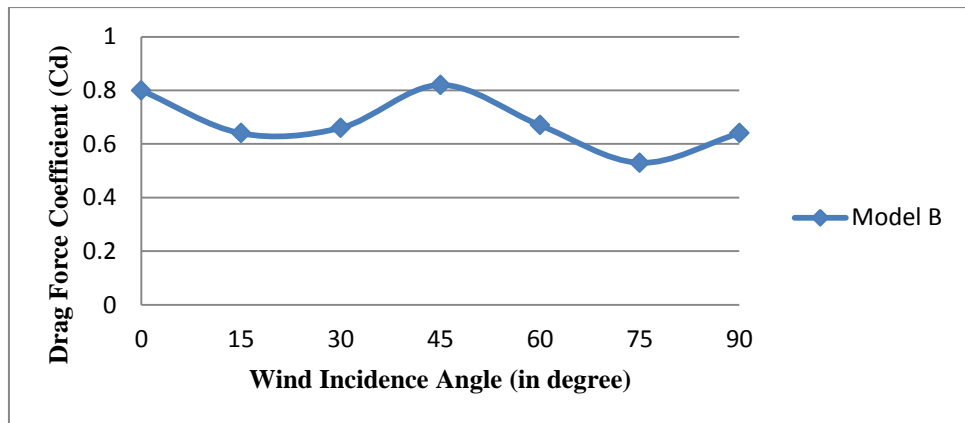
Fig. 4.6 Variation of drag force coefficient on model-B with wind incidence angle
