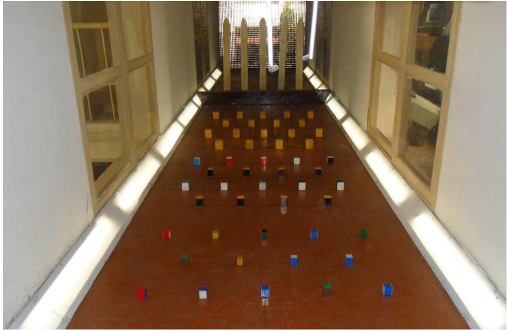
Photo. 3.2 In-side view of wind tunnel showing flow roughening devices
