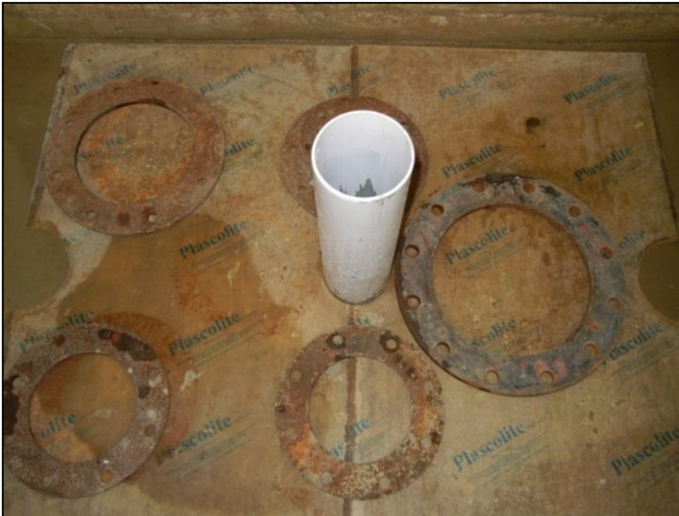
Fig 4.11 Covering nearby area around pier by a transparent perspex sheet prior to start of an experimental run
