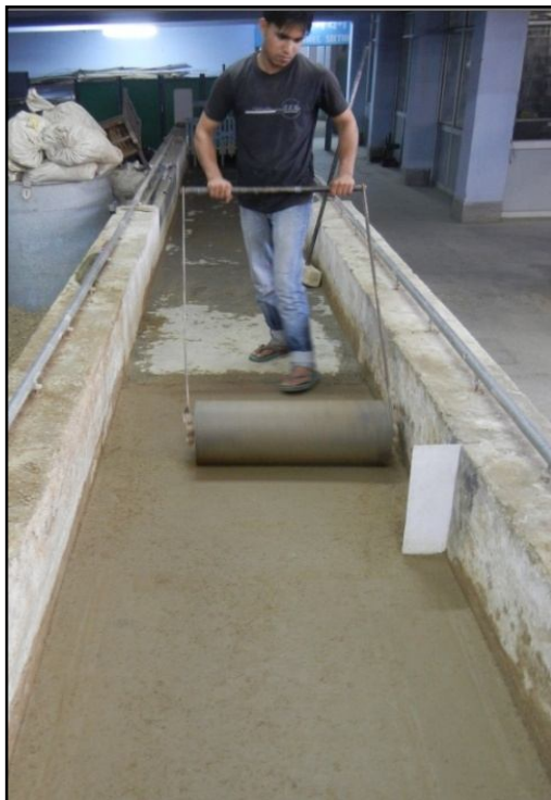
Fig. 4.7 A view of compaction of the channel bed by (a) roller and (b) rammer
