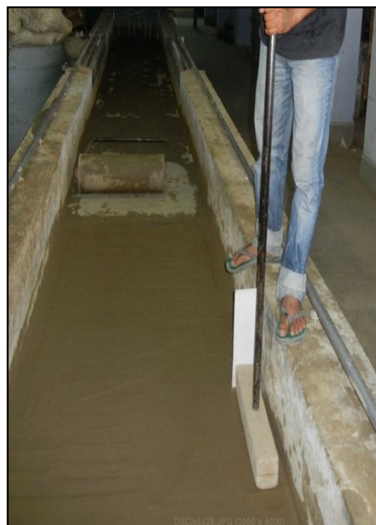
Fig. 4.7 A view of compaction of the channel bed by (a) roller and (b) rammer
