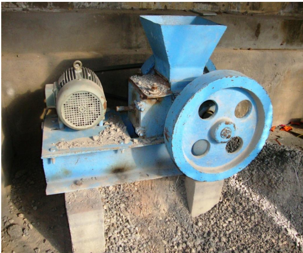
Figure 3.14 Jaw crusher used for crushing of the waste concrete
