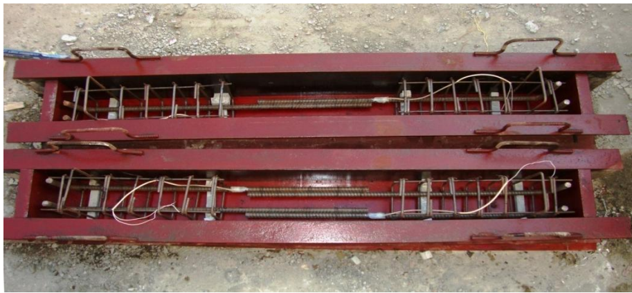
Figure 3.30 A pair of splice beam specimens ready for casting
