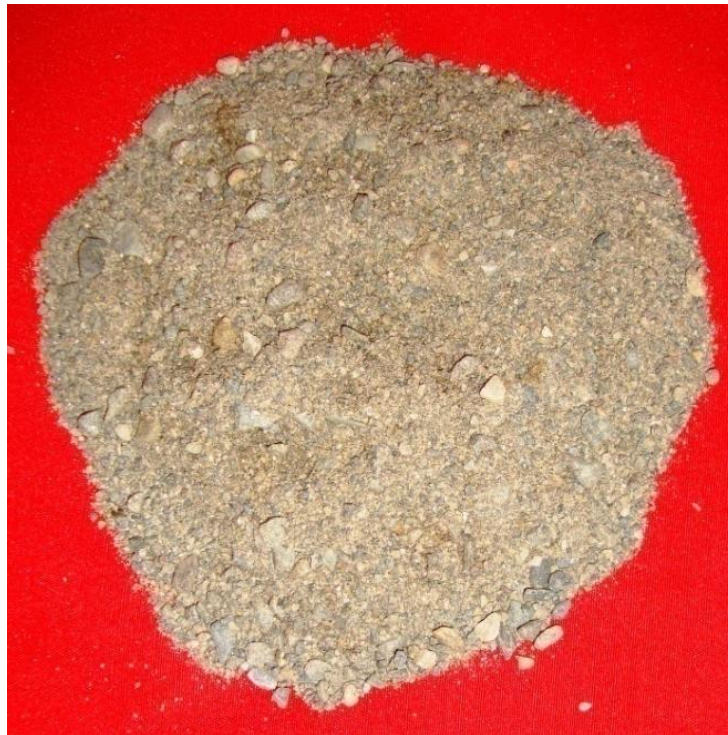
Figure 3.1 A sample of the fine aggregates
