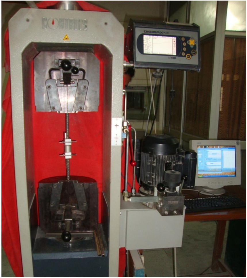
Figure 3.7 Tension testing of a steel reinforcing bar
