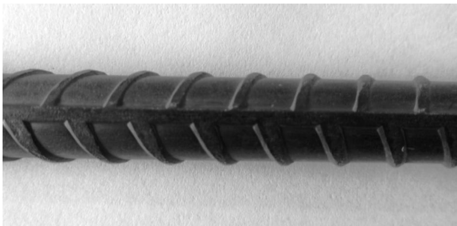
Figure 3.5 Typical rib orientation in the deformed steel bars
