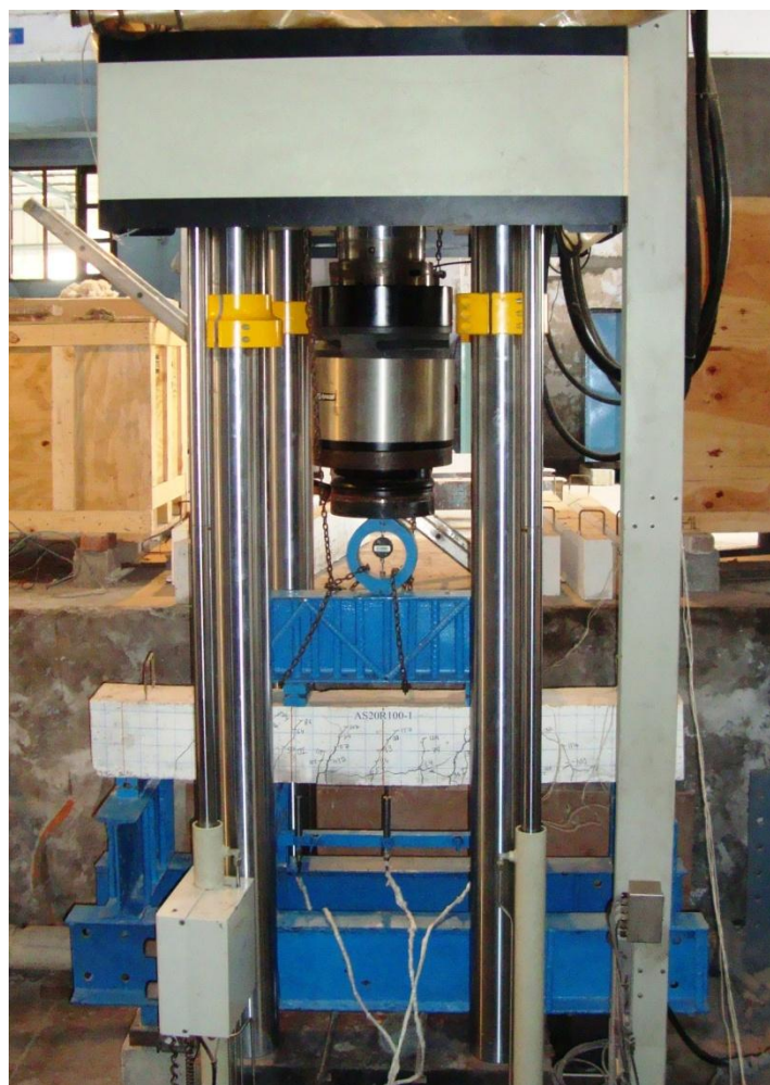
Figure 3.32 Splice beam test in progress
