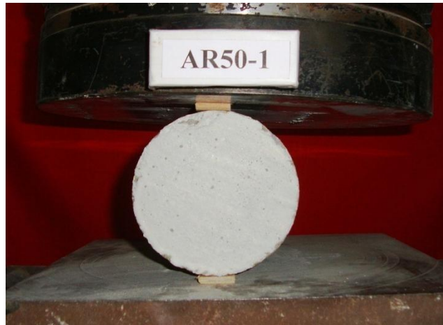
Figure 3.20 Splitting tensile strength testing of a cylinder
