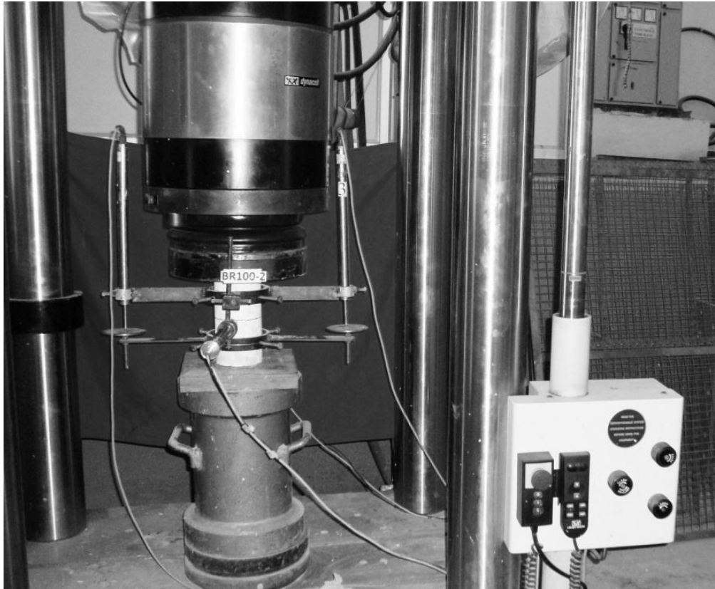
Figure 3.17 Compression testing of a cylindrical specimen
