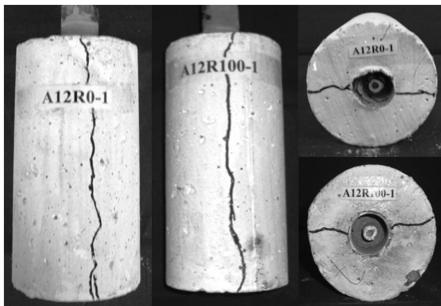
Figure 4. 11 Typical pullout failure induced by through-splitting
