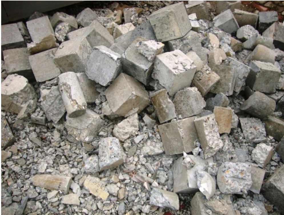
Figure 3.13 Waste concrete specimens used for producing the RCA
