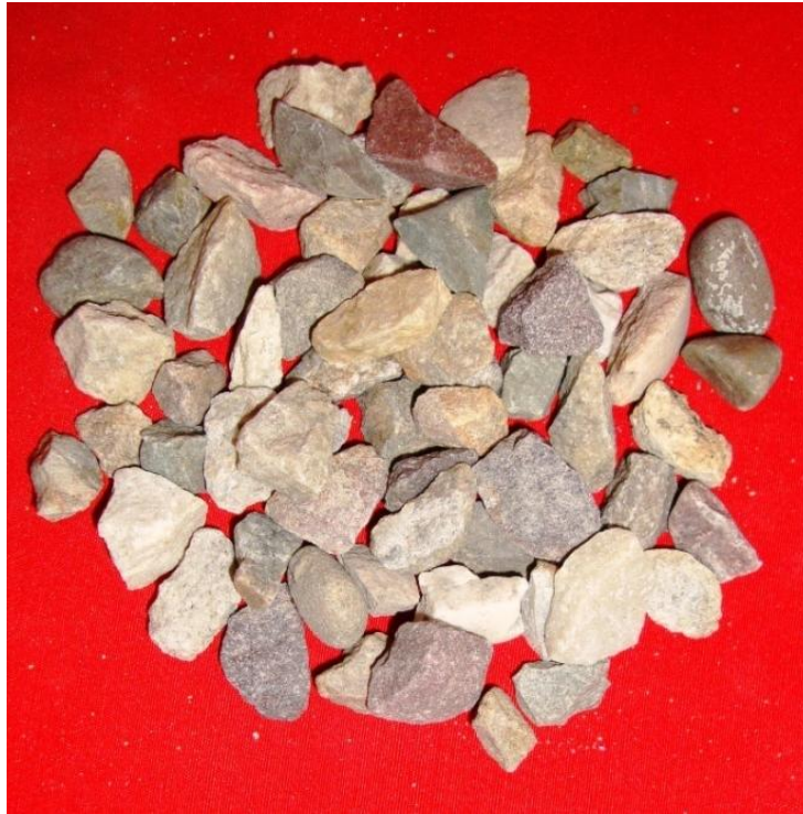
Figure 3.2 A sample of the natural coarse aggregates
