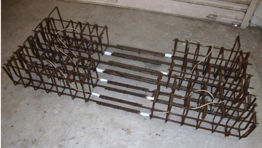
Figure 3.29 A set of reinforcement cages for the splice beam specimens
