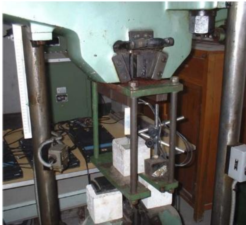
Figure 2.15 Pullout test setup (Xiao and Falkner, 2007)
