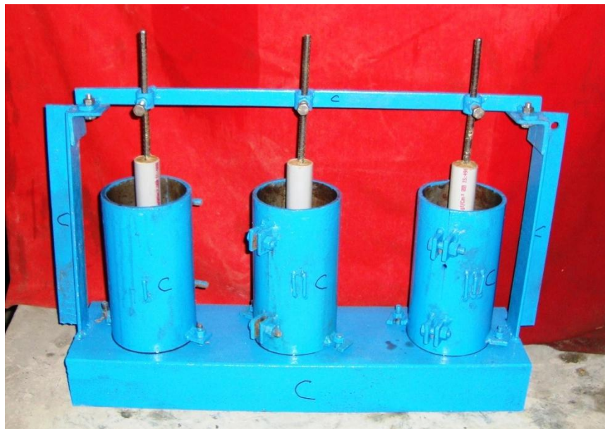
Figure 3.25 Pullout moulds with steel fixture
