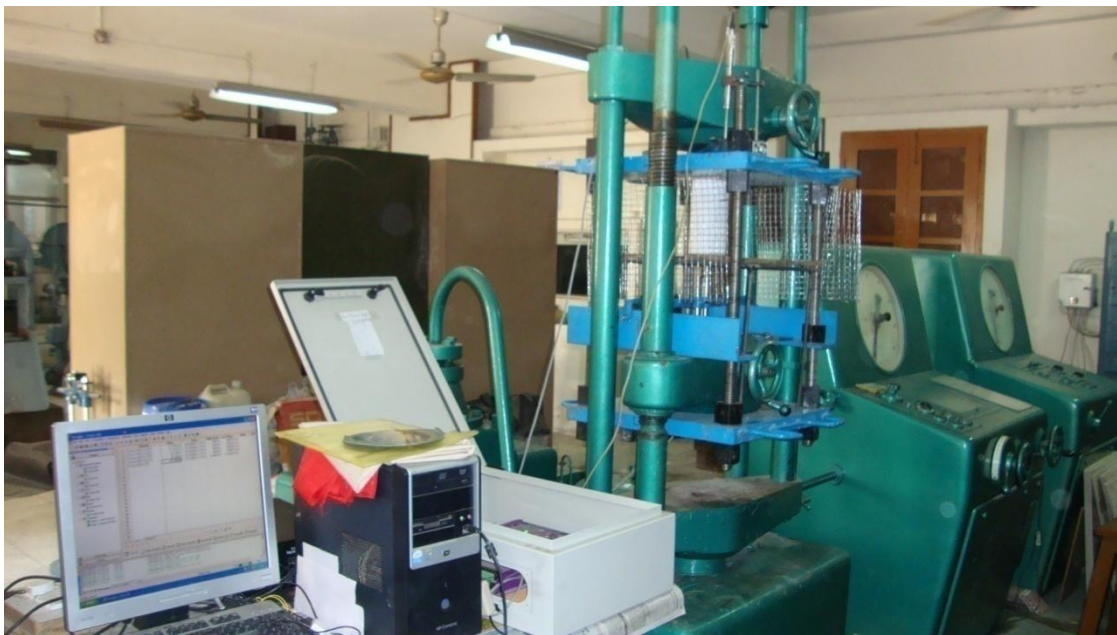
Figure 3.26 Pullout test setup
