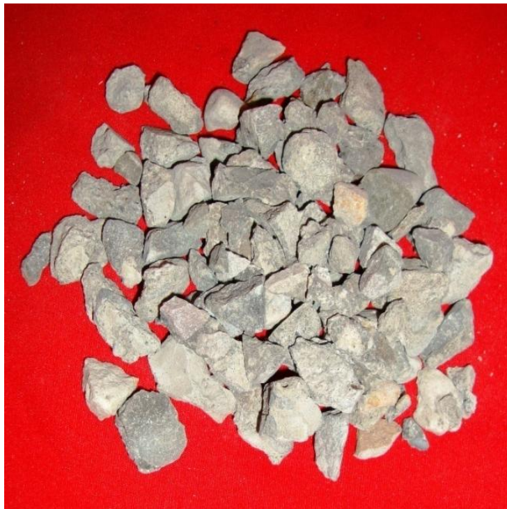
Figure 3.4 A sample of the coarse recycled concrete aggregates
