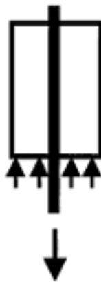
Figure 2.7 Pullout specimen (ACI, 2003)
