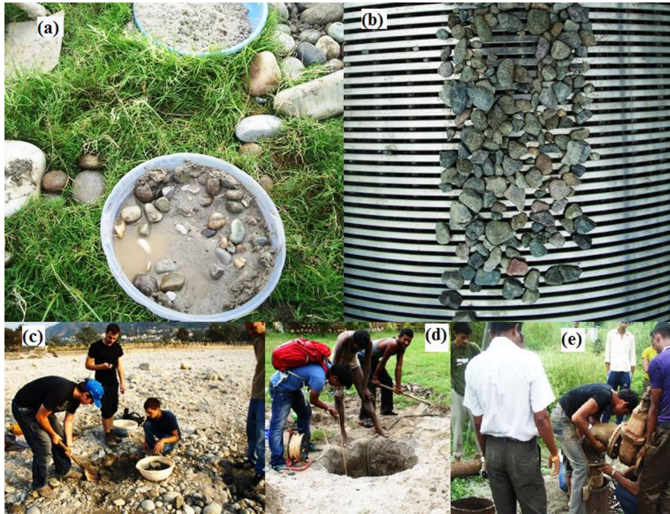
Figure A2 Activities in the RBF site (a) Aquifer material collection from bore hole (b) Filter assemble with pea gravel (c) Riverbed material collection (d) Piezometric water level measuring (e) Preparation of pumping test
