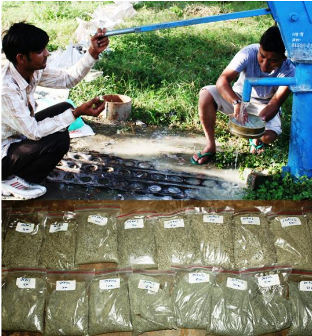
Figure 3.12 Removing bentonite clay from the formation material and sample preparation for sieve analysis
