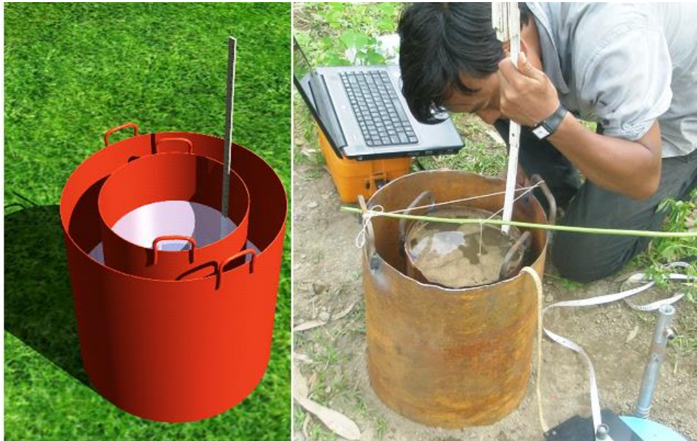
Figure 3.10 During measurement of water level in the double ring infiltrometer
