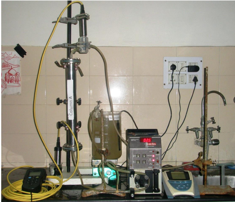
Figure 3.14 Conducting tracer test on the filter media
