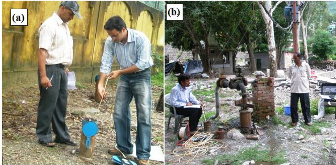
Figure 3.7 (a) Measurement of the water level in the monitoring well, (b) Conducting pumping test.
