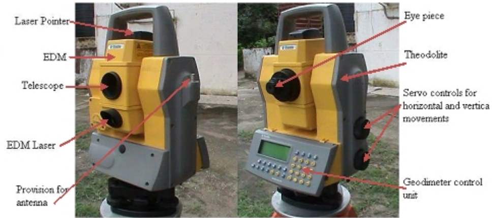
Fig.4.5 Robotic Total Station (Trimble 5601 DR200+)
