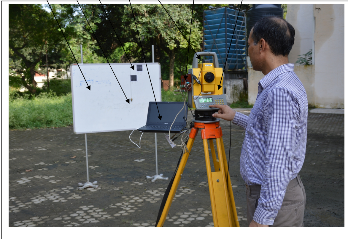
Fig.6.4 System Setup for Precise Object Targeting in PMTS
