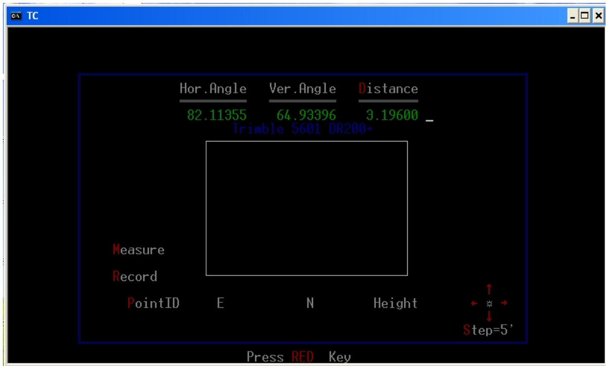
Fig. 4.8 Slope Distance measurement – Press D from CPU or A/M from GCU
