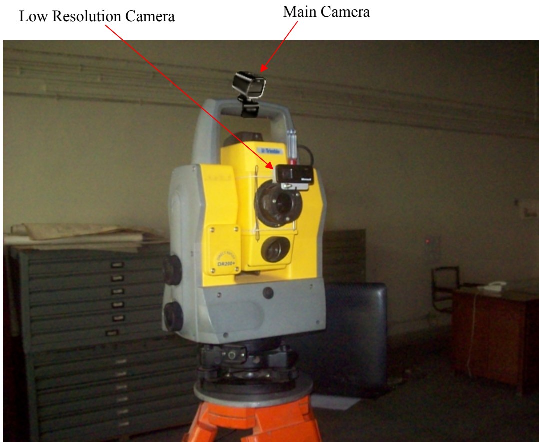
Fig.5.1 Camera mounting over handle position of Total Station
