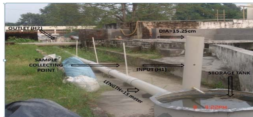
Figure 3.6 Photograph of experimental set-up for long horizontal column.
