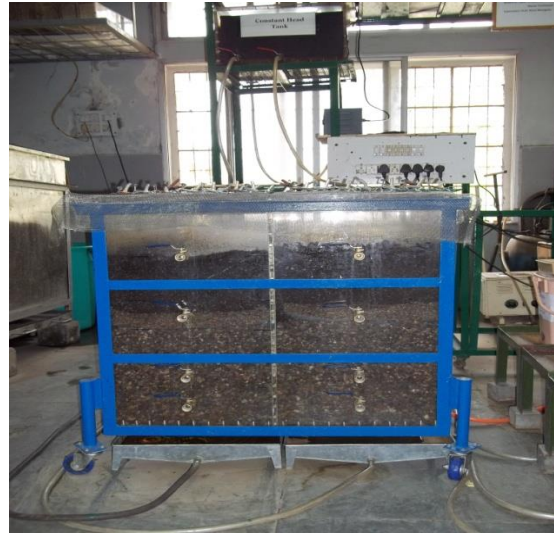
Fig. 3.7: Pilot scale vermifilter and geofilter
