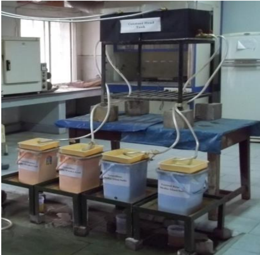
Fig. 3.4: Lab scale vermifilter having different earthworm stocking densities
