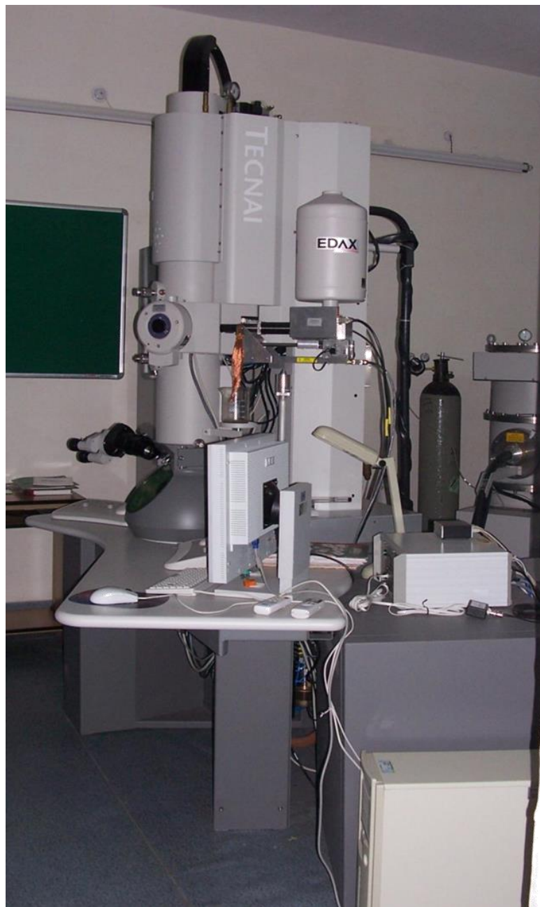
Fig. 2.16 (b) Photograph of HR-TEM (FEI Tecnai-20 G 2 ).
