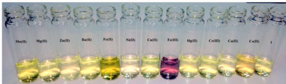
Fig. 7.9 Naked eye detection of NED2 in the presence of representative metal ions (10 eq)
