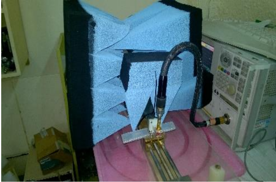
Fig. 6.4 Measurement set up with absorbing materials
