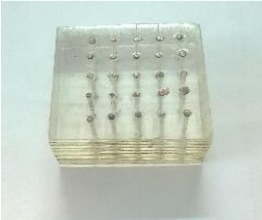
Fig. 6.2 Fabricated rodged metamaterial structure
