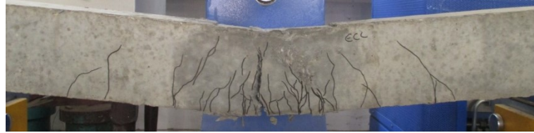
SB 1-Engineered cementitious composites (ECC)
