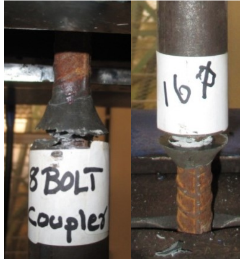
Figure 7.5: Failure pattern of 16mm dia. rebar with coupler under tension
