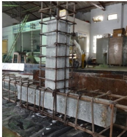
Figure 5.5: Construction technique of SIFCON core enable specimen
