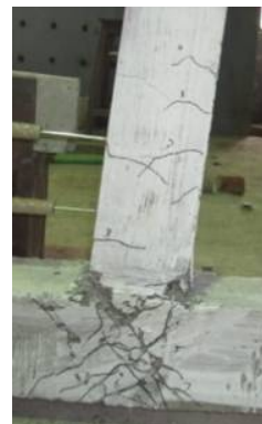
(e) EJ 5-Steel fiber reinforced
