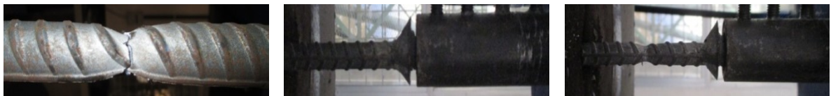
(a) Control rebar failure
