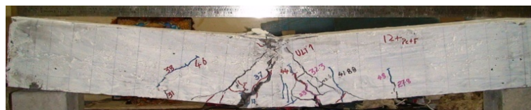
(c) B3-Geo-grid confinement with steel fibers
