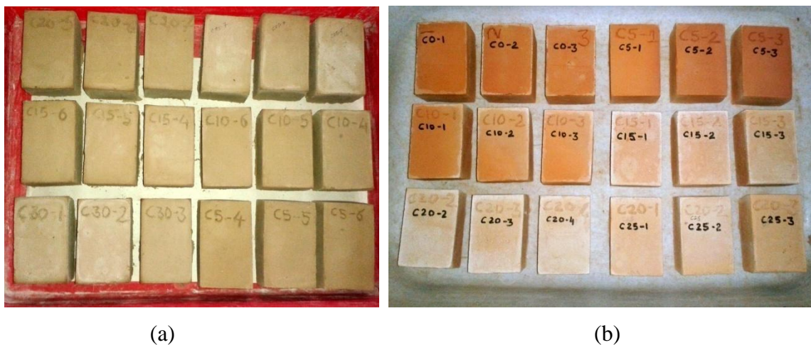
Figure-4.13 Visual appearance of brick specimens before and after firing with different dosage of deinking sludge
