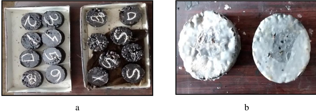
Figure 7.3 (a) Marshall Samples of BC, DBM & SMA; (b) Wax coated SMA mixes
