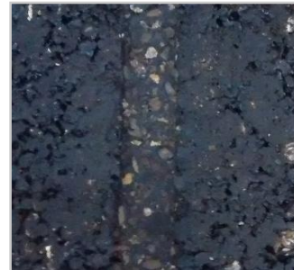
Figure 8.2 (a,b) Wheel tracking test samples, (a) before, (b) after
