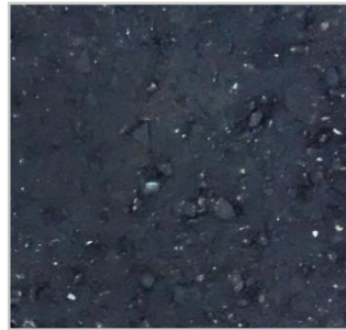
Figure 8.2 (a,b) Wheel tracking test samples, (a) before, (b) after
