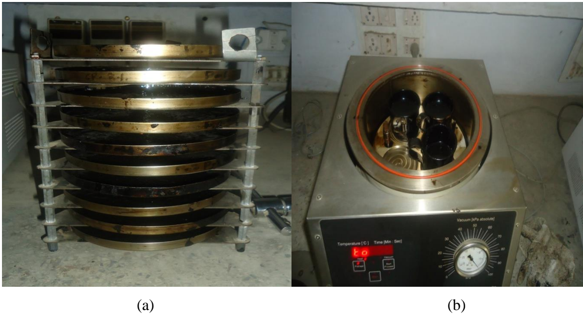
Figure 2.12 (a, b) Schematic figure of PAV pans and chamber
