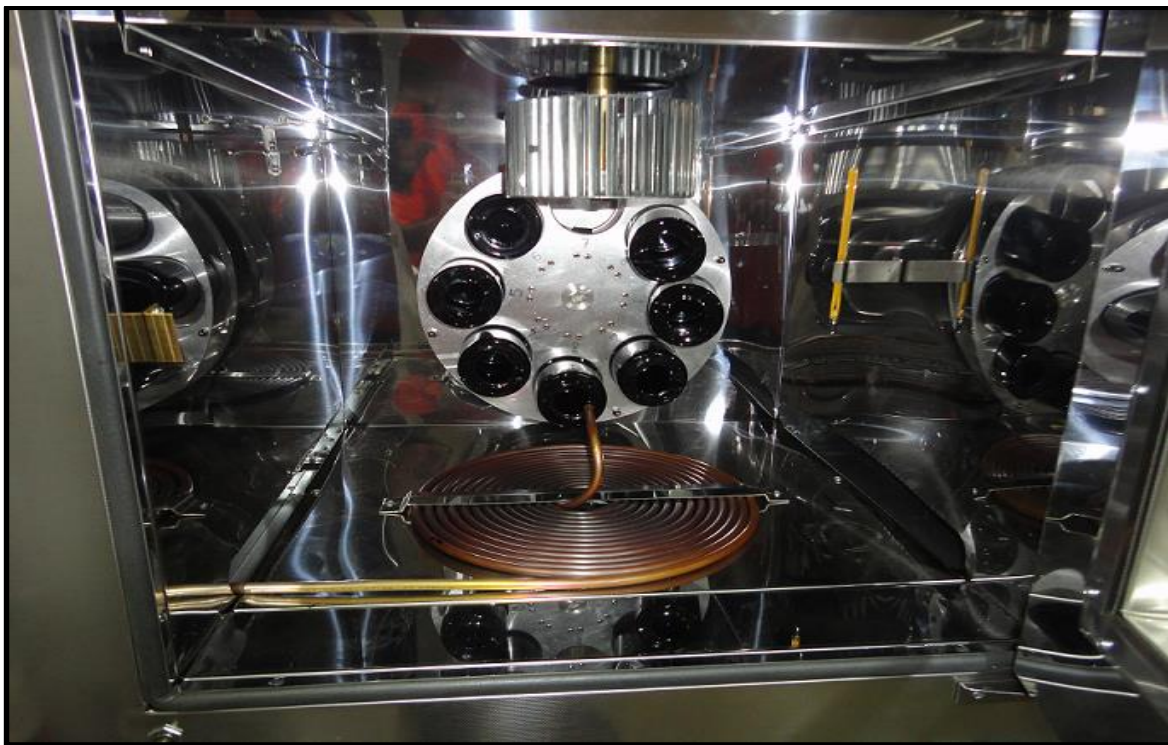
Figure 2.11 Inside chamber of the RTFOT used in the study
