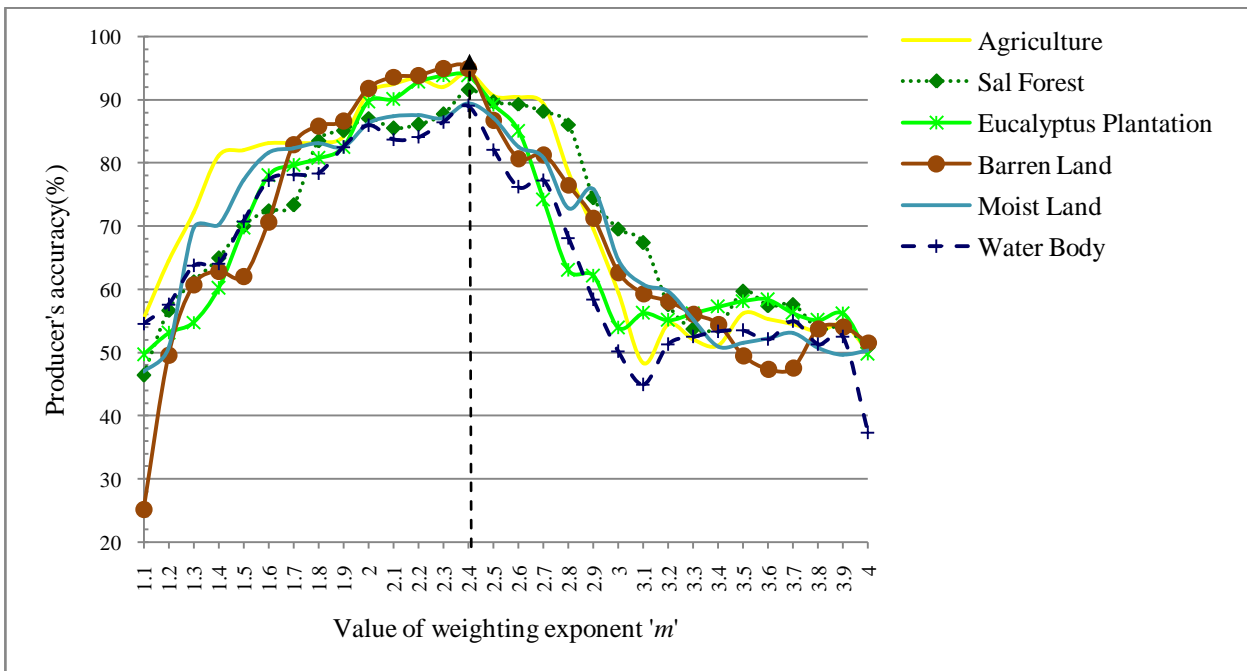
Fig. 6.10(b): Producer's accuracy of PCM classifier for AWiFS dataset using LISS-IV as reference dataset.
