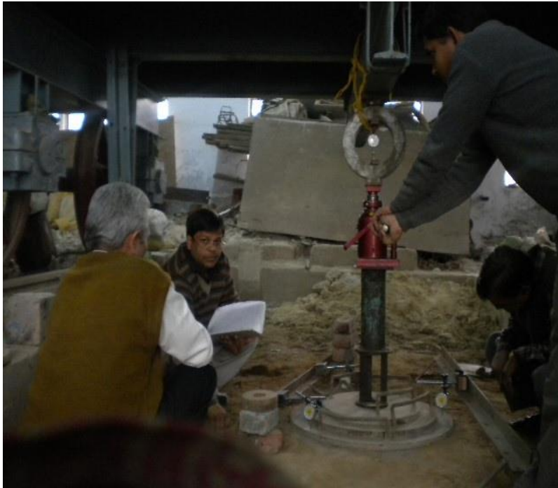
Photograph 4.9 Plate Load Test for Soil Subgrade
