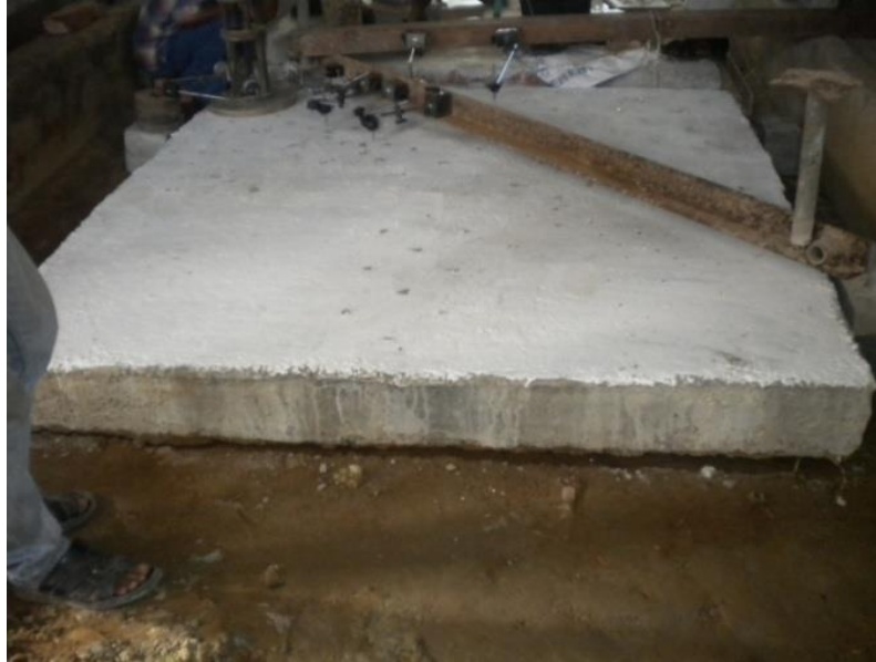
Photograph 4.21 Testing of HSHPC Pavement for Corner Position Showing Lifting from Opposite Corner
