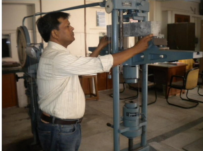
Photograph 4.4 Testing of Specimen for Flexural Strength
