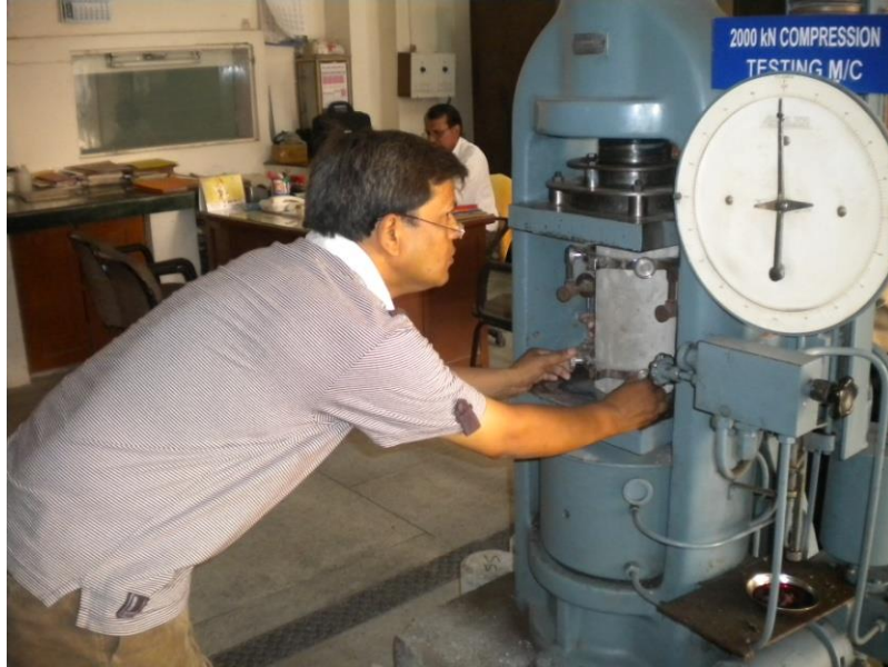
Photograph 4.6 Testing of Specimen for Modulus of Elasticity Test
