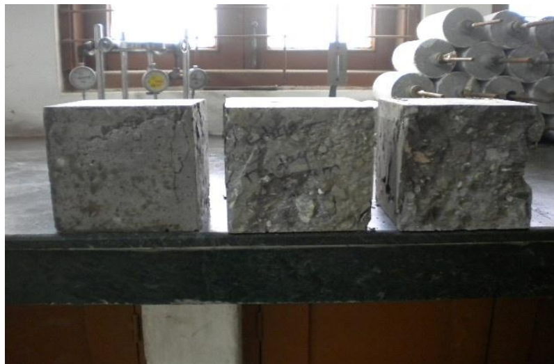
Photograph 4.3 The Broken Specimen of Compressive Strength Test
