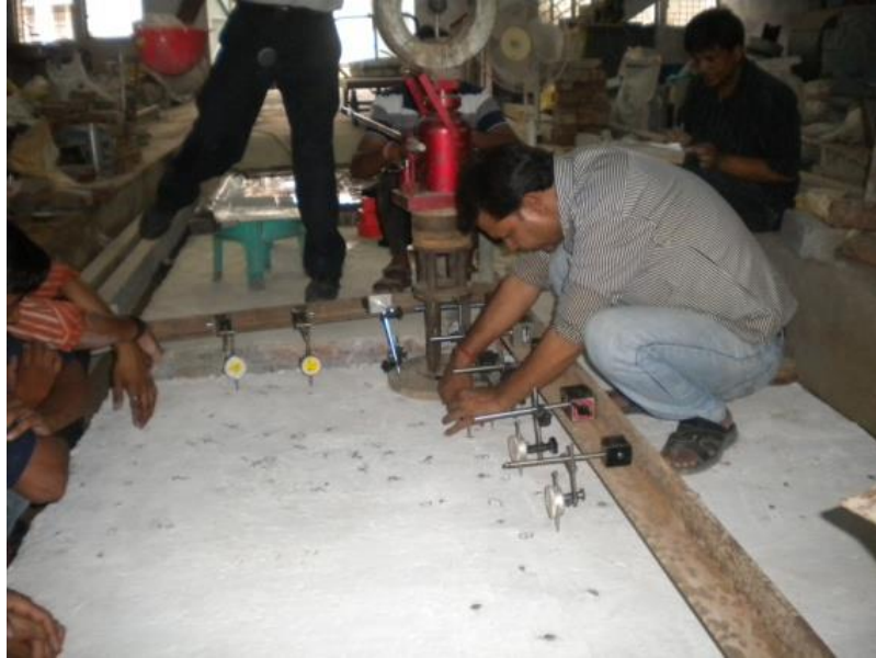
Photograph 4.19 Surface Strains Reading is being Taken during the Testing of HSHPC Pavement for Edge Position
