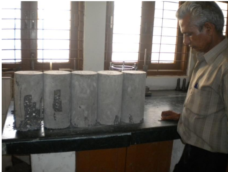
Photograph 4.7 Broken Specimen of Modulus of Elasticity Test
