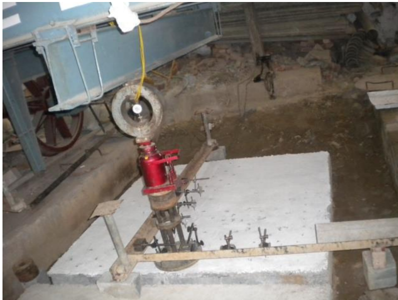
Photograph 4.18 Testing of HSHPC Pavement for Edge Position Showing Loading Arrangement and Dial Gauges
