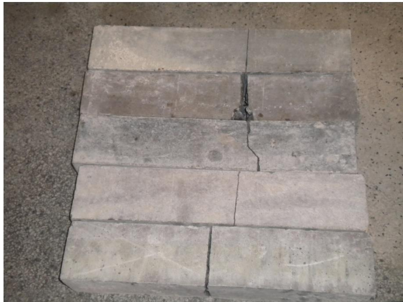
Photograph 4.5 Broken Specimen of Flexural Strength Test
