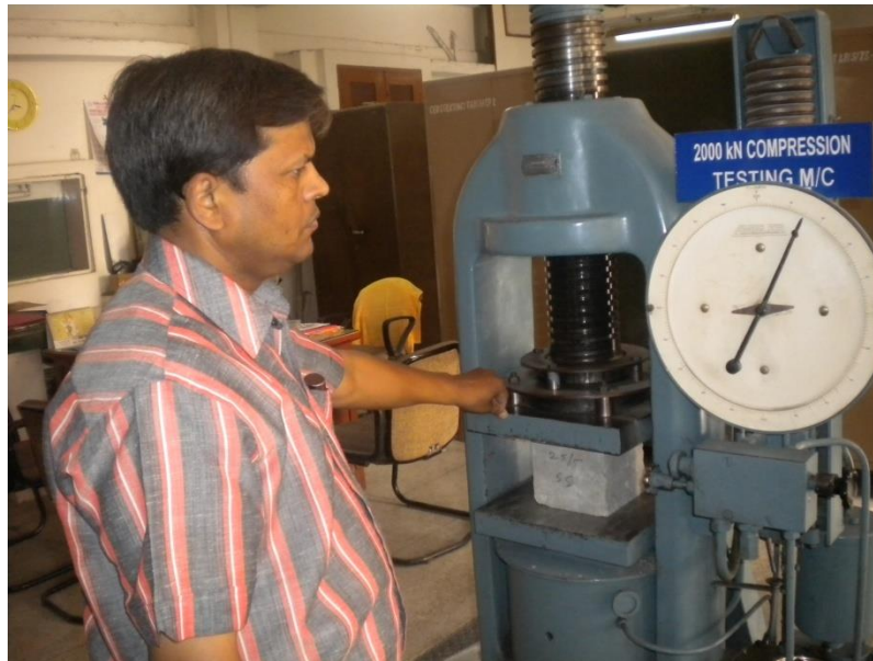
Photograph 4.2 Testing of Specimen for Compressive Strength
