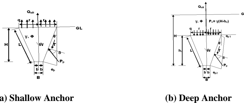
Fig. 4: Forces acting on Assumed Failure Surface
