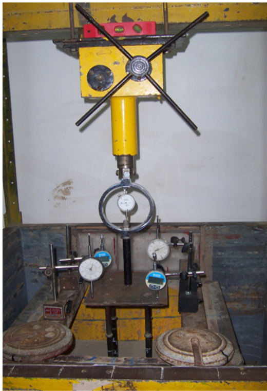
Fig. 3.6: Laboratory Test in Progress for Vertical Helical Screw Anchor
