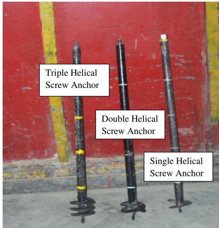
Fig. 3.1: Single, Double and Triple Helical Screw Anchor (Lab Test)
