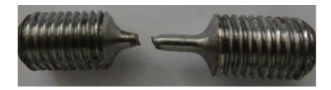
Fig. 2.21 Deformed specimen at high strain rate
