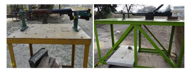
Fig. 4.1 Projectiles fired from (a) Sniper rifle and (b) Air Defence gun mounted on mounting fixture
