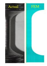
Fig. 3.15 Geometry of the tension specimen for axisymmetric finite element simulations
