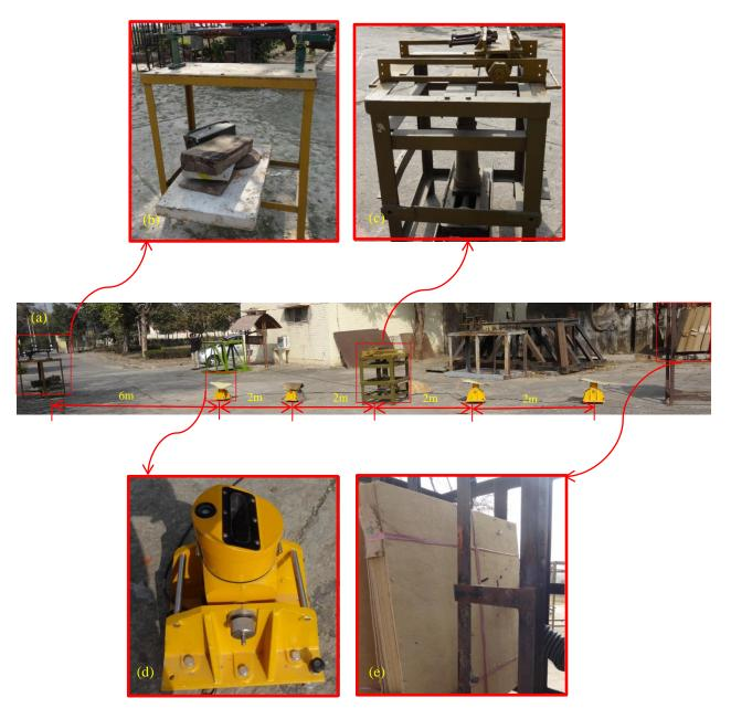
Fig. 4.2 Experimental arrangements of (a) complete test set up (b) Sniper rifle mounted on mounting platform (c) target mounting platform (d) infrared emitter device (e) projectile catcher
