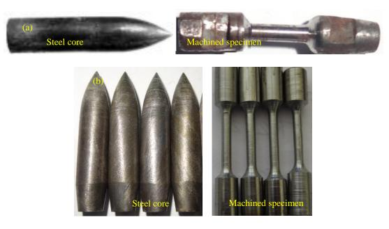
Fig. 2.47 Steel core and smooth cylindrical specimens of (a) 7.62 API and (b) 12.7 API Projectile
