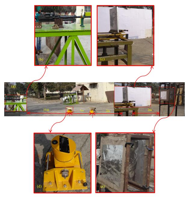
Fig. 5.2 Experimental arrangements of (a) complete test set up (b) Air Defence gun mounted on mounting platform (c) target mounted on mounting platform (d) infrared emitter device (e) aluminium foil screen
