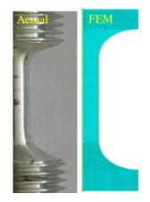
Fig. 3.21 Geometry of the tension specimen for axisymmetric finite element simulations
