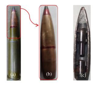
Fig. 2.44 7.62 mm API ammunition (a) projectile with shell (b) steel core with jacket and (c) cross section
