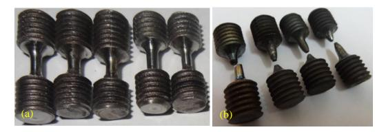
Fig. 2.54 Projectile specimens of (a) undeformed and (b) deformed surfaces at varying temperature
