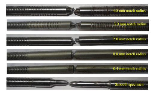
Fig. 2.20 Deformed specimens of different notch radius
