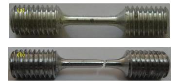
Fig 2.35 Material specimens of (a) undeformed and (b) deformed profile at high strain rate
