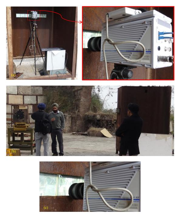
Fig. 4.3 High speed videography setup of (a) high speed camera – PHOTRON Fastcam APX-RS (b) camera shelter and target mounting platform (c) bullet proof glass
