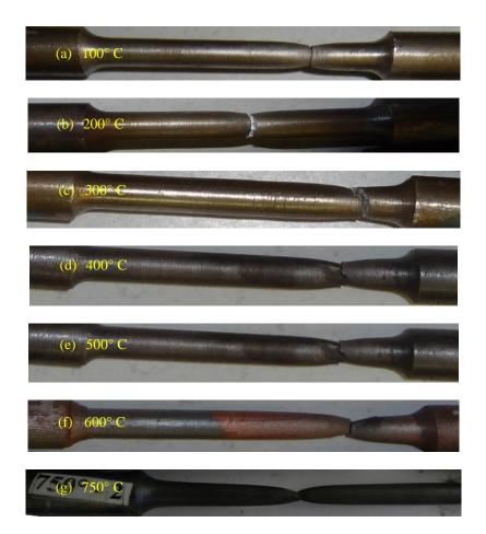
Fig. 2.13 Deformed specimens at varying temperature
