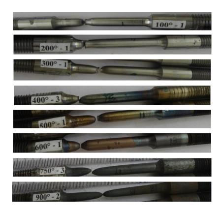
Fig. 2.24 Smooth cylindrical deformed specimens at varying temperature
