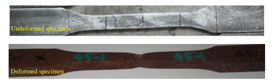
Fig. 2.1 Undeformed and deformed smooth flat specimens
