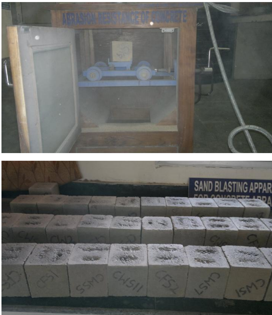
Plate 3.19 Abrasion test conducted on cubical mortar specimens
