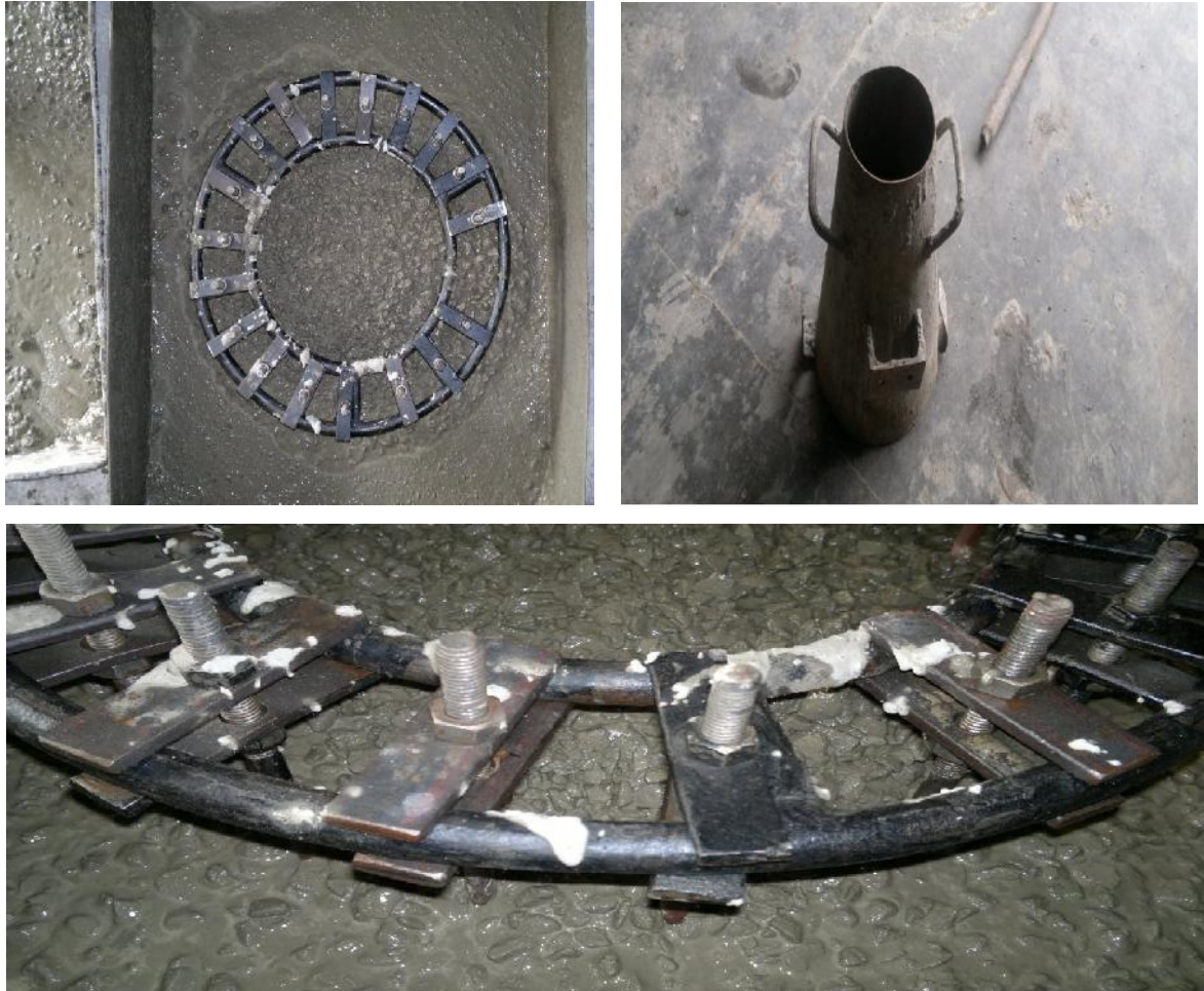
Plate 3.11 J Ring test conducted in laboratory to check the passability of SCC
