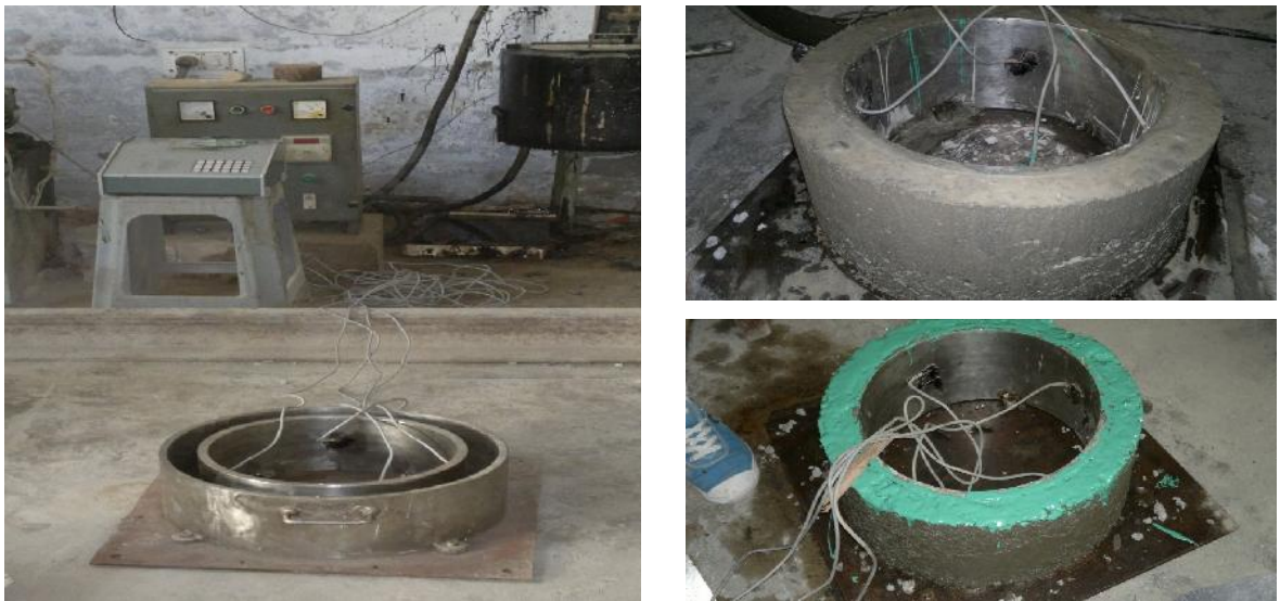
Plate 3.13 Ring shrinkage test
