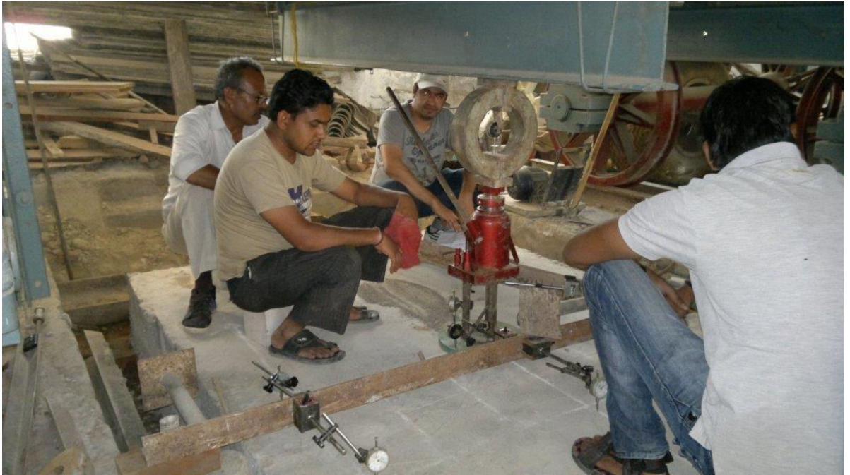
Plate 5.1 Plate load test on non-rehabilitated normal PQC
