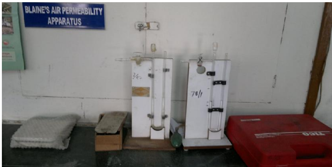
Plate 3.2 Blaine's air permeability apparatus
