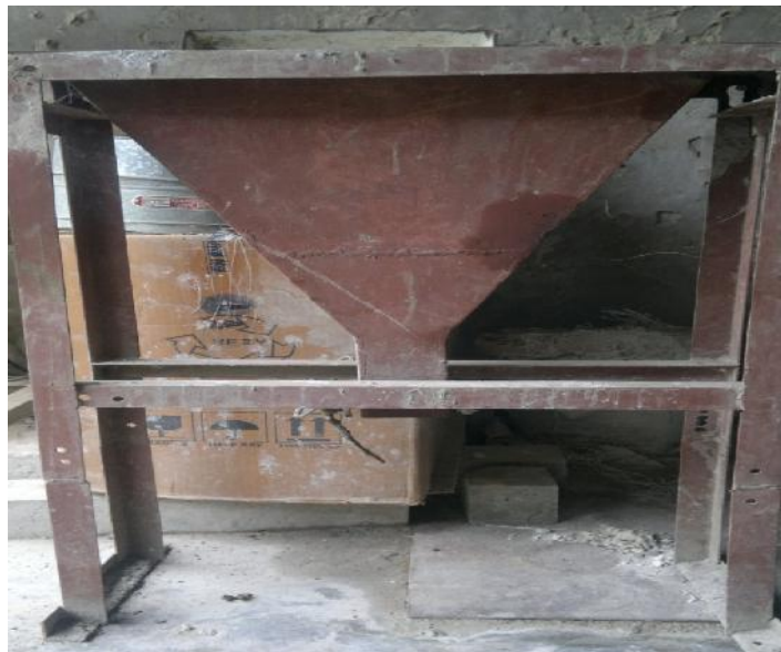
Plate 3.10 V Funnel used for checking the flow time and segregation resistance of SCC
