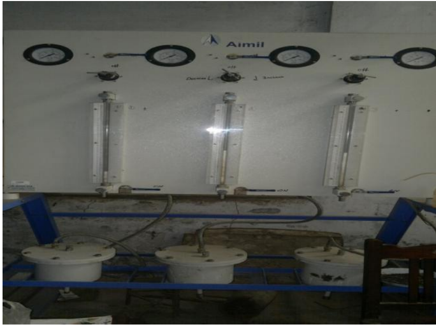
Plate 3.21 Permeability test being conducted at the laboratory
