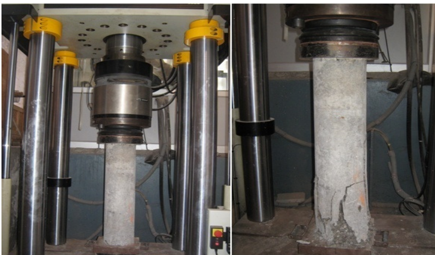
(c) Bare RCC specimen
