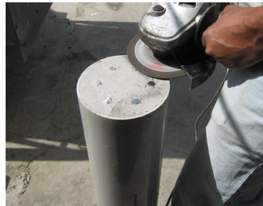
Fig. 3.16 Platens of different diameters Fig. 3.17 Levelling of specimen before testing
