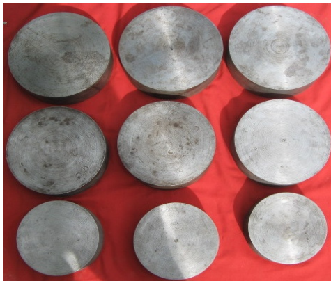
Fig. 3.16 Platens of different diameters Fig. 3.17 Levelling of specimen before testing
