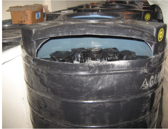
Fig. 3.14 Specimens submerged in sea water
