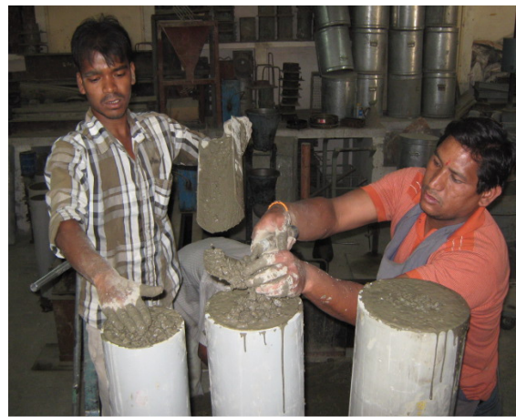
Fig. 3.11 Casting of specimens
