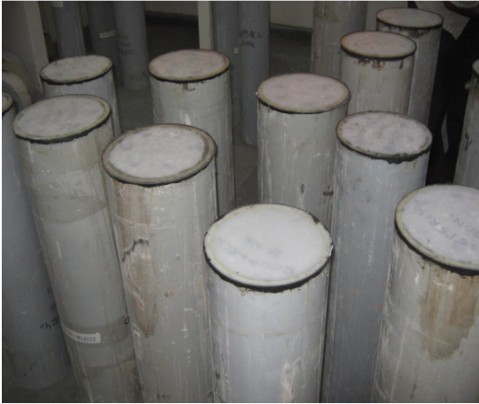
Fig. 3.13 Plastic sheet fixed on top and bottom of specimens
