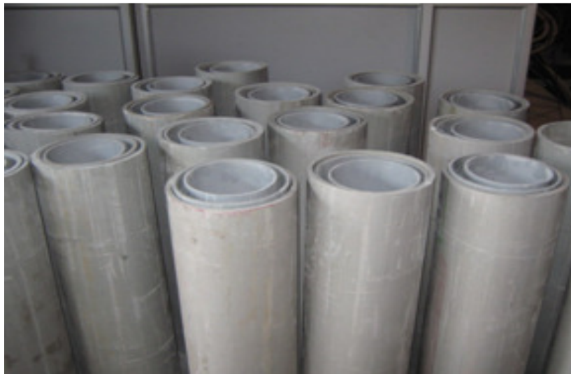
Fig. 3.2 UPVC tubes of different diameters and thicknesses after Cutting and levelling
