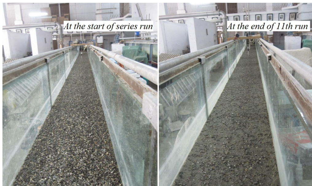
Figure 5.1: Bed surface at the start and at the end 11 th run of series 2L
