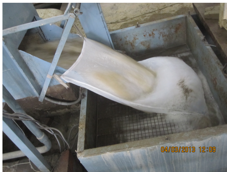
Figure 3.3: Nylon net (trap) tied at the downstream end of flume
