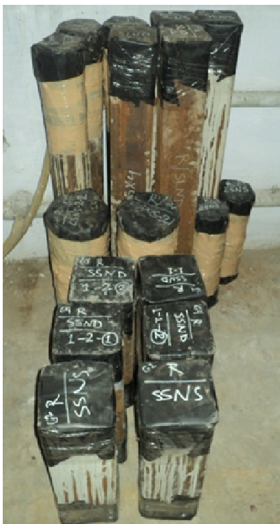
Figure 3.15 Casting of extra concrete at top to avoid effect of longitudinal shrinkage
