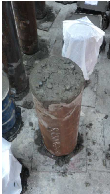
Figure 3.15 Casting of extra concrete at top to avoid effect of longitudinal shrinkage
