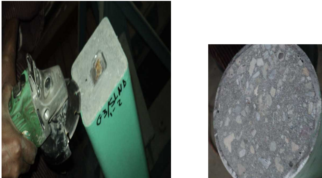
Figure 3.17 Finished CFST specimens ready for testing
