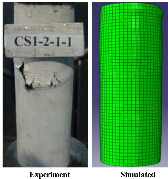
Figure 5.2(b) Comparison of Experimental and Numerical Deflected shapes of short (L3D) 165.1 mm diameter CFST columns
