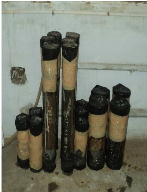
Figure 3.15 Casting of extra concrete at top to avoid effect of longitudinal shrinkage
