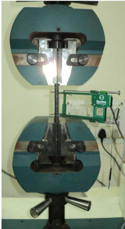
Figure 3.12 Typical test layout of rebars used for RCC-RCFST specimens
