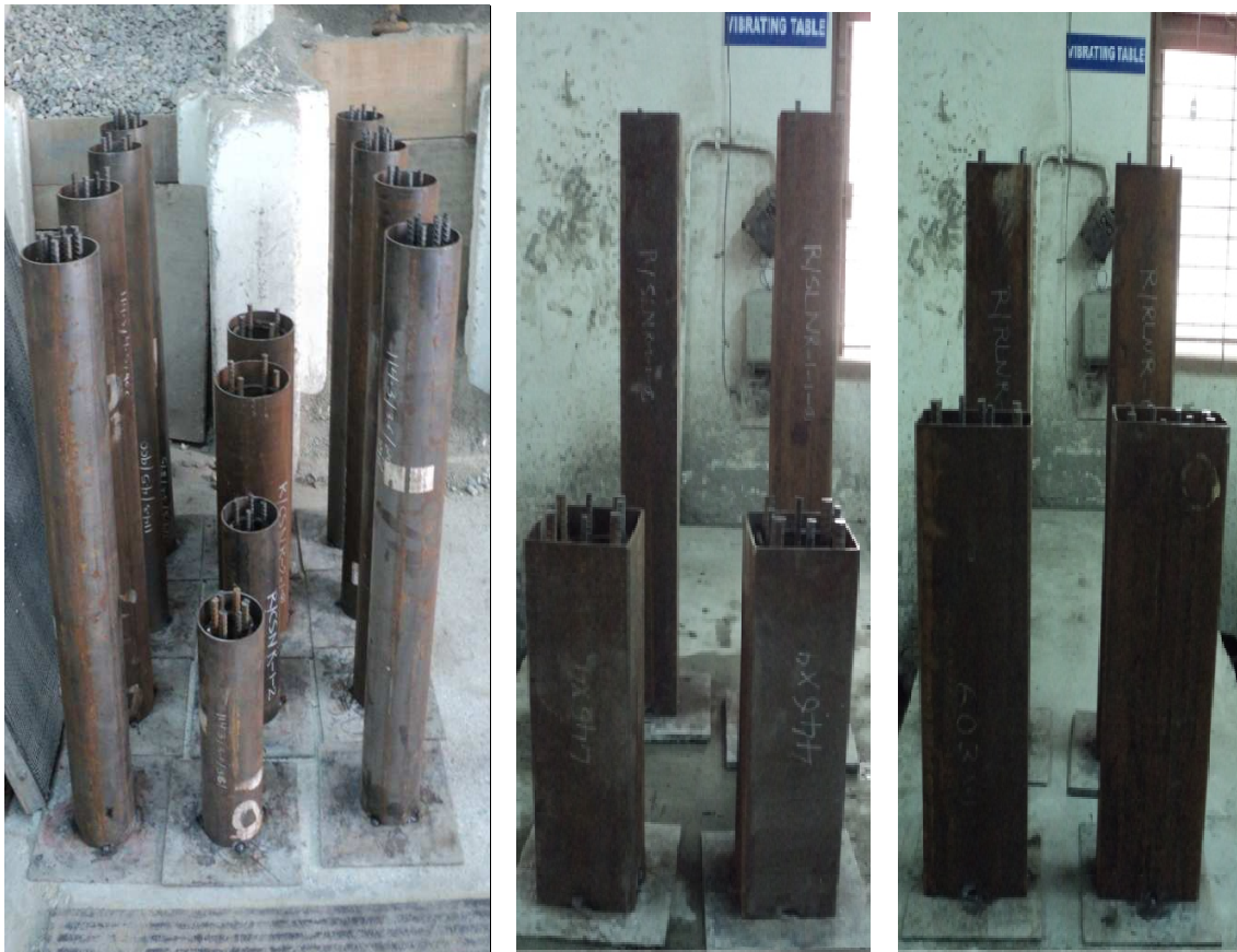
Figure 3.14 RCC-CFST specimens ready for casting
