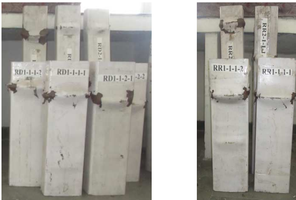
Figure 7.1(b) All tested Rectangular CFDST and RCC-CFST specimens
