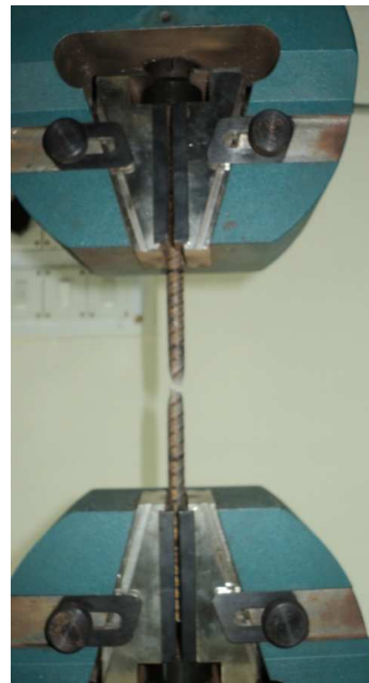
Figure 3.12 Typical test layout of rebars used for RCC-RCFST specimens
