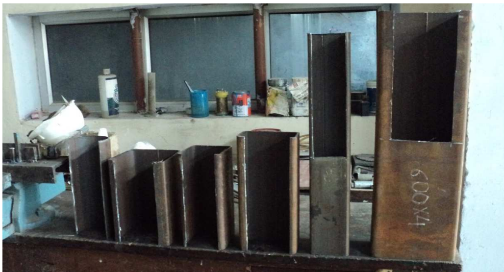
Figure 3.9 Cut locations of specimens for tensile strength test
