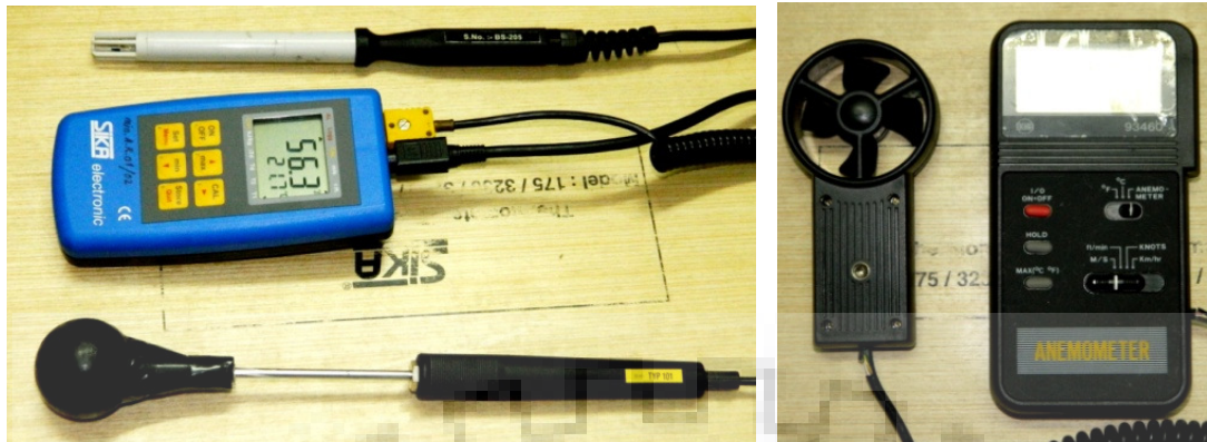
Fig 3.4a MH 3350- Thermo Hygrometer (with temperature probes) and Handheld Digital Vane Thermo Anemometer
