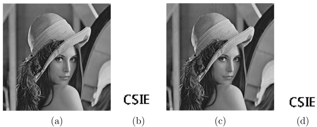
Figure 1.2: Invisible watermarking example [124]. (a): original image. (b): original watermark. (c): watermarked image. Watermark is not visible. (d): extracted watermark.
