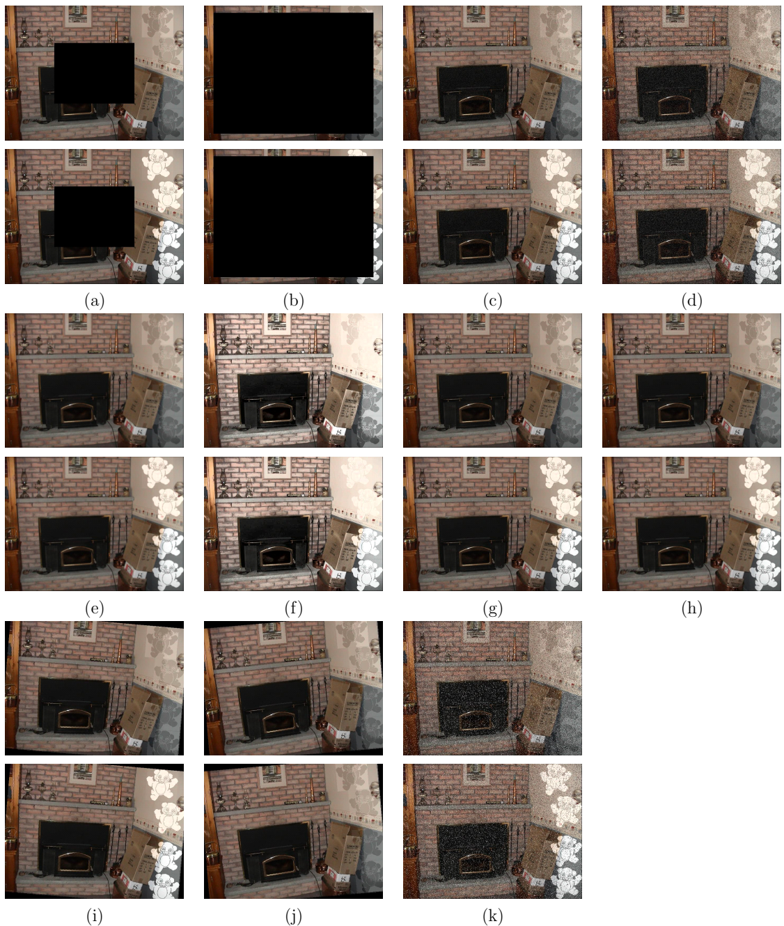
Figure 5.15: Attack analysis and comparison between proposed and existing [132] watermark embedding strategies. Results are corresponding to Fig. 5.12. Top row in each sub-figures is corresponding to proposed watermark embedding strategy and the bottom rows are corresponding to existing watermark embedding strategy of [132]. (a): Cropping 20% (b): cropping 80 % (c) Gaussian noise, variance=0.001 (d) Gaussian noise, variance=0.001 (e) Gaussian filter, variance 1, filter size 11X11 (f) histogram equalization (g) JPEG compression, quality factor=70 (h) scaling down and up, scale factor=0.5 (i) rotation 5 degree (j) rotation -5 degree (k) salt and pepper noise, density=0.1
