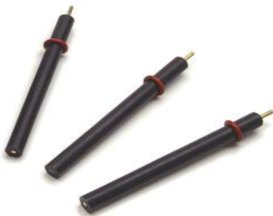
Fig. 1.1 Glassy carbon electrode used for electrochemical studies.
