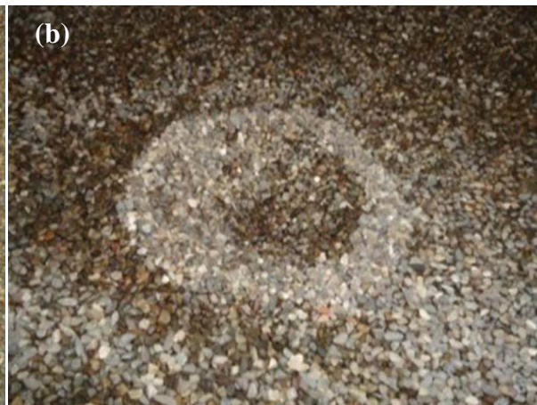
Run no. G2, d_o = 12.5 mm, u_o = 7.19 m/s, h_j = 0.15 m, d_{50} = 2.7 mm
