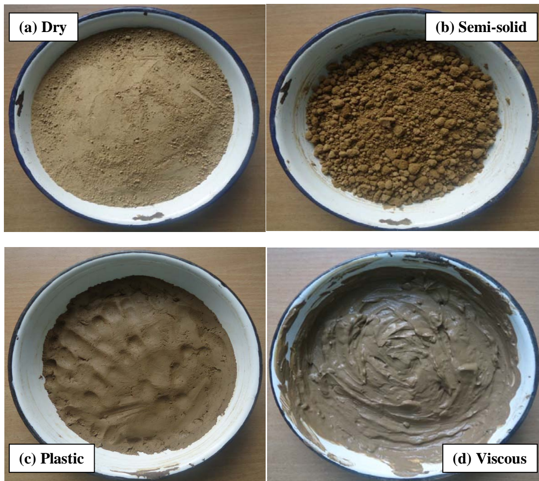
Fig. 3.4 Picture showing (a) dry, (b) semi-solid, (c) plastic and (d) viscous states of cohesive sediment
