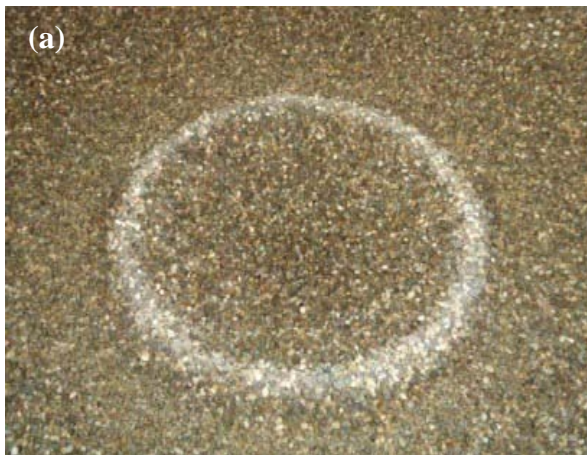
Run no. G1, d_o = 12.5 mm, u_o = 7.19 m/s, h_j = 0.30 m, d_{50} = 2.7 mm
