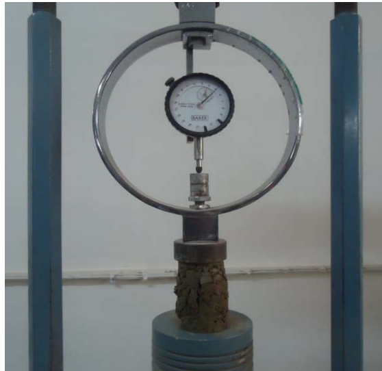
Fig. 3.12 Measurement of unconfined compressive strength of the sediment sample
