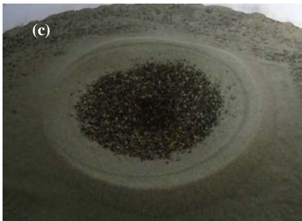
Run no. SG5, d_o = 8 mm, u_o = 9.84 m/s, h_j = 0.30 m, d_a = 1.47 mm
