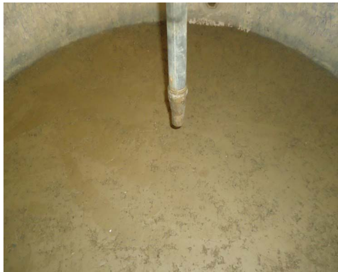
Fig. 3.11 Prepared cohesive sediment bed before start of the experiment
