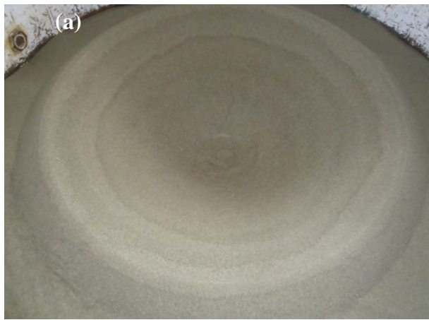
Run no. S1, d_o = 12.5 mm, u_o = 7.19 m/s, h_j = 0.30 m, d_{50} = 0.24 mm
