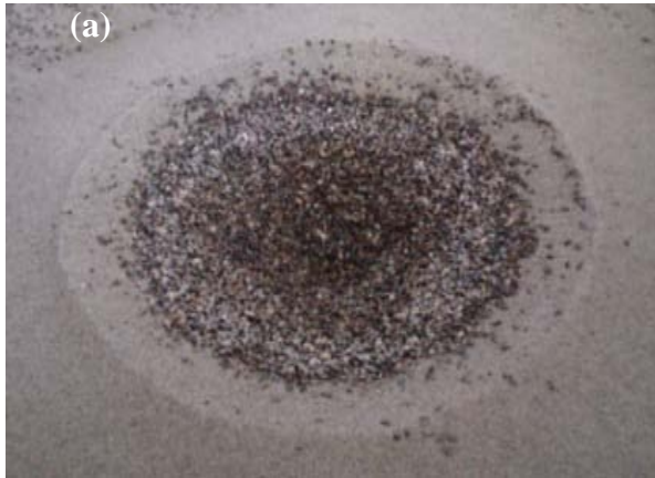
Run no. SG1, d_o = 12.5 mm, u_o = 7.19 m/s, h_j = 0.30 m, d_a = 1.47 mm
