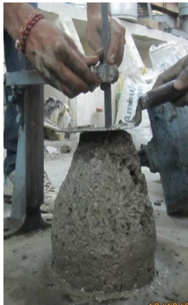
Fig. 2. 3: Slump test of green concrete
