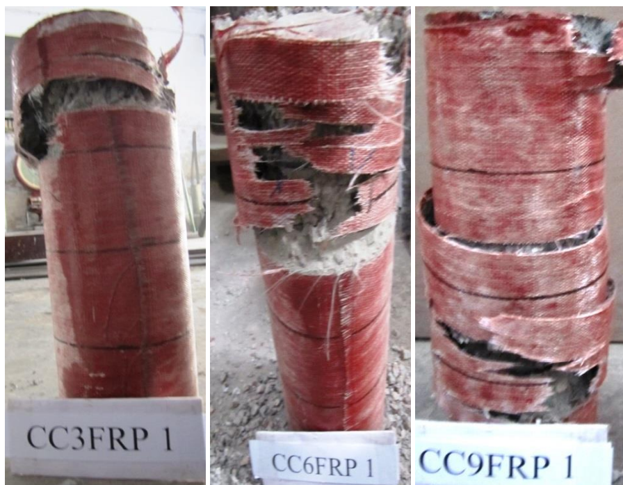
Fig. 2. 18: Failure pattern of heat damaged reinforced concrete columns strengthened by GFRP jacket
