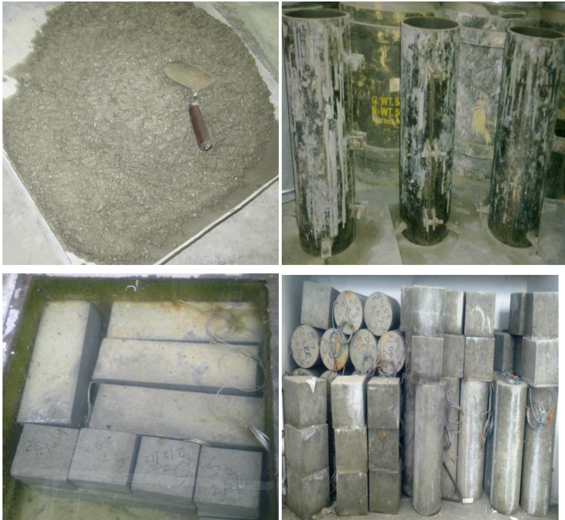
Fig. 2. 4: Stages of casting, de-moulding, curing and laboratory condition of specimens
