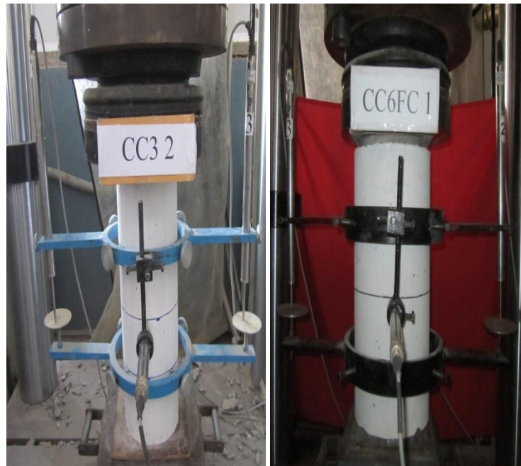
Fig. 2.14: Test set up and arrangement of instruments on control specimens and on strengthen specimens
