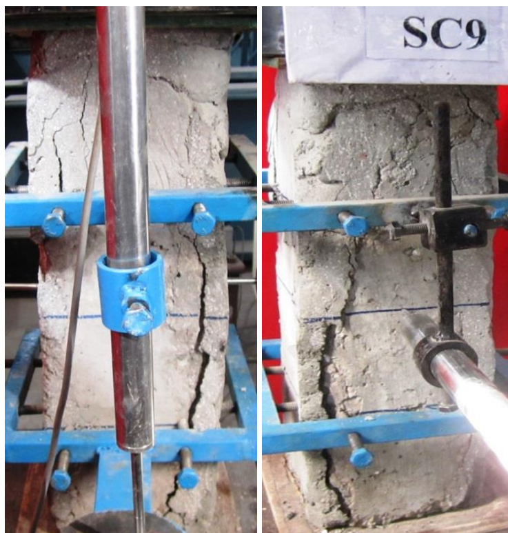
Fig. 3. 17: Typical failure pattern of micro concrete repaired specimens
