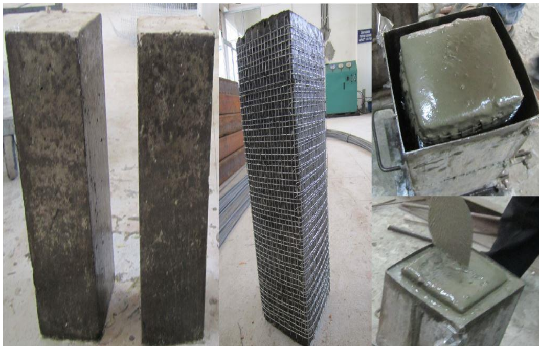
Fig. 3.8: Strengthening process of FC jacketing
