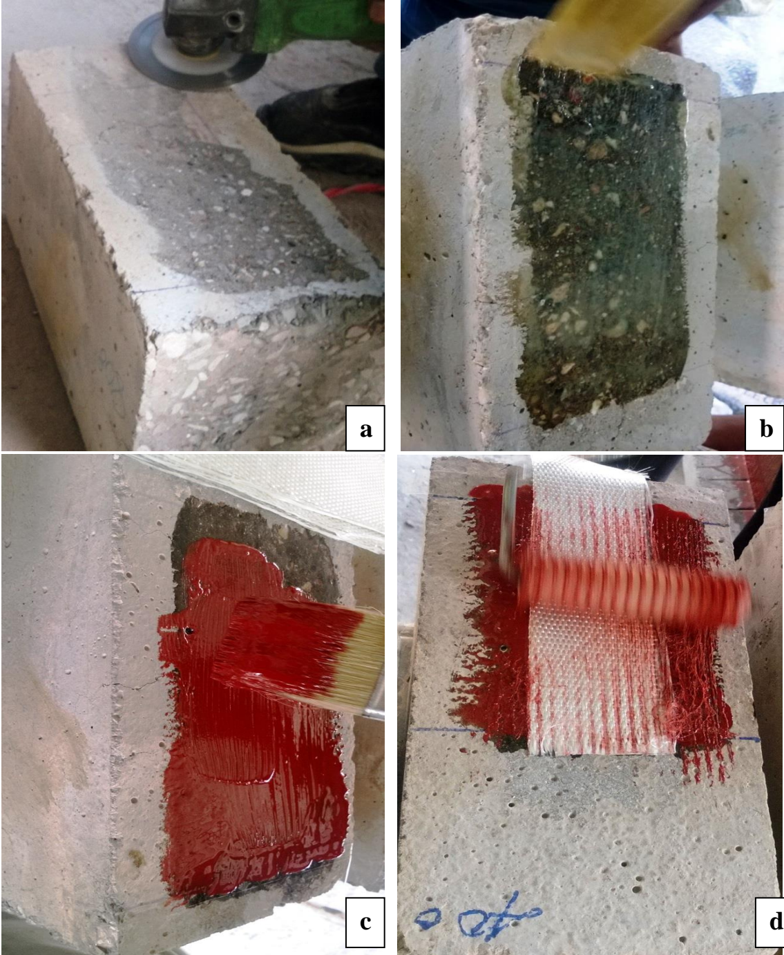
Fig. 5. 5(a-d): Process of bonding GFRP sheet to SST Specimens
