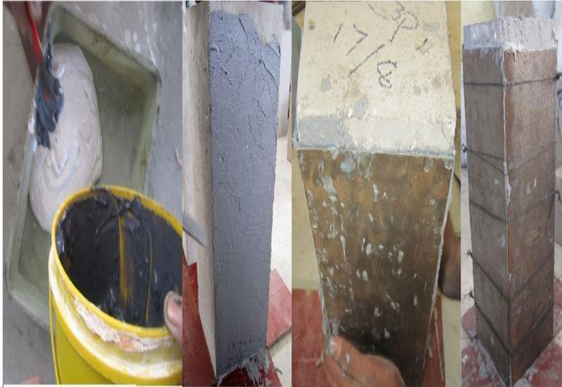
Fig. 3.10: Strengthening process of SP Jacketing
