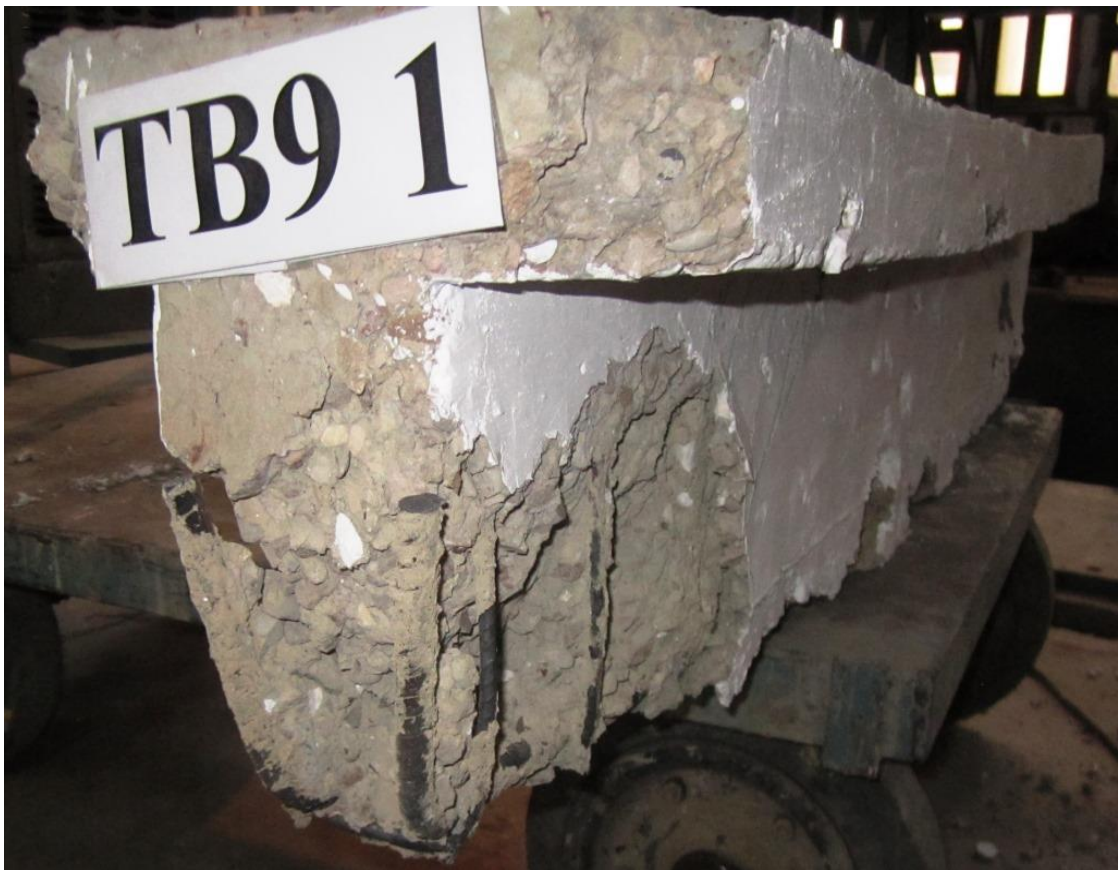
Fig. 4.22: Failure pattern of 900° C heat damaged beams
