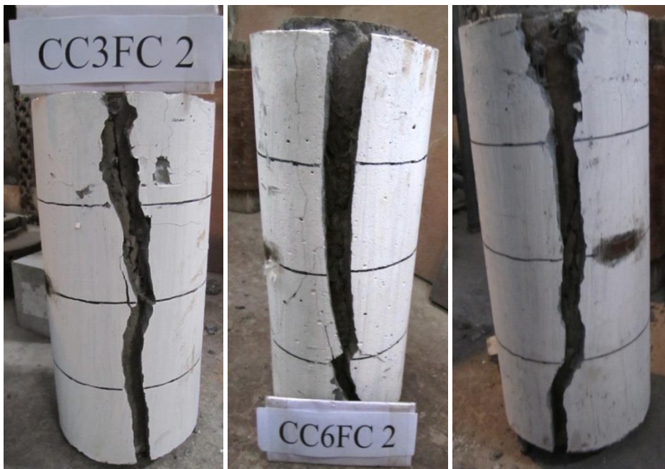
Fig. 2.16: Failure pattern of heat damaged reinforced concrete columns strengthened by HSFRC jacket
