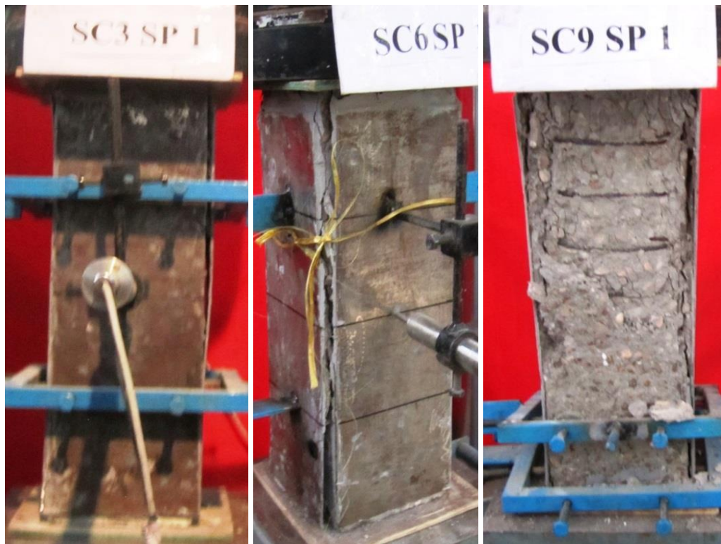
Fig. 3. 16: Typical failure pattern of SP strengthened square column
