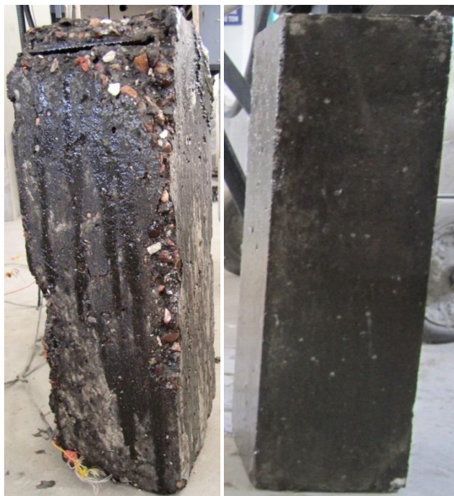
Fig. 3.6: View of a typical specimen before repair and after application of micro concrete
