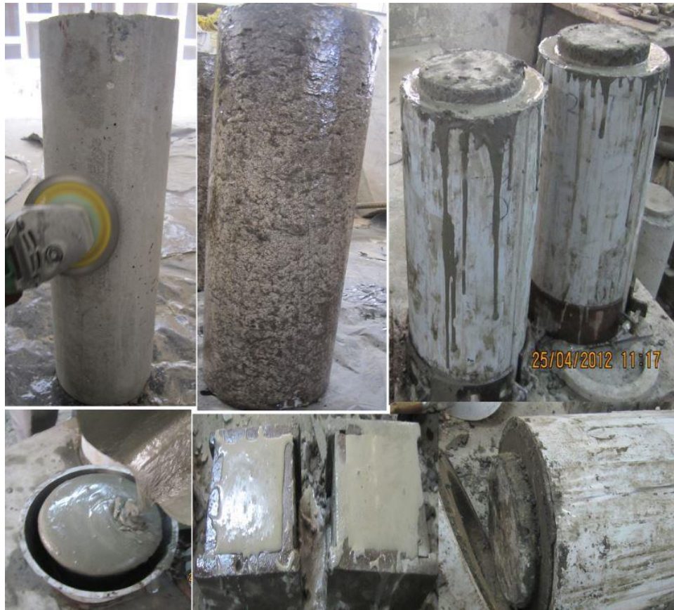
Fig. 2.11: Stages of HSFRC jacketing
