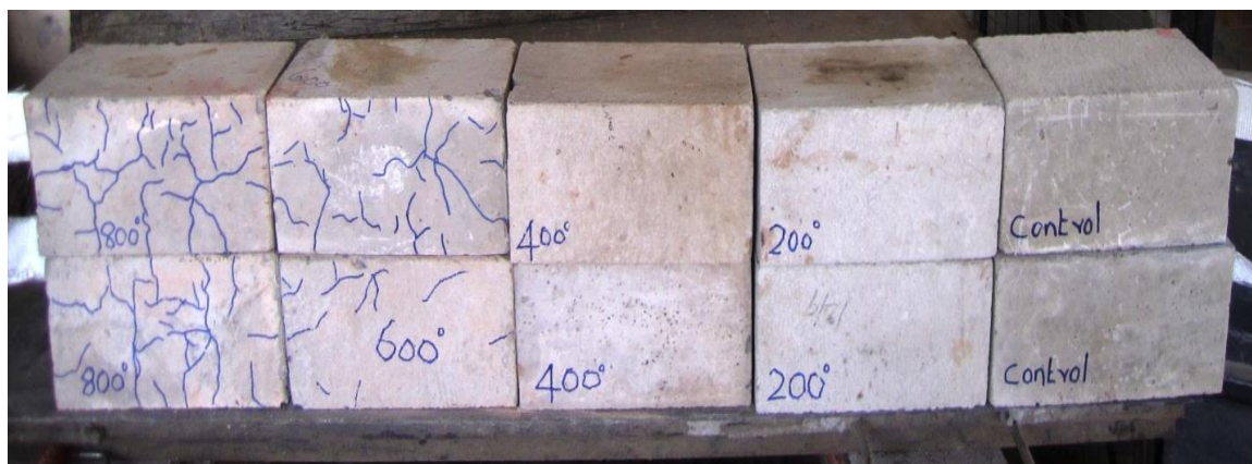
Fig. 5.3: Crack pattern in heated specimens
