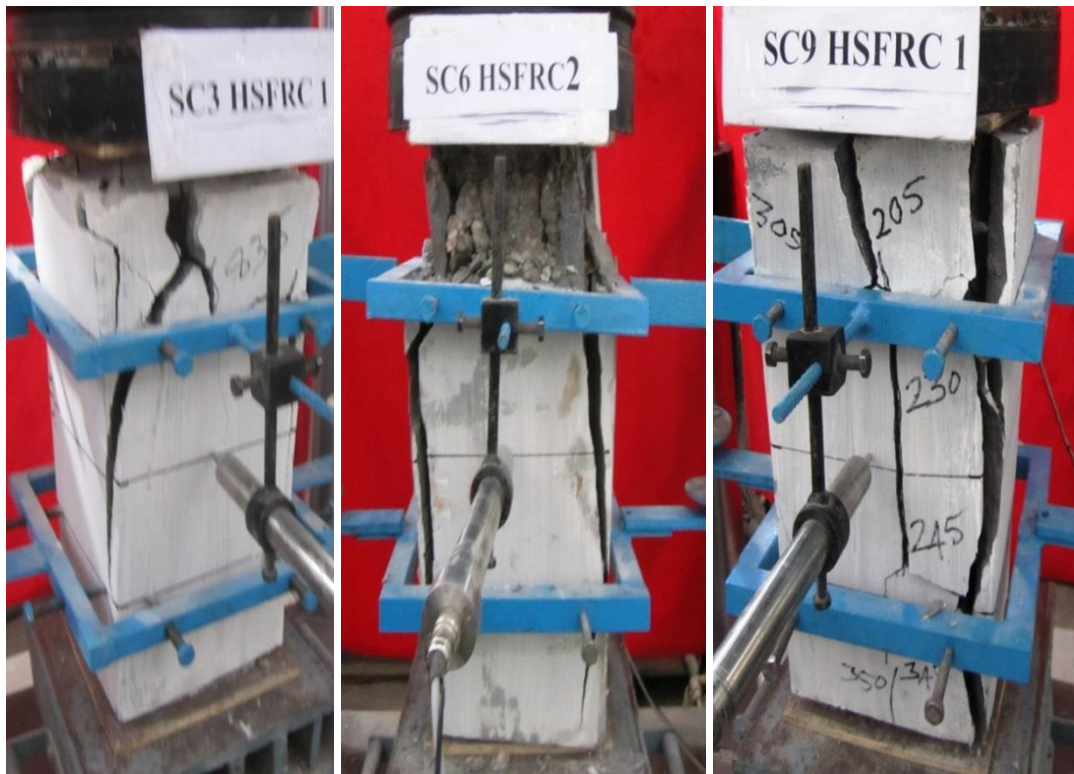
Fig. 3.13: Typical failure pattern of HSFRC strengthened square column specimens
