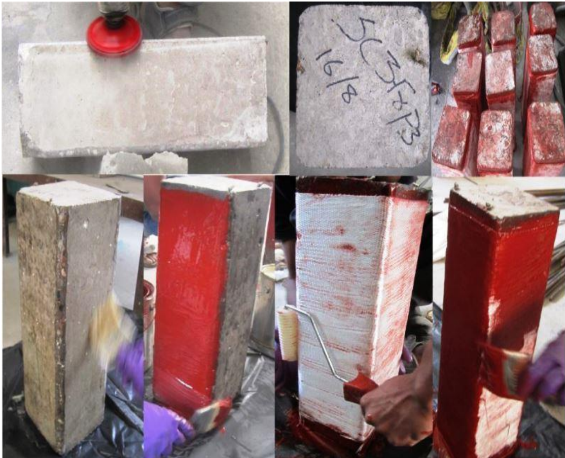
Fig. 3. 9: Strengthening process of GFRP jacketing
