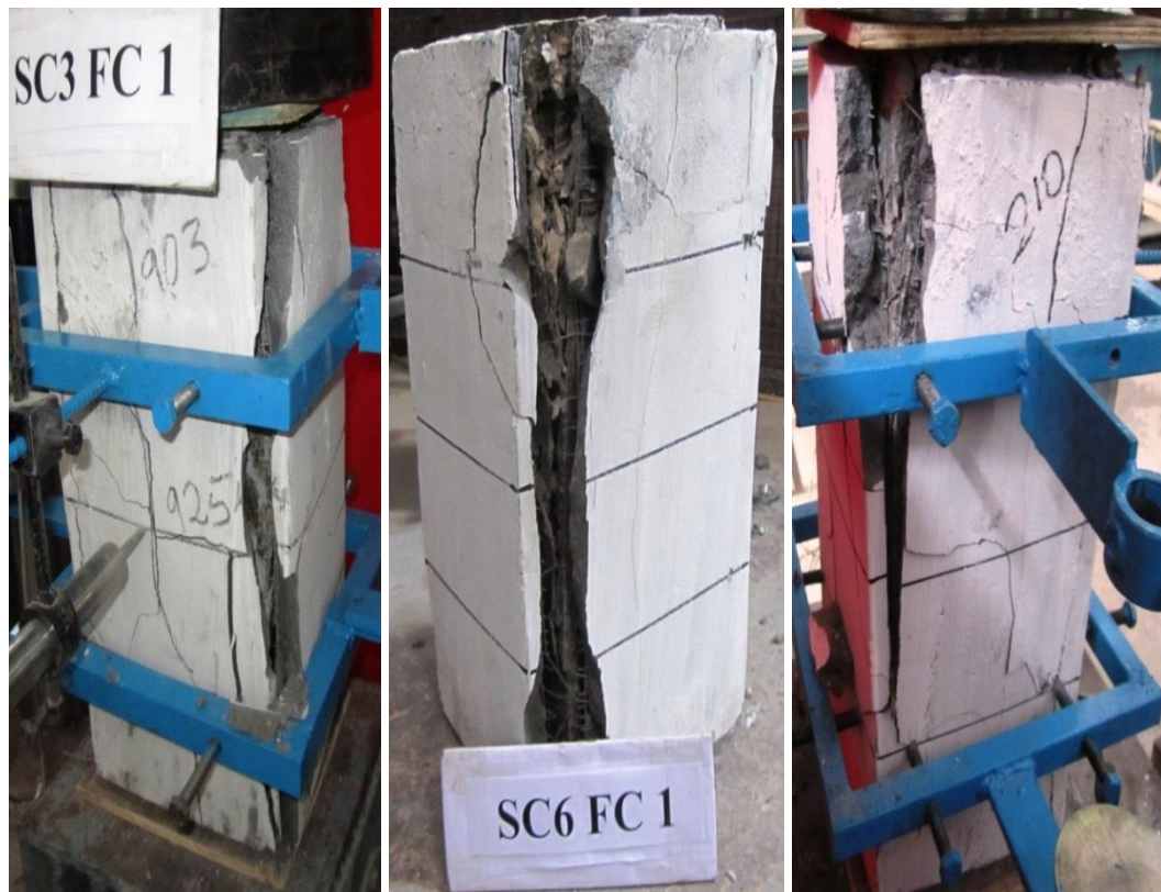
Fig. 3.14: Typical failure pattern of FC strengthened square column
