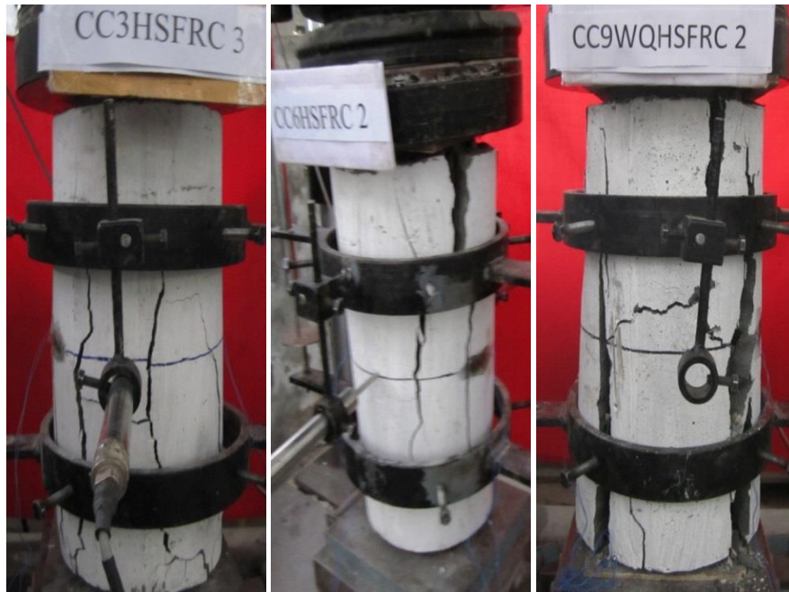
Fig. 2.16: Failure pattern of heat damaged reinforced concrete columns strengthened by HSFRC jacket
