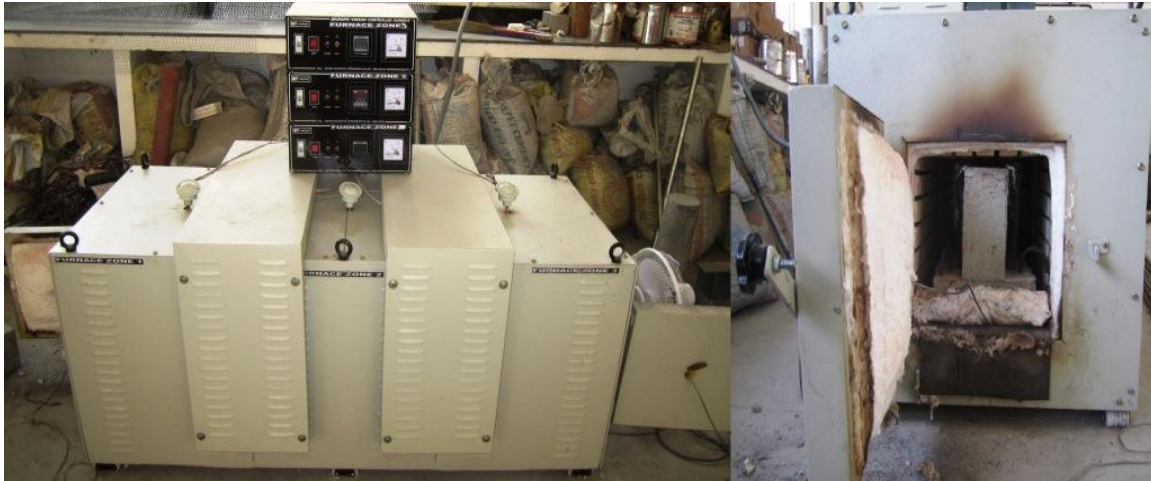
Fig. 4.4: A view of furnace and beam specimen
