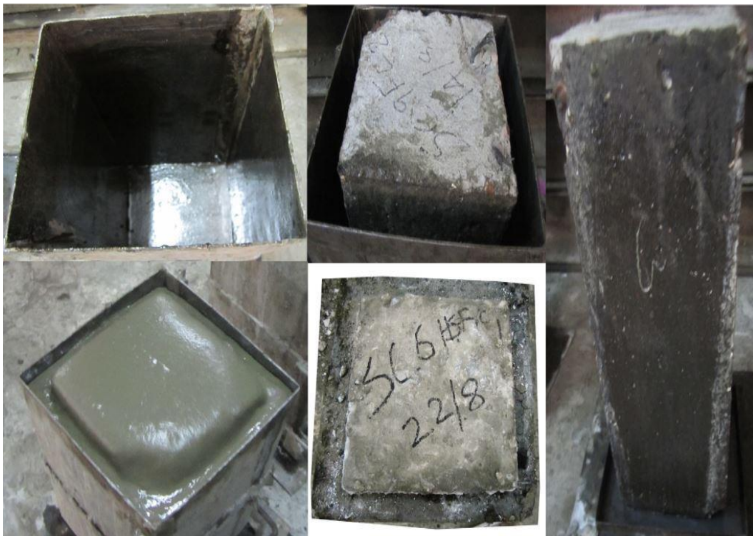
Fig. 3.7: Strengthening process of HSFRC jacketing
