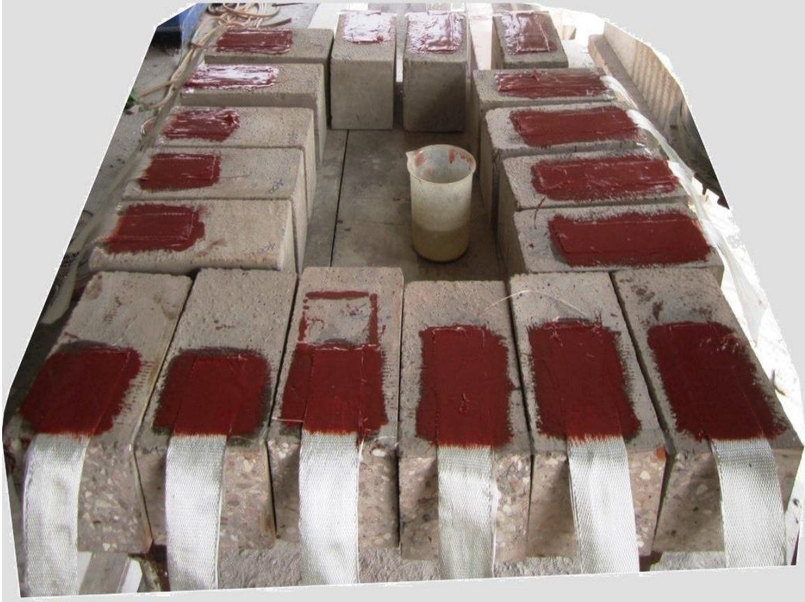
Fig. 5. 6: Specimens after GFRP bonding
