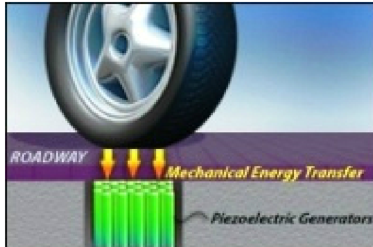
Figure 1.1: Electricity generated from force
