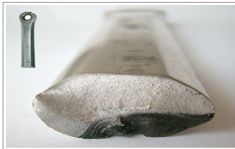
Figure 1.15: Brittle fracture in Aluminum crank arm
