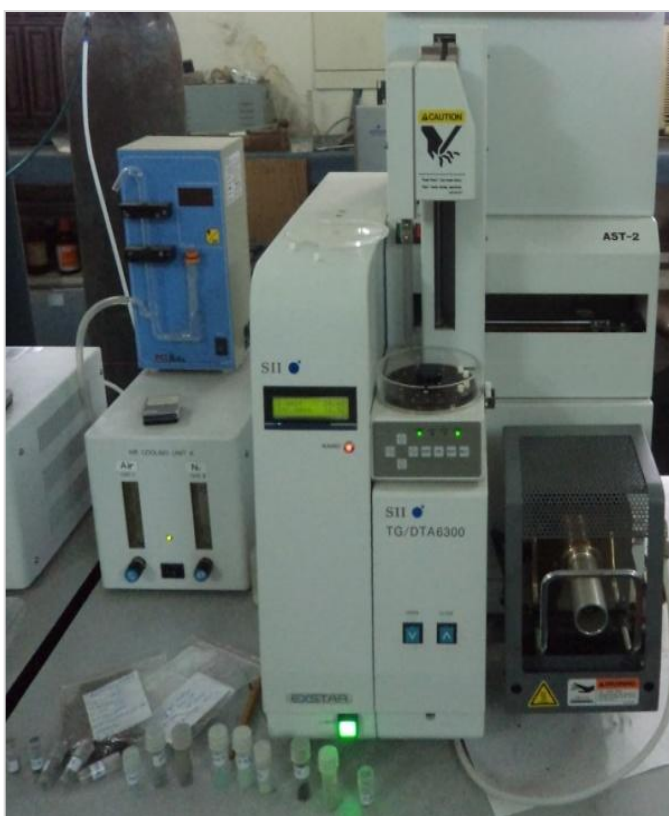
Fig. 4.12: A photograph of thermo gravimetric analysis (TGA) system used in the present study.
