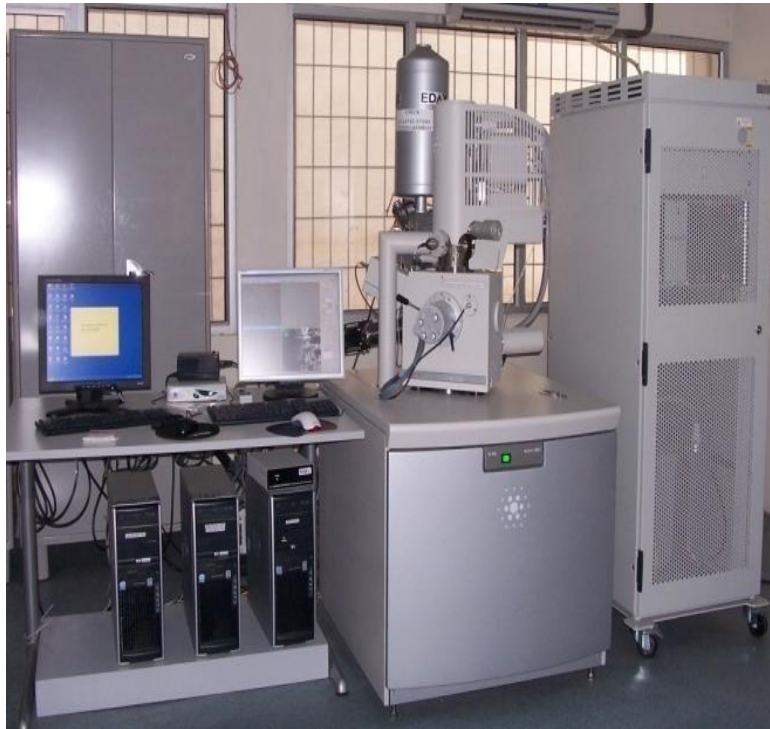
Fig. 4.1: Field emission scanning electron microscope (FESEM) equipped with EDS analyzer.
