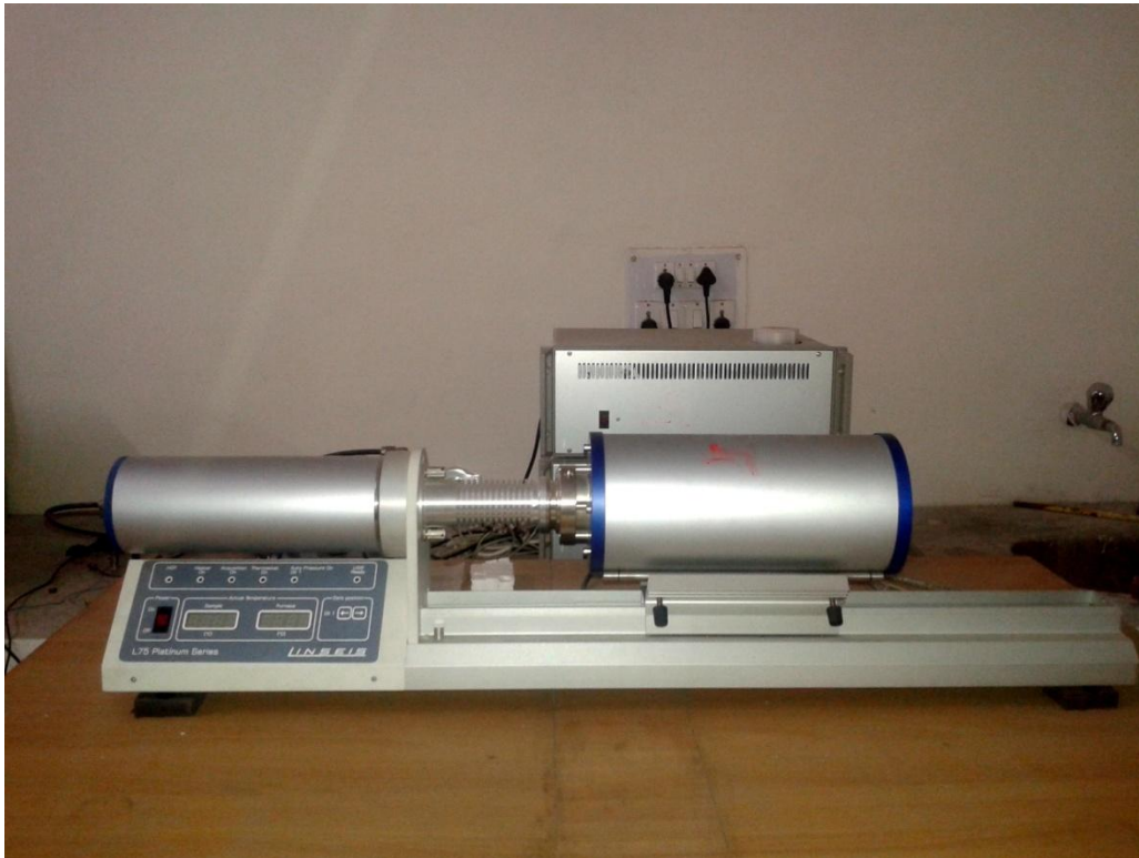
Fig. 4.13: LINSEIS L 75 Dilatometer used for coefficient of thermal expansion.
