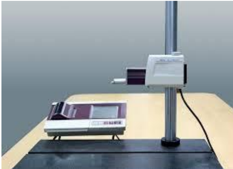
Fig. 4.11: Surface profiler (Mitutoyo SJ-400, Japan) used for surface roughness of the specimens.
